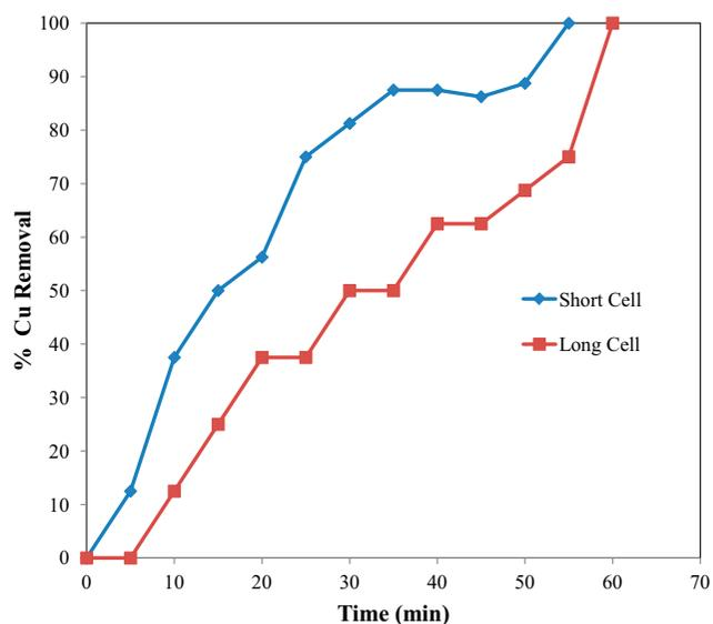
Fig. 9. Effect of size of the EC cell.  $C_0 = 10$  g/L, stirring speed = 60 rpm, 8Fe electrodes, current = 250 mA, voltage = 12 V.
