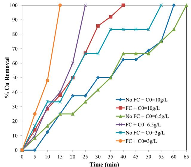
Fig. 8. Effect of using FC, 8Fe electrodes, stirring speed = 60 rpm, short cell, current = 250 mA, voltage = 12 V.
