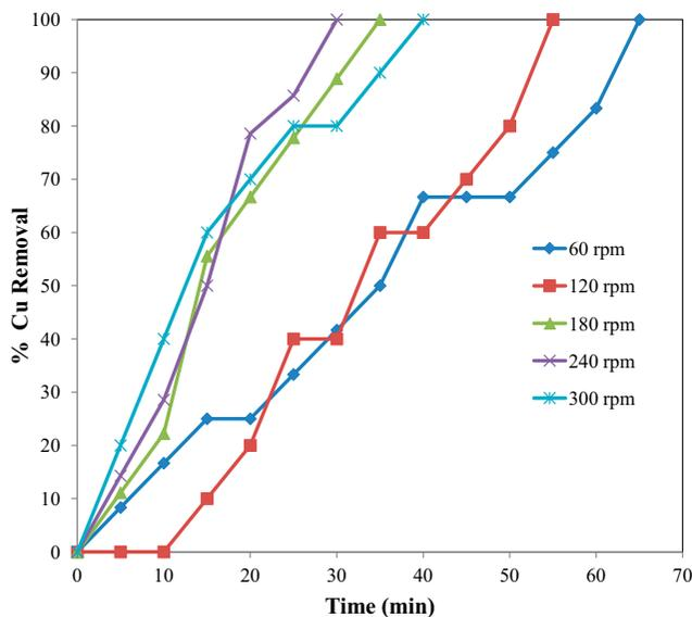
Fig. 3. Effect of speed of stirring,  $C_0 = 6.5$  g/L, 8 Fe electrodes, short cell, current = 250 mA, voltage = 12 V.
