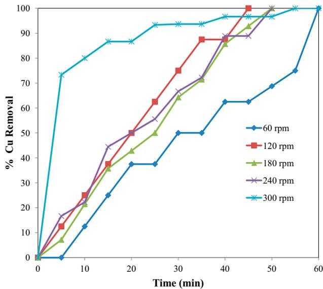
Fig. 2. Effect of speed of stirring,  $C_0 = 10$  g/L, 8 Fe electrodes, short cell, current = 250 mA, voltage = 12 V.
