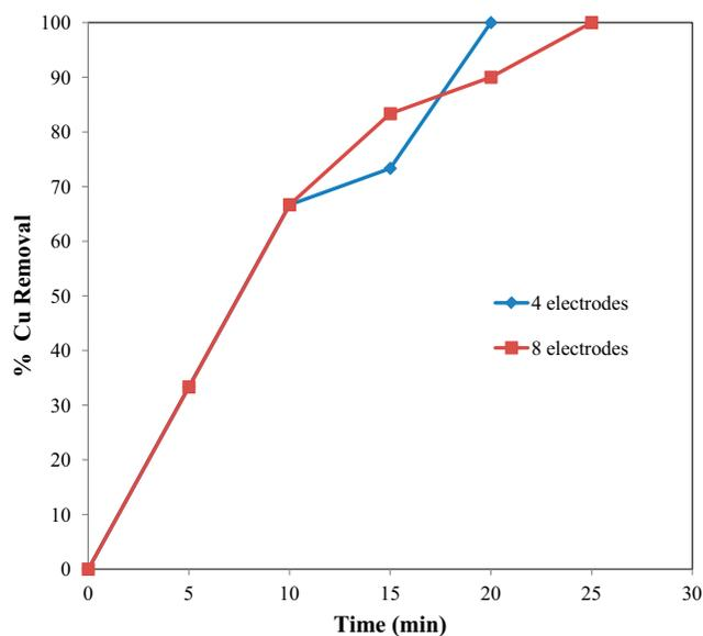
Fig. 5. Effect of number of Fe electrodes,  $C_0 = 3$  g/L, stirring speed = 300 rpm, short cell, current = 250 mA, voltage = 12 V.
