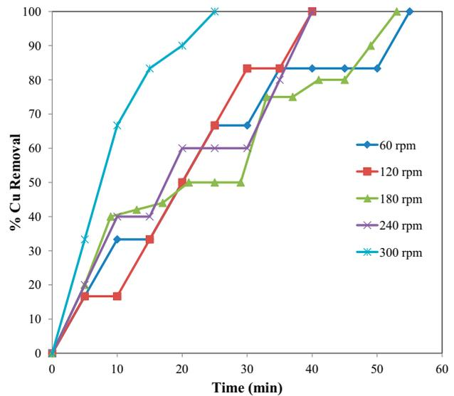
Fig. 4. Effect of speed of stirring,  $C_0 = 3$  g/L, 8 Fe electrodes, short cell, current = 250 mA, voltage = 12 V.
