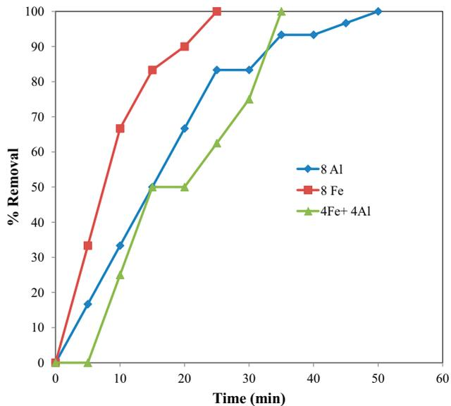
Fig. 6. Effect of material of sacrificial electrode,  $C_0 = 3 \text{ g/L}$ , stirring speed = 300 rpm, short cell, current = 250 mA, voltage = 12 V.
