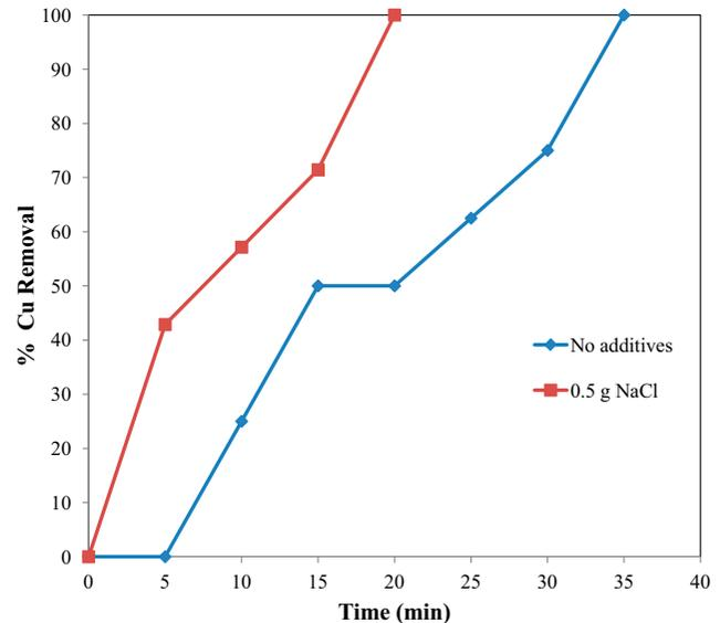
Fig. 7. Effect of presence of supporting electrolyte,  $C_0 = 3 \text{ g/L}$ , stirring speed = 300 rpm, Short cell, 4Al electrodes + 4Fe electrodes, current = 250 mA, voltage = 12 V.
