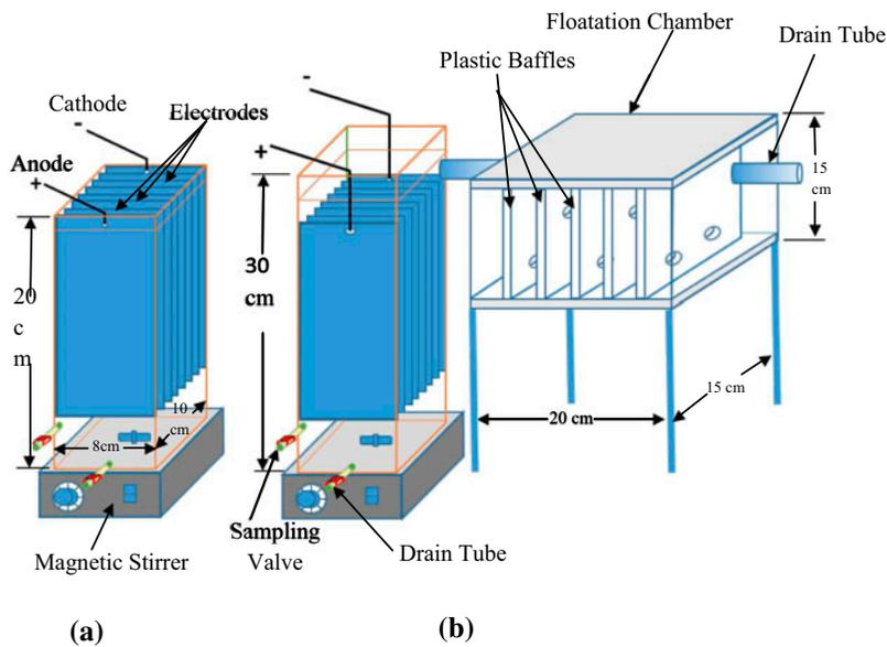
Fig. 1. Schematic diagram of set-up, (a) without FC and (b) with FC.
