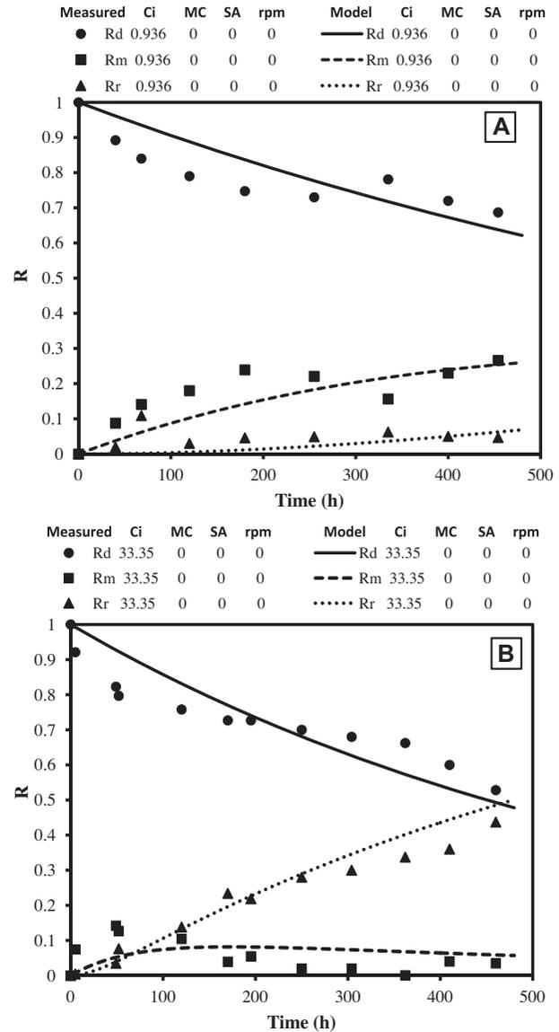
Fig. 3. Time variation of reduced concentrations of NaCl in DP, LM, and RP ( $R_d$ ,  $R_m$ , and  $R_r$ ) at MC = 0 for initial donor concentration (A) 0.936 g/l and (B) 33.35 g/l.
