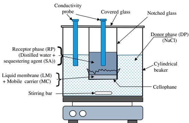
Fig. 1. Apparatus used in SLM experiments.
