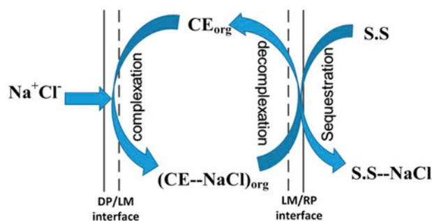
Fig. 2. Schematic of NaCl transport through the SLM.
