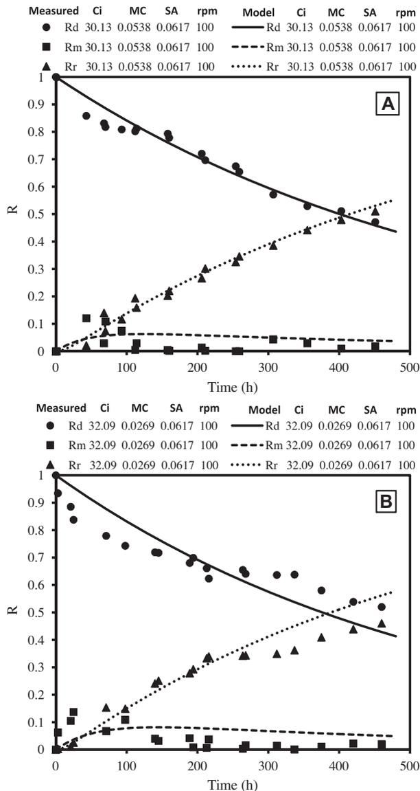
Fig. 5. Time variation of reduced concentrations of NaCl in DP, LM, and RP ( $R_d$ ,  $R_m$ , and  $R_r$ ) at  $C_i \cong 31$  g/l for quantity of MC (A) 0.0538 mol/l of LM and (B) 0.0269 mol/l of LM.
