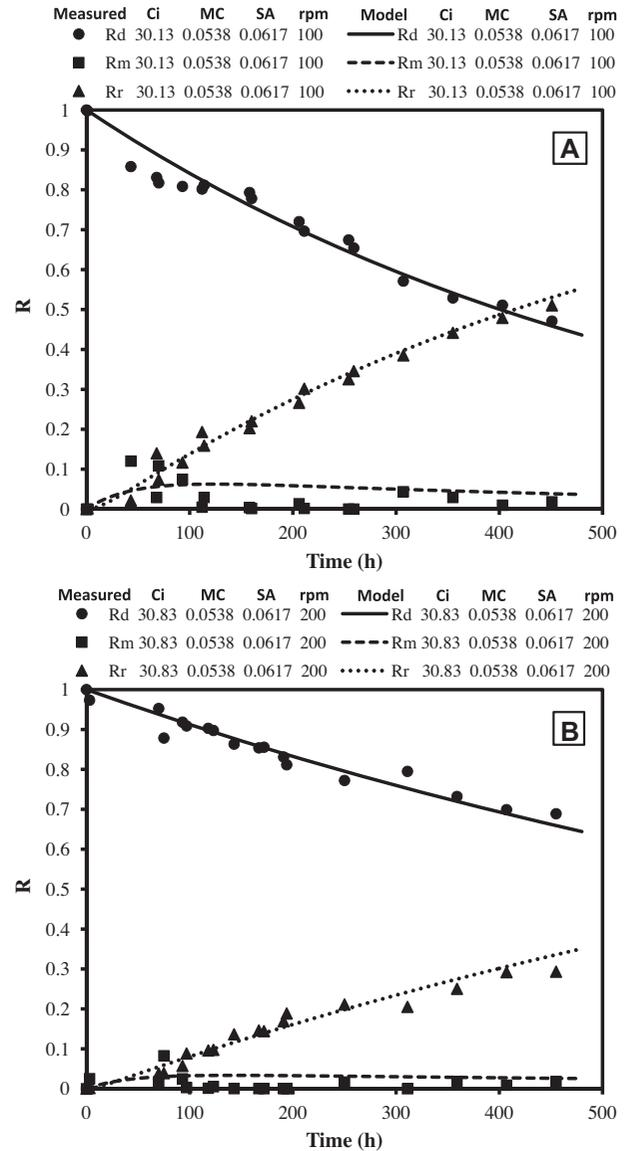
Fig. 6. Time variation of reduced concentrations of NaCl in DP, LM, and RP ( $R_d$ ,  $R_m$ , and  $R_r$ ) at  $C_i \cong 32$  g/l for quantity of MC (A) 0.0617 mol/L of RP and (B) 0.1233 mol/L of RP.
