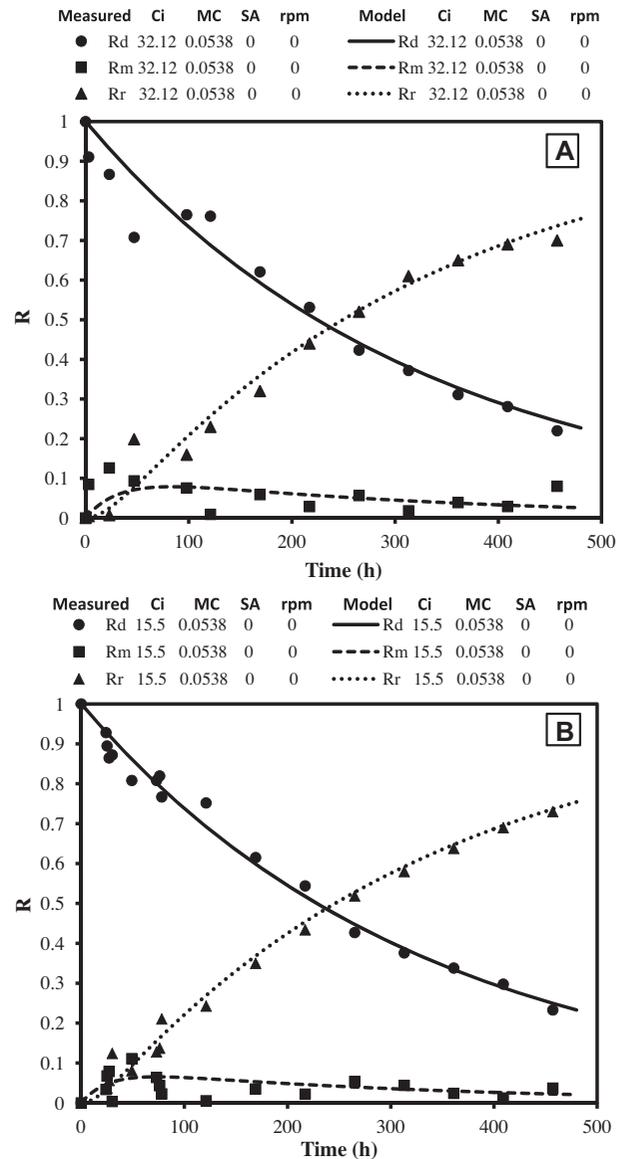
Fig. 4. Time variation of reduced concentrations of NaCl in DP, LM, and RP ( $R_d$ ,  $R_m$ , and  $R_r$ ) at MC = 0.0538 mol/l of LM for initial donor concentration (A) 32.12 g/l and (B) 15.5 g/l.
