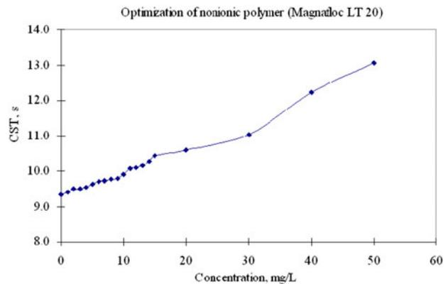
Fig. 5. Optimization of nonionic polymer (Magnafloc LT 20).
