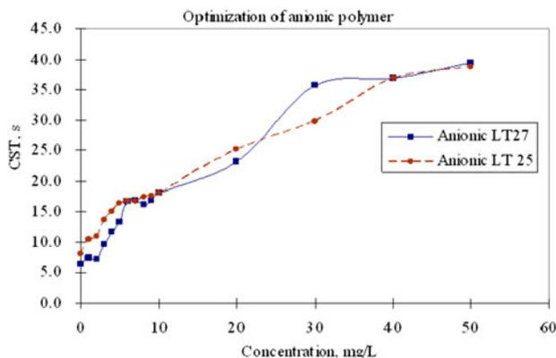
Fig. 4. Optimization of anionic polymer (Magnafloc LT 27 and LT 25).
