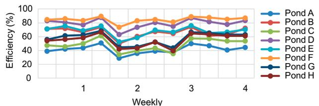
Fig. 20. Efficiency of BOD removal with time (Set 1,  $V_2$ ).
