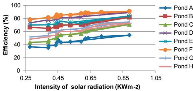
Fig. 45. Efficiency of BOD removal vs. solar intensity (Set 1,  $V_3$ ).
