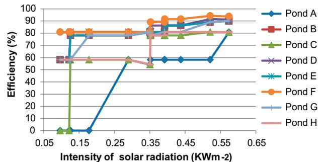
Fig. 43. Efficiency of coliform removal vs. solar intensity (Set 1,  $V_2$ ).
