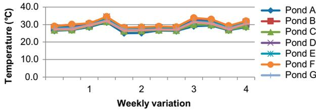
Fig. 14. Weekly temperature variation in ISHJEWSPs effluent with time (Set 1,  $V_2$ ).
