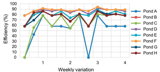
Fig. 34. Efficiency of coliform removal with time (Set 1,  $V_3$ ).
