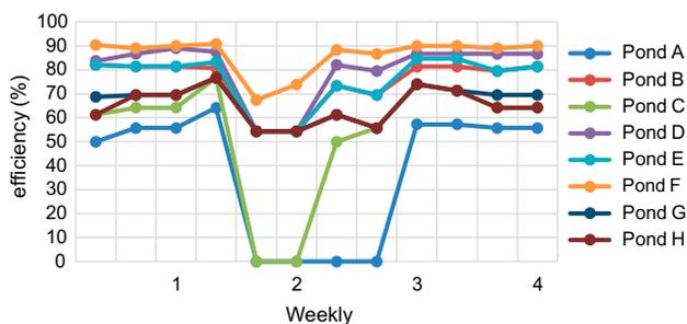
Fig. 24. Efficiency of E coli removal with time (Set 1, V<sub>2</sub>).
