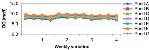
Fig. 13. Weekly DO variation in ISHJEWSPs effluent with time (Set 1,  $V_2$ ).
