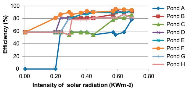
Fig. 39. Efficiency of coliform removal vs. solar intensity (Set 1,  $V_1$ ).
