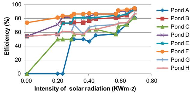
Fig. 40. Efficiency of E coli removal vs. solar intensity (Set 1,  $V_1$ ).
