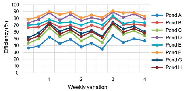
Fig. 32. Efficiency of BOD removal with time (Set 1,  $V_3$ ).
