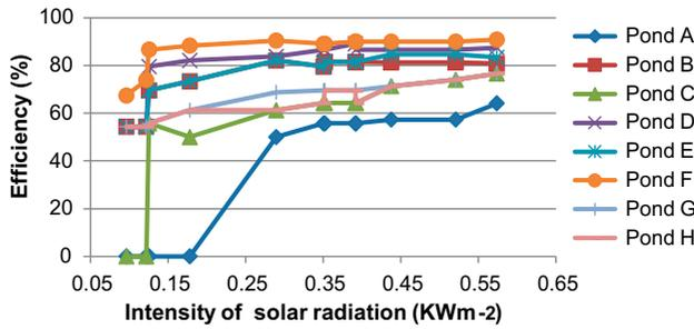
Fig. 44. Efficiency of E coli removal vs. solar intensity (Set 1,  $V_2$ ).
