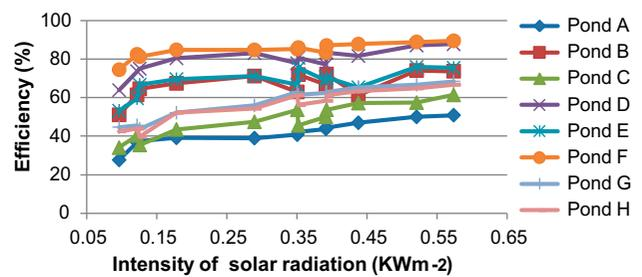
Fig. 41. Efficiency of BOD removal vs. solar intensity (Set 1,  $V_2$ ).
