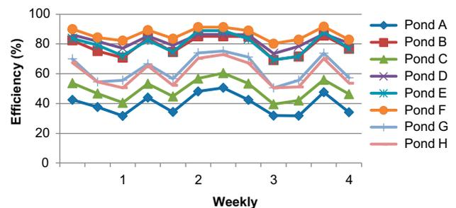
Fig. 6. Efficiency of suspended solids removal with time (Set 1,  $V_1$ ).
