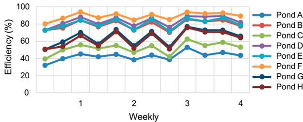
Fig. 30. Efficiency of suspended solids removal with time (Set 1,  $V_3$ ).
