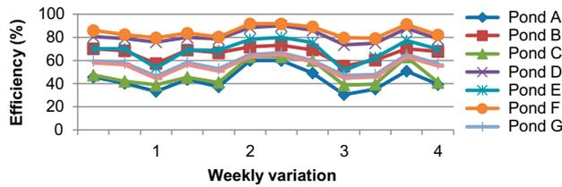
Fig. 8. Efficiency of BOD removal with time (Set 1,  $V_1$ ).
