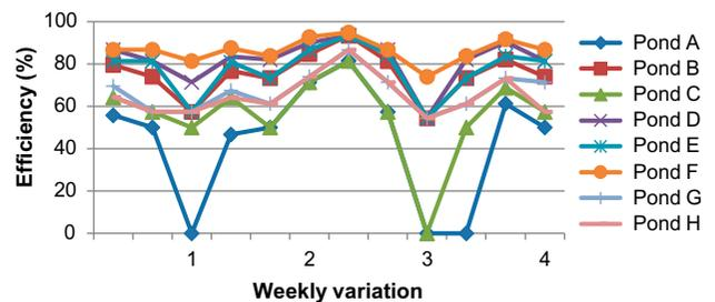
Fig. 12. Efficiency of E coli removal with time (Set 1,  $V_1$ ).
