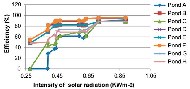
Fig. 48. Efficiency of E coli removal vs. solar intensity (Set 1,  $V_3$ ).
