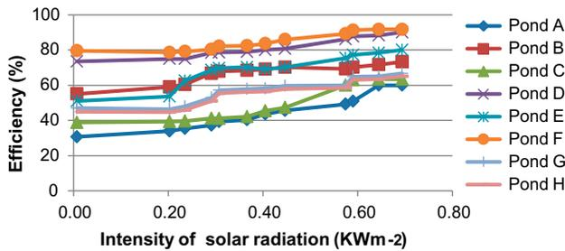
Fig. 37. Efficiency of BOD removal vs. solar intensity (Set 1,  $V_1$ ).
