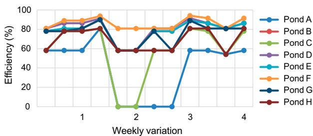
Fig. 22. Efficiency of coliform removal with time (Set 1, V<sub>2</sub>).
