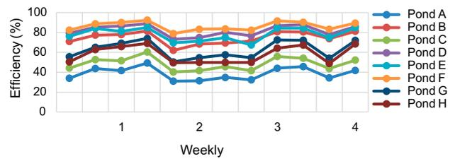
Fig. 18. Efficiency of suspended solids removal with time (Set 1,  $V_2$ ).
