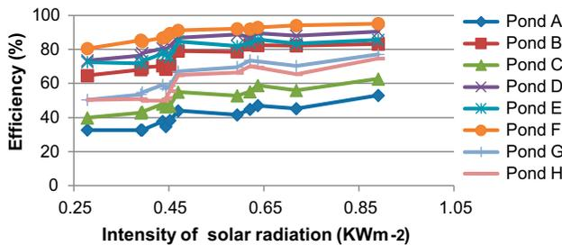
Fig. 46. Efficiency of suspended solids vs. solar intensity (Set 1,  $V_3$ ).
