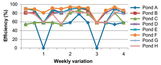
Fig. 10. Efficiency of coliform removal with time (Set 1,  $V_1$ ).
