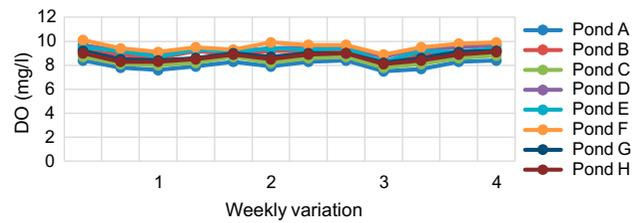
Fig. 25. Weekly DO variation in ISHJEWSPs effluent with time (Set 1, V<sub>3</sub>).
