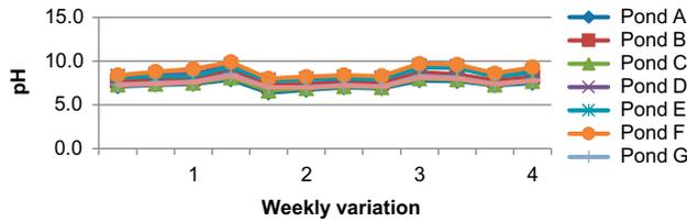
Fig. 15. Weekly pH variation in ISHJEWSPs effluent with time (Set 1,  $V_2$ ).
