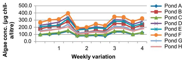
Fig. 16. Weekly algae concentration variation in ISHJEWSPs effluent with time (Set 1,  $V_2$ ).
