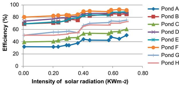
Fig. 38. Efficiency of suspended solids vs. solar intensity (Set 1,  $V_1$ ).
