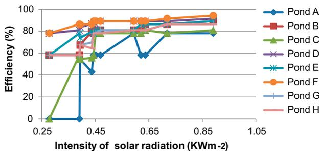
Fig. 47. Efficiency of coliform removal vs. solar intensity (Set 1,  $V_3$ ).
