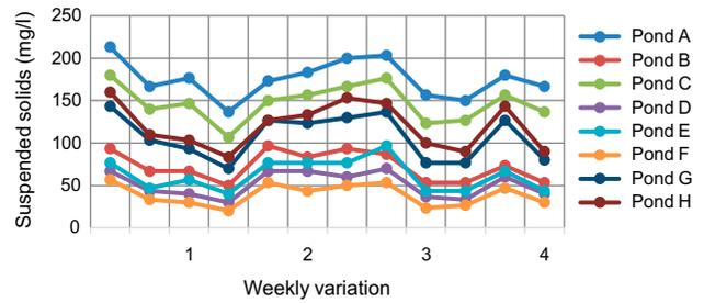
Fig. 17. Weekly suspended solids variation in ISHJEWSP with time (Set 1,  $V_2$ ).
