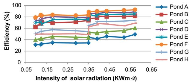
Fig. 42. Efficiency of suspended solids vs. solar intensity (Set 1,  $V_2$ ).
