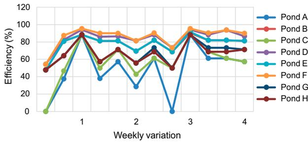
Fig. 36. Efficiency of E coli removal with time (Set 1,  $V_3$ ).
