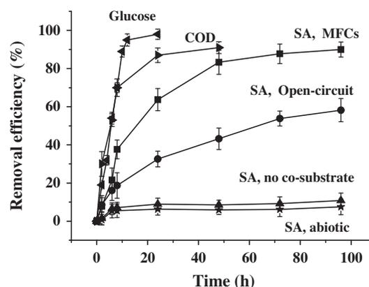
Fig. 5. Removal performances of sulfanilamide (30 mg L<sup>-1</sup>) in normal MFCs, open-circuit MFCs, no co-substrate MFCs, and abiotic MFCs (SA is short for sulfanilamide); glucose and COD removal performance in normal MFCs.
