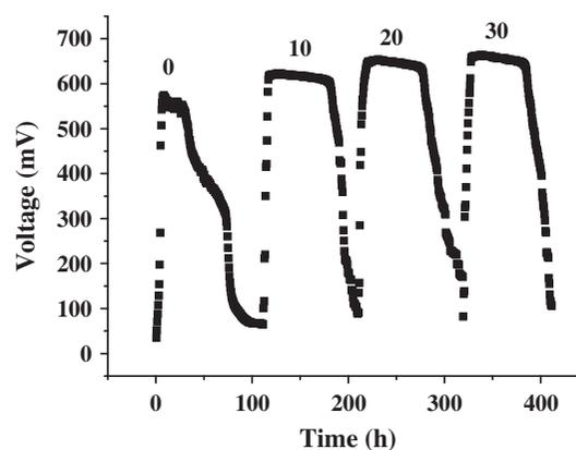
Fig. 2. Voltage generation from MFCs with 1 g L<sup>-1</sup> glucose and different concentration of sulfanilamide (numbers indicated the concentration of sulfanilamide, mg L<sup>-1</sup>) under external resistance of 1,000  $\Omega$ .
