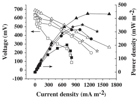
Fig. 3. Polarization (hollow symbol) and power density (solid symbol) curves of MFCs with  $1 \text{ g L}^{-1}$  glucose and different concentrations of sulfanilamide ( $0 \text{ mg L}^{-1}$ ,  $10 \text{ mg L}^{-1}$ ,  $20 \text{ mg L}^{-1}$ , and  $30 \text{ mg L}^{-1}$ ).
