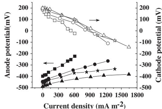
Fig. 4. Anode (solid symbol) and cathode (hollow symbol) polarization curves of MFCs with  $1 \text{ g L}^{-1}$  glucose and different concentrations of sulfanilamide ( $0 \text{ mg L}^{-1}$ ,  $10 \text{ mg L}^{-1}$ ,  $20 \text{ mg L}^{-1}$ , and  $30 \text{ mg L}^{-1}$ ).
