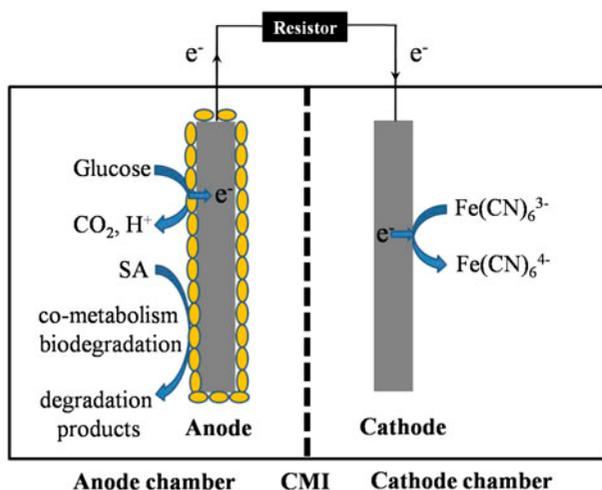
Fig. 1. Configuration of the two-chambered MFC (SA is short for sulfanilamide).
