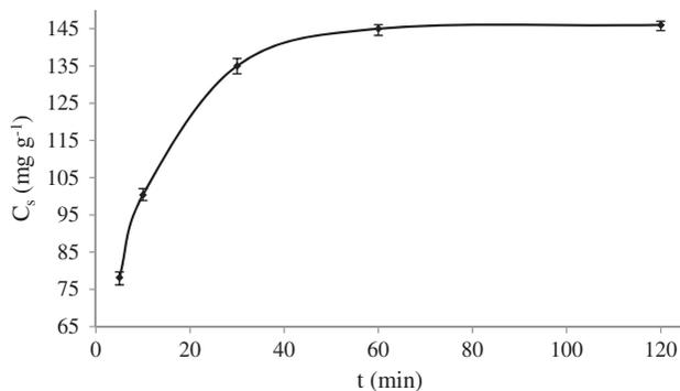
Fig. 3. Effect of contact time on the sorption of  $\text{Hg}^{2+}$  towards GMA-MMA-DVB-DTTA terpolymer sorbent ( $100 \mu\text{g L}^{-1}$   $\text{Hg}^{2+}$  solution, 20.0 mL sample volume, pH 6.0, 30.0 mg sorbent at  $25^\circ\text{C}$  sorption temperature).
