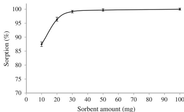
Fig. 2. Effect of GMA-MMA-DVB-DTTA terpolymer sorbent amount on sorption ( $100 \mu\text{g L}^{-1} \text{Hg}^{2+}$  solution, 20.0 mL sample volume, pH 6.0, 60 min contact time, at  $25^\circ\text{C}$  sorption temperature).
