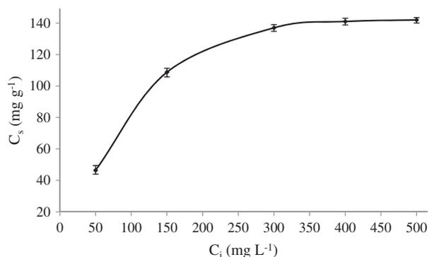
Fig. 4. Variation in the amount of  $\text{Hg}^{2+}$  sorbed with the initial concentration of  $\text{Hg}^{2+}$  solution (20.0 mL sample volume, pH 6.0, 60 min contact time, at 25°C sorption temperature).
