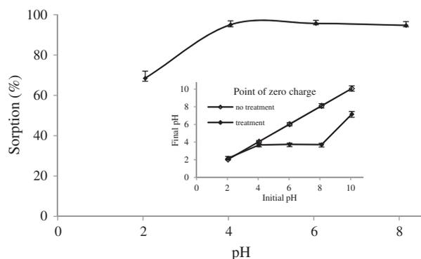
Fig. 1. Effect of pH on the sorption of  $\text{Hg}^{2+}$  towards GMA-MMA-DVB-DTTA terpolymer sorbent ( $100 \mu\text{g L}^{-1} \text{Hg}^{2+}$  solution, 20.0 mL sample volume, 2 hours contact time, 30.0 mg sorbent at  $25^\circ\text{C}$  sorption temperature).
