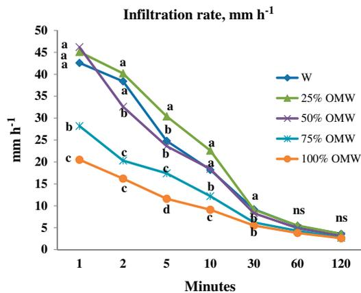
Fig. 1. Infiltration rate of diluted and undiluted OMW into the soil ( $\text{mm h}^{-1}$ ).
