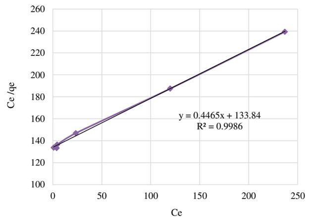
Fig. 7. Linearized Langmuir isotherms for  $\text{Cu}^{2+}$  adsorption by Fe-clinoptilolite.
