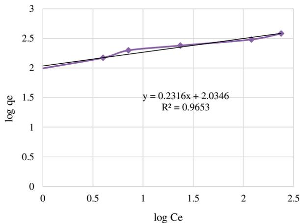
Fig. 8. Linearized Freundlich isotherms for  $\text{Cu}^{2+}$  adsorption by Fe-clinoptilolite.
