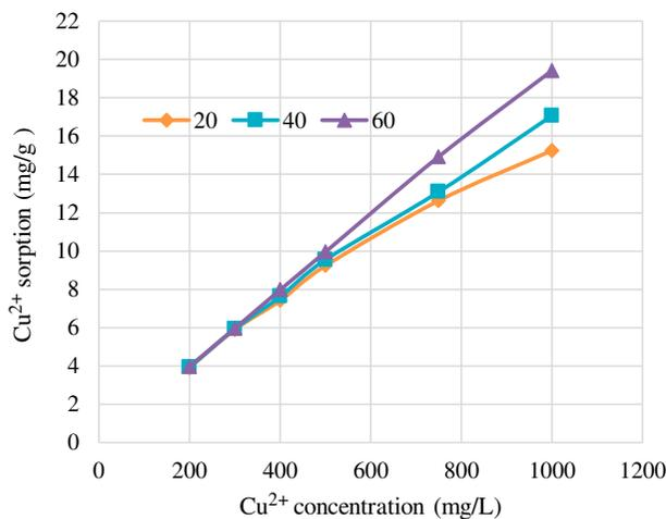
Fig. 6. Effect of temperature on  $\text{Cu}^{2+}$  adsorption ( $T = 20, 40, 60^\circ\text{C}$ , pH 3.5–5.5,  $S/L = 1/20$ ).
