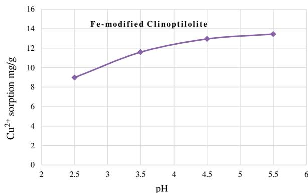
Fig. 4. Effect of initial pH on metal adsorption for ( $T = 20^\circ\text{C}$ , pH 2.5–5.5,  $S/L = 1/20$ ).
