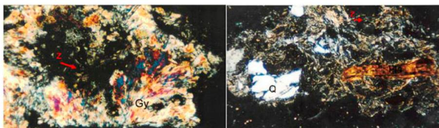
Fig. 1. Zeolite sample polish sections, Gy = Gypsum, Z = Zeolite, Q = quartz.
