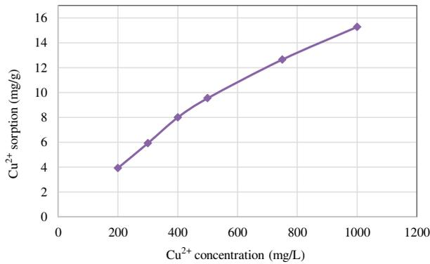
Fig. 5. Effects of metal concentration on metal adsorption ( $T = 20^\circ\text{C}$ , pH 4.5–5.5,  $S/L = 1/20$ ).
