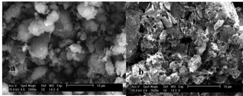
Fig. 3. SEM images of clinoptilolite before and after modification by  $\text{Fe}(\text{NO}_3)_3$  (a) natural clinoptilolite and (b) modified clinoptilolite by  $\text{Fe}(\text{NO}_3)_3$ .
