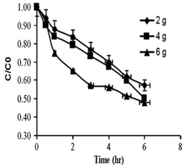
Fig. 7. Effect of increasing the catalyst load on beads.
