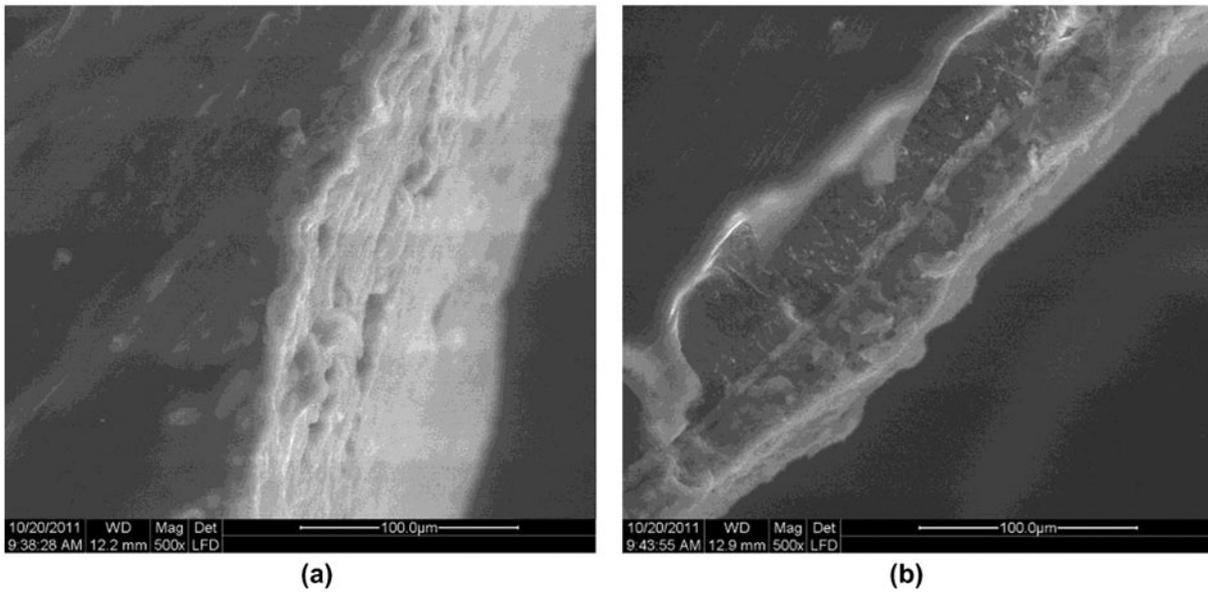
Fig. 5. TiO<sub>2</sub> coating thickness on different catalyst load (a) 2 g of TiO<sub>2</sub> coated on 200 g of beads and (b) 4 g of TiO<sub>2</sub> coated on 200 g of beads.
