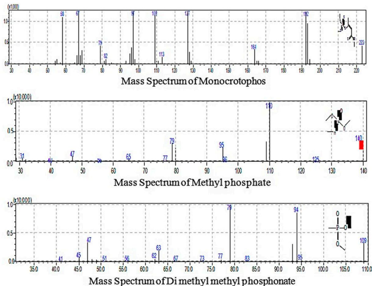
Fig. 9. GC–MS analysis of MCP and its intermediate degradation products formed in IBPR.
