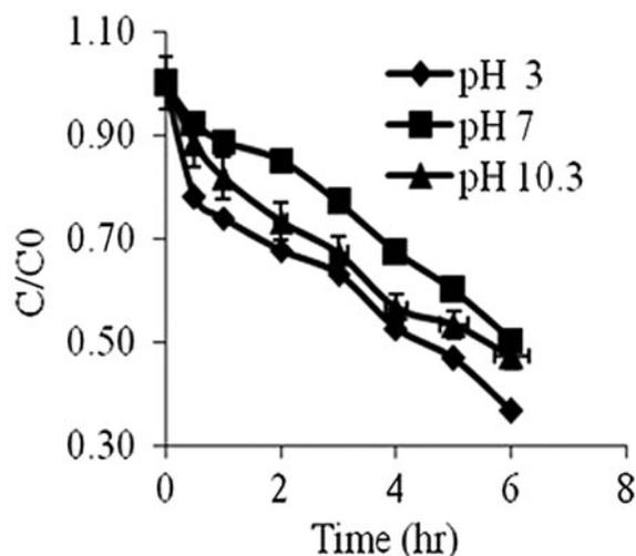
Fig. 4. Effect of pH on MCP degradation.
