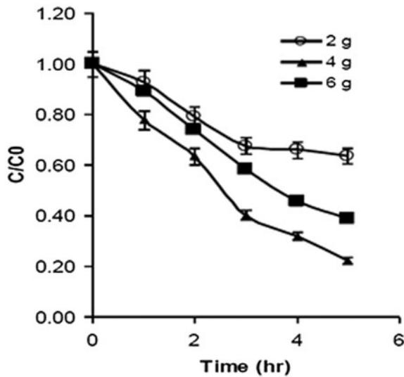
Fig. 6. Effect of increase in catalyst surface area (legend represents the increase in catalyst loading by changing number of beads).
