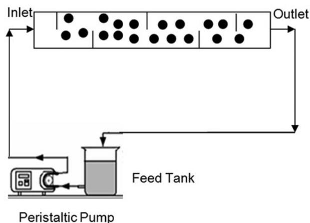
Fig. 1. Schematic representation of IBPR reactor.
