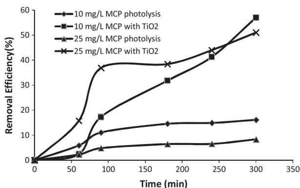
Fig. 2. Comparison of photolysis and photocatalysis on MCP.
