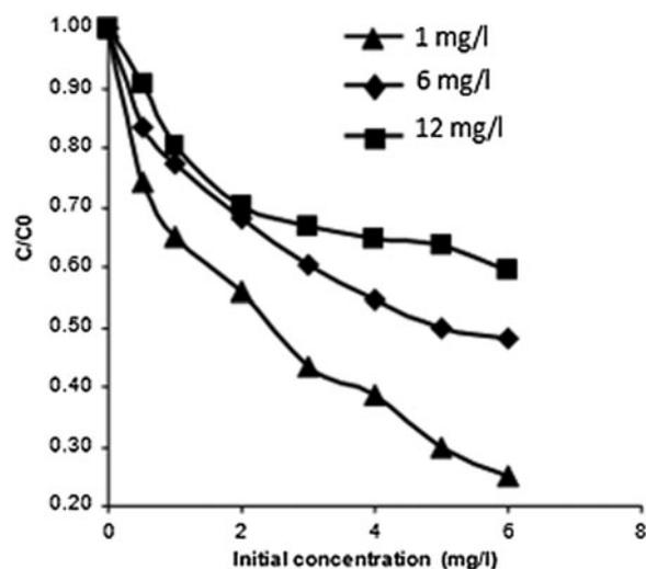
Fig. 3. Effect of initial concentration on MCP degradation.
