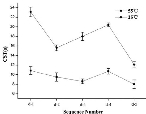
Fig. 2. CST evolution of sludge as a function of temperature and dosages (d-1:4 mg/g DS FeCl<sub>3</sub> and 25 mg/g DS Steel slag; d-2:4 mg/g DS FeCl<sub>3</sub> and 50 mg/g DS Steel slag; d-3:5.5 mg/g DS FeCl<sub>3</sub> and 37.5 mg/g DS Steel slag; d-4:7 mg/g DS FeCl<sub>3</sub> and 25 mg/g DS Steel slag; d-5:7 mg/g DS FeCl<sub>3</sub> and 50 mg/g DS Steel slag).
