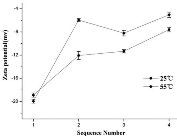
Fig. 3. Zeta potential evolution of sludge as a function of dosage under mild thermal treatment at 25 and 55°C (1–0; 2–50 mg/g DS Steel slag; 3–5.5 mg/g DS FeCl<sub>3</sub>; 4–5.5 mg/g DS FeCl<sub>3</sub> and 50 mg/g DS Steel slag).
