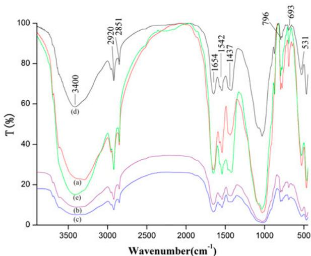
Fig. 4. FT-IR spectra of the sludge with different dosages and temperatures (a) 0; (b) 50 mg/g Steel slag; (c) 5.5 mg/g DS FeCl<sub>3</sub>; (d) 5.5 mg/g DS FeCl<sub>3</sub> and 50 mg/g DS Steel slag; (e) 5.5 mg/g DS FeCl<sub>3</sub> and 50 mg/g DS Steel slag; (a), (b), (c), (d) under 55°C; (e) under 25°C).
