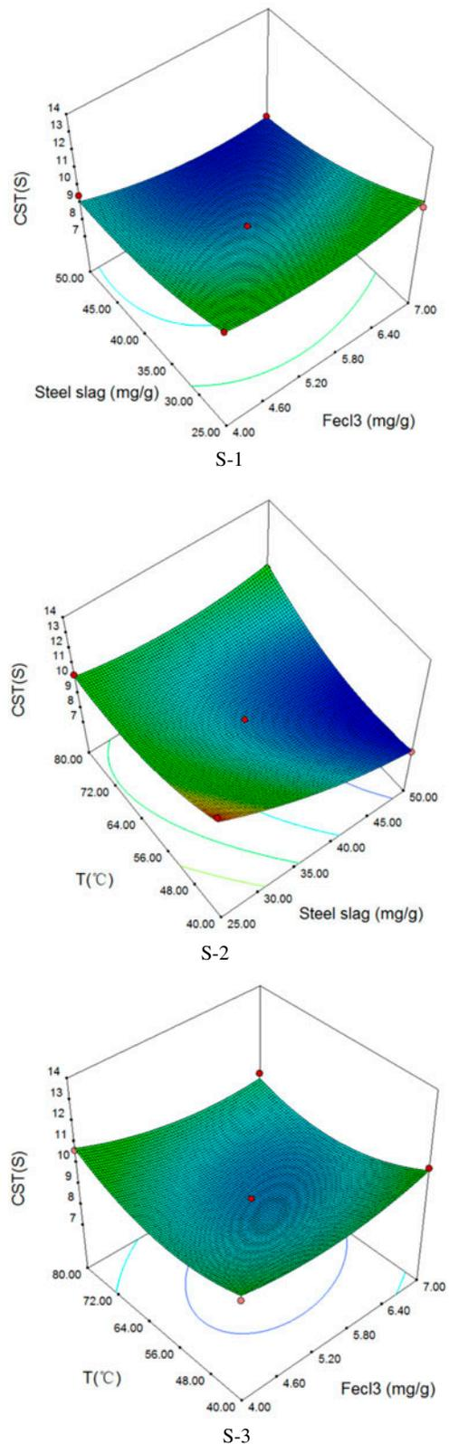
Fig. 1. Response surface plots: S-1 dosage of steel slag and  $\text{FeCl}_3$ ; S-2 dosage of steel slag and temperature; S-3 dosage of  $\text{FeCl}_3$  and temperature.
