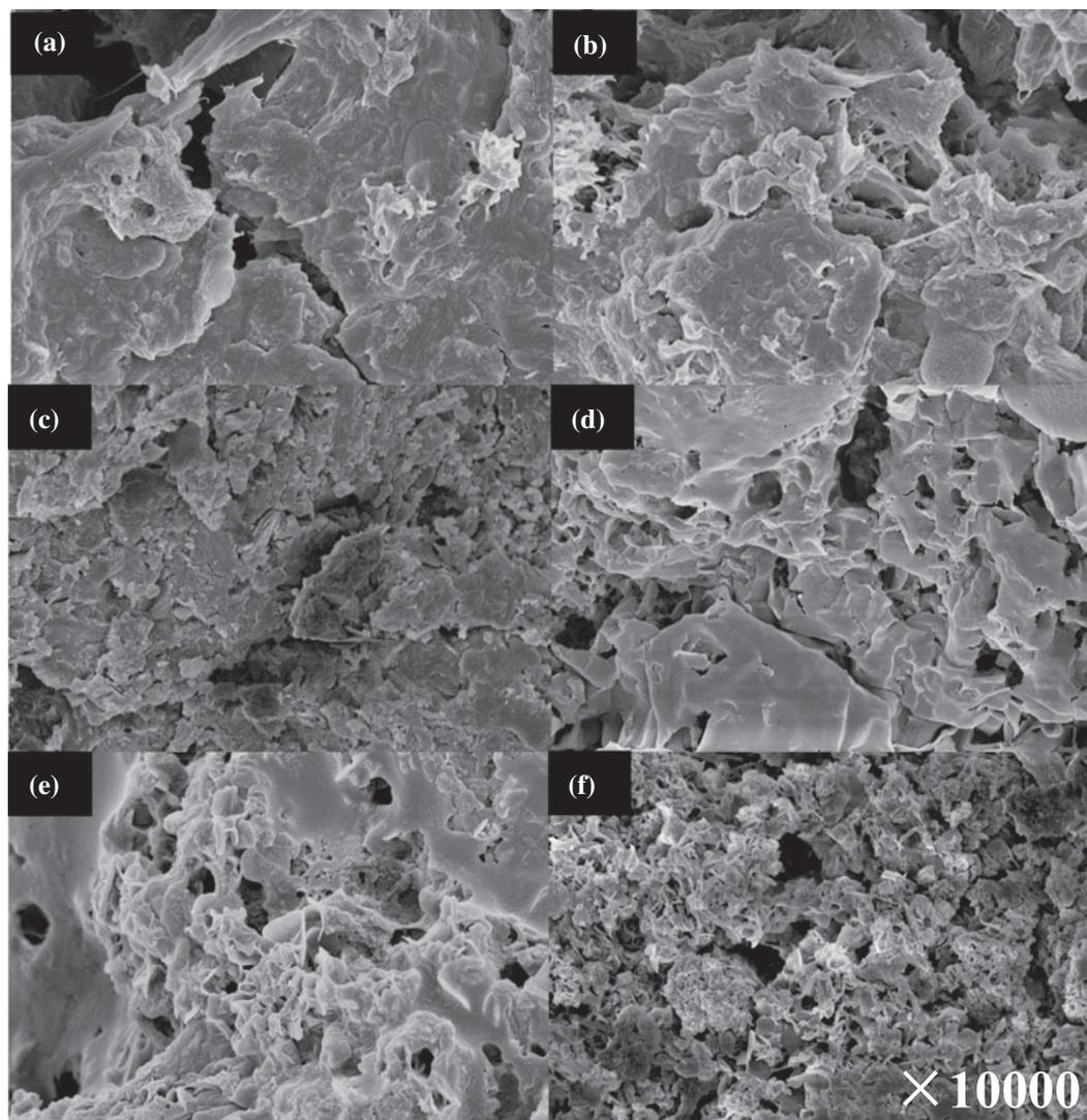
Fig. 5. SEM images of (a), (b) raw sludge; (c) conditioned by 5.5% FeCl<sub>3</sub>; (d) conditioned by 50% Steel slag; (e), (f) conditioned by 5.5% FeCl<sub>3</sub> and 50% Steel slag; (a), (e) under 25 °C; (b), (c), (d), (f) under 55 °C.
