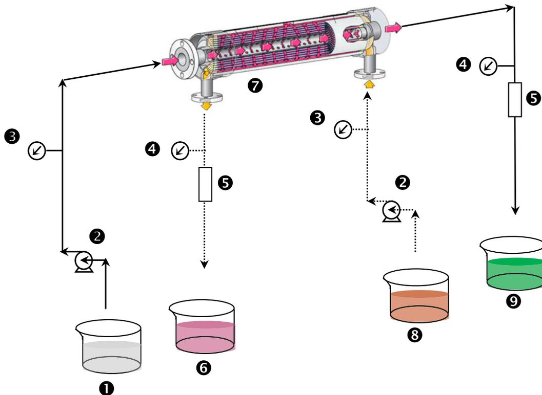
Fig. 2. Schematic counter-current flow diagram for one-through-mode operation in a HFSLM. 1. inlet feed solution reservoir, 2. gear pump, 3. inlet pressure gages, 4. outlet pressure gages, 5. flow meters, 6. outlet stripping solution reservoir, 7. hollow fiber module, 8. inlet stripping solution reservoir, and 9. outlet feed solution.
