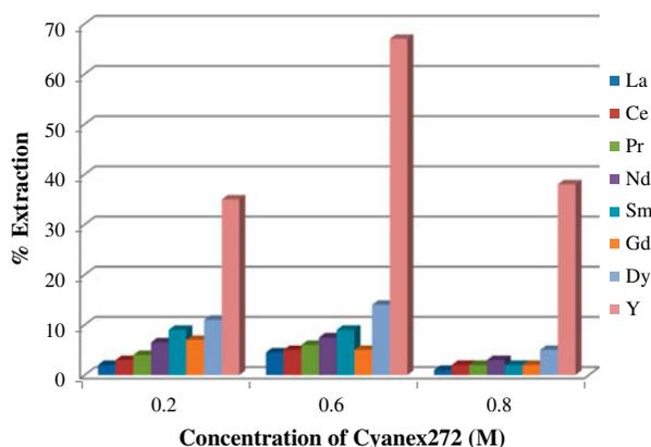
Fig. 3. Extractabilities of rare earth ions by Cyanex272.
