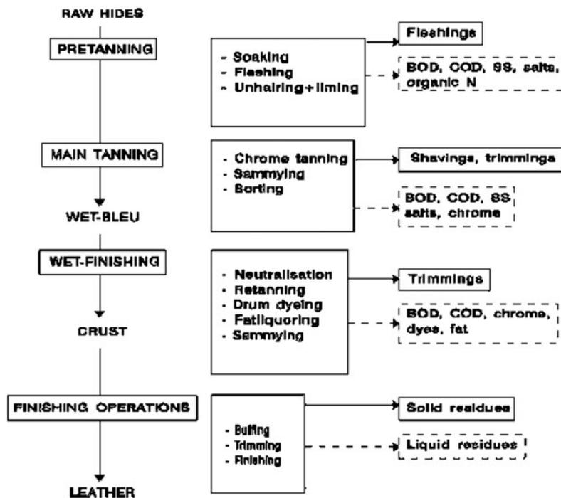
Fig. 1. Production of wastewater at various stages of tannery industry processing.
