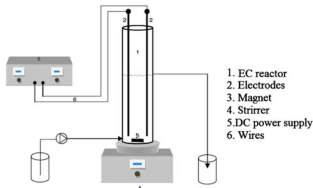
Fig. 2. Schematic diagram of EC reactor.
