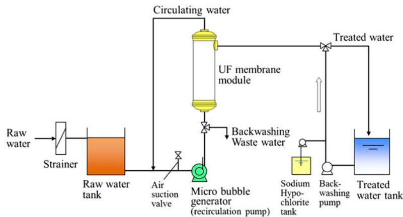
Fig. 2. Schematic diagram of the membrane filtration equipment in the pilot plant with microbubble generator.
