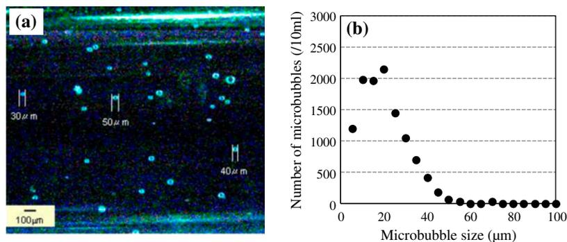
Fig. 4. (a) Optical image of MBs, taken via CCD camera. (b) Distribution of MB size measured by optical particle counter.
