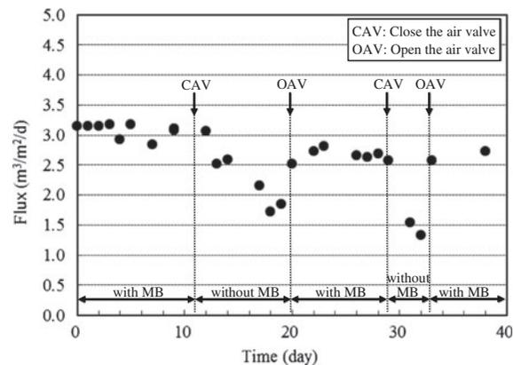
Fig. 8. Effect of MB addition during filtration over a long-time period.
