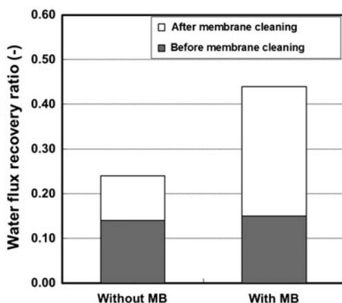
Fig. 9. Effect of MB addition on the membrane cleaning.
