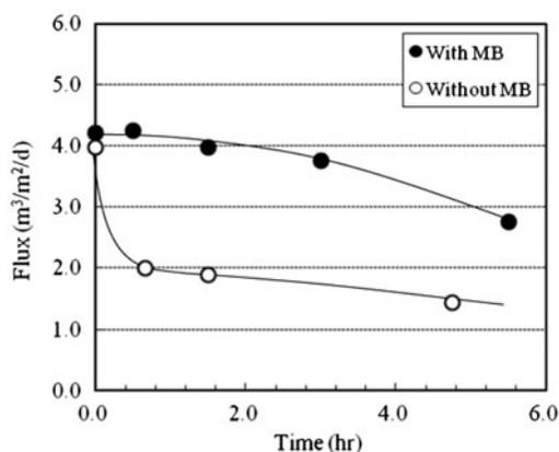
Fig. 5. Effect of MB addition on filtration flux during filtration over a short-time period. Flow velocity: 0.16 m/s.
