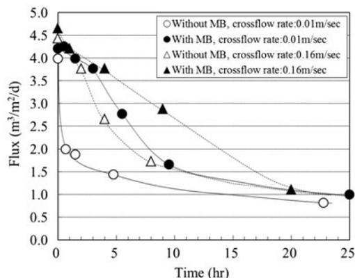
Fig. 7. Influence of flow velocity on the effectiveness of MB addition.
