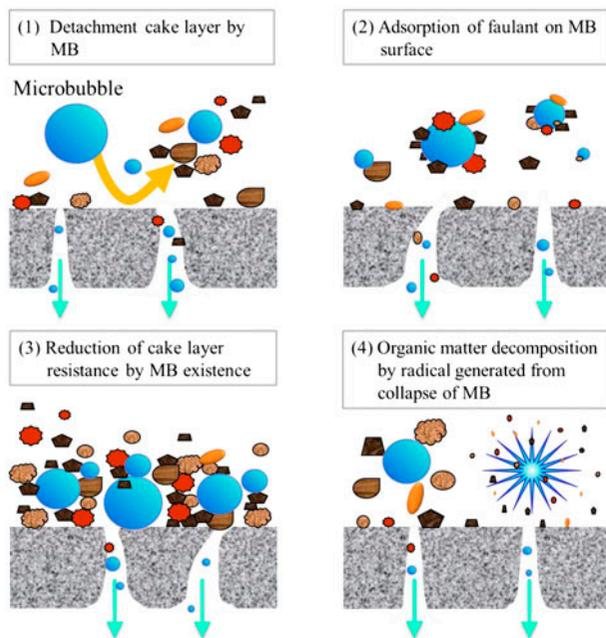
Fig. 6. Possible mechanisms by which MBs reduce fouling.
