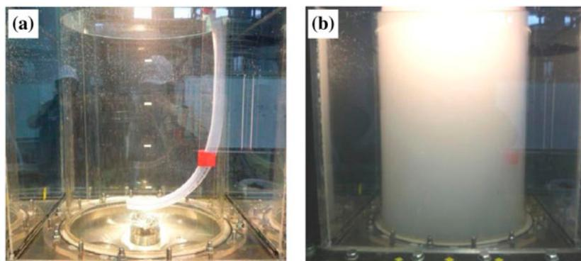
Fig. 3. MBs generated in pure water: (a) Before generation and (b) During generation.
