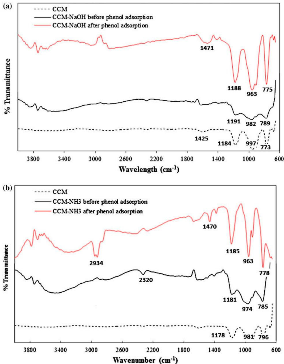
Fig. 1. FT-IR spectra of modified CCM: (a) CCM-NaOH and (b) CCM-NH<sub>3</sub>.
