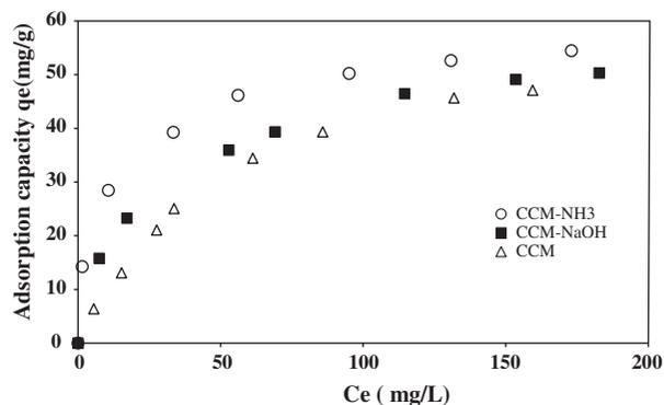
Fig. 7. Comparison of equilibrium adsorption capacities between unmodified CCM [8] and modified CCM.
