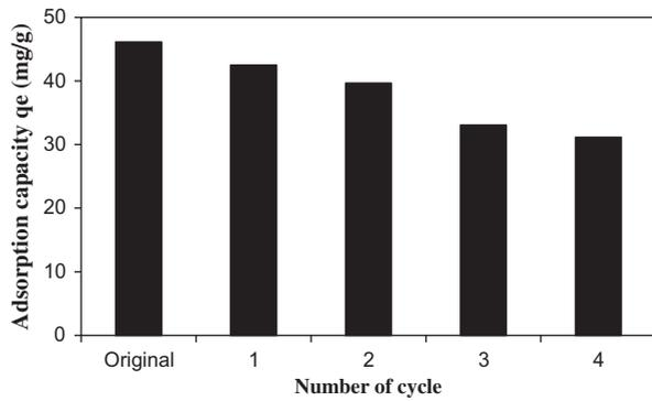
Fig. 8. Regeneration studies plot of CCM-NH<sub>3</sub>. (Conditions: initial phenol concentration—200 mg L<sup>-1</sup>, speed of shaker—200 rpm, temperature—30°C, and contact time—24 h).
