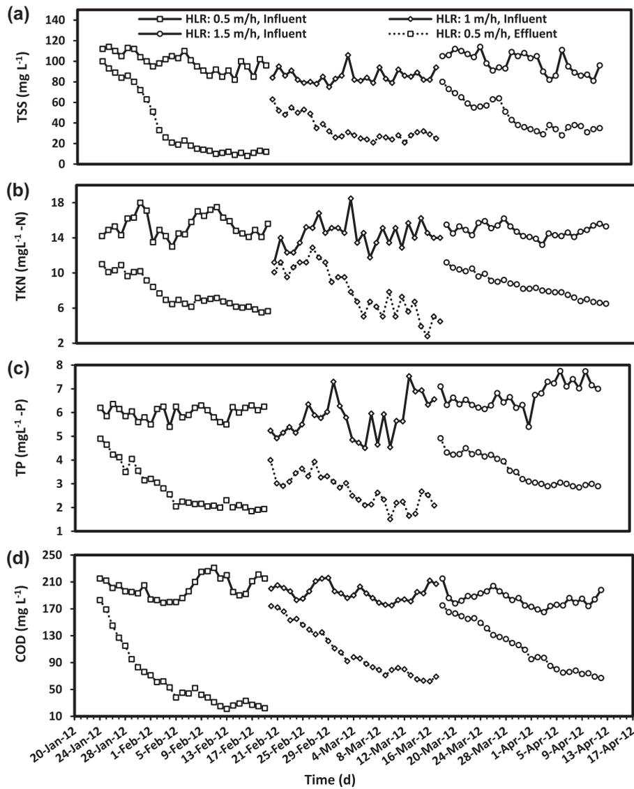
Fig. 3. Values of (a) SS, (b) TKN, (c) TP, and (d) COD from influent and effluent flows of HRF during three subsequent  $V_f$  (0.5, 1, and 1.5 m<sup>3</sup> m<sup>-2</sup> h<sup>-1</sup>).
