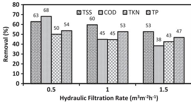
Fig. 2. Removal efficiencies of TSS, COD, TKN, and TP in three hydraulic filtration rates (0.5, 1, and 1.5 m<sup>3</sup> m<sup>-2</sup> h<sup>-1</sup>).
