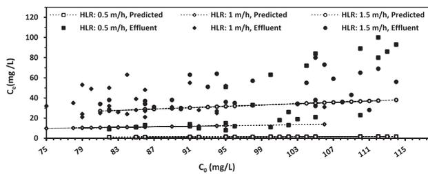
Fig. 4. Comparison of observed vs. predicted TSS in effluent for various filtration rates.
