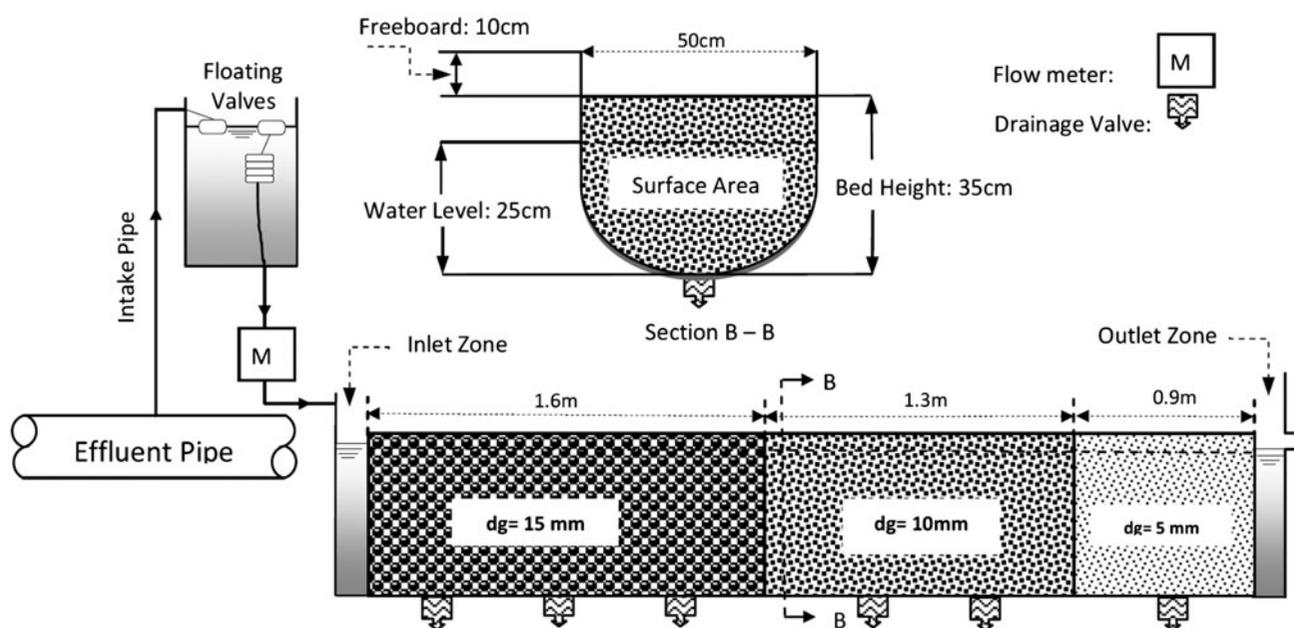
Fig. 1. Schematic layout and details of HRF pilot system.
