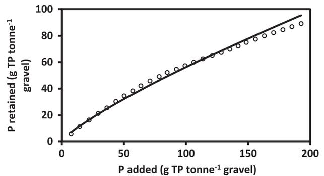
Fig. 5. The relationship between added and retained phosphorous during the first filtration rate ( $V_f = 0.5 \text{ m}^3 \text{m}^{-2} \text{h}^{-1}$ ).
