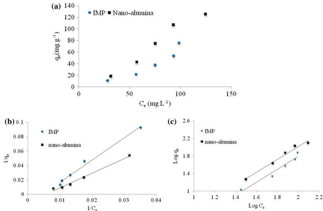
Fig. 4. (a) The adsorption of nitrate on the IMP and nanoalumina, (b) Langmuir, and (c) Freundlich isotherm of nitrate sorption on nanoalumina and IMP. pH 5; contact time, 60 min; IMP dose  $0.5 \text{ g L}^{-1}$ ; and nanoalumina dose  $0.25 \text{ g L}^{-1}$ .
