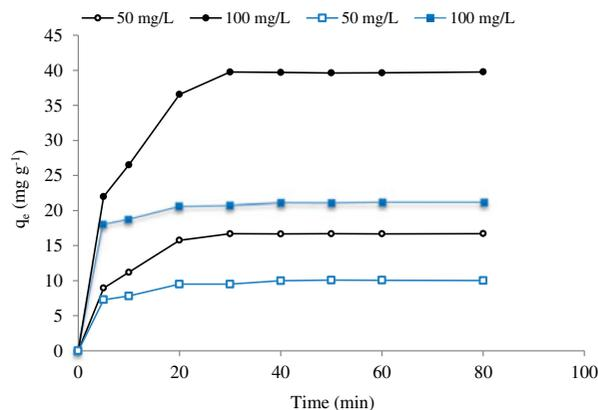
Fig. 1. Effect of contact time on the removal of nitrate by nanoalumina (●) and IMP (■).
