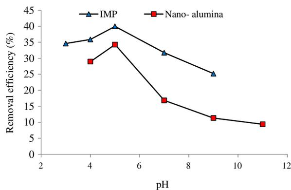
Fig. 2. Effect of pH on nitrate sorption on nanoalumina and IMP (temperature = 20°C, contact time = 30 min, sorbent dose = nanoalumina (0.25  $\text{g L}^{-1}$ ), IMP (0.5  $\text{g L}^{-1}$ ), and  $\text{NO}_3$  concentration = 50  $\text{mg L}^{-1}$ ).
