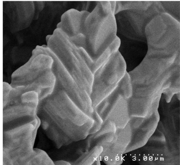
Fig. 6. SEM micrograph of supports sintered at 1,000°C for 3 h.
