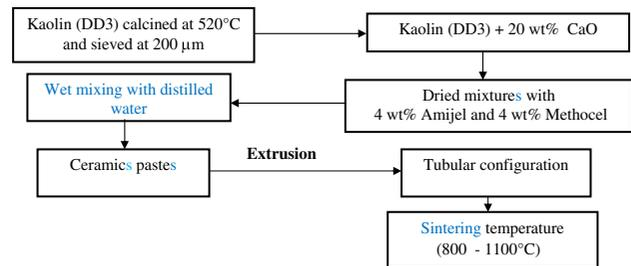
Fig. 2. The main steps of the processing route for tubular supports preparation.
