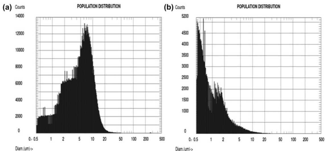
Fig. 1. Particle size distribution of powders used in this work. (a) calcite powder and (b) kaolin powder (DD3).
