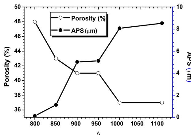
Fig. 4. Effect of sintering temperature on porosity (%) and APS of supports.
