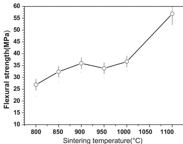
Fig. 7. Effect of sintering temperature on Flexural strength of supports.
