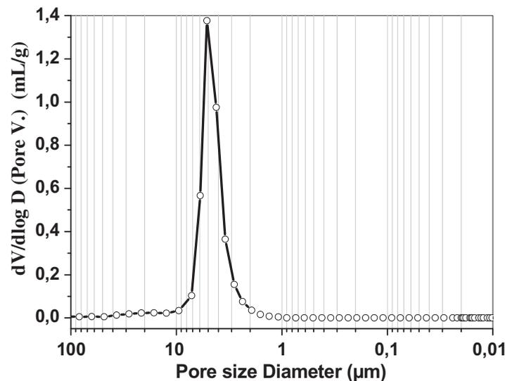
Fig. 5. Pore size distribution of supports sintered at 1,000°C for 3 h.
