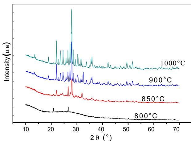
Fig. 3. The XRD spectra for samples sintered at different temperatures for 3 h.
