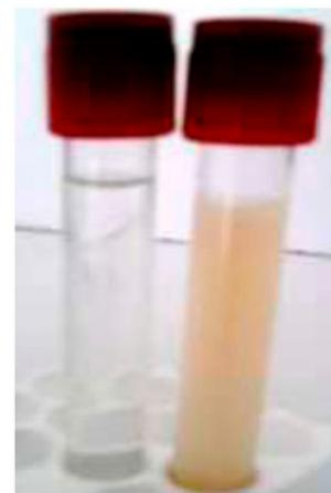
Fig. 6. A photograph of wastewater before and after the support MF treatment.
