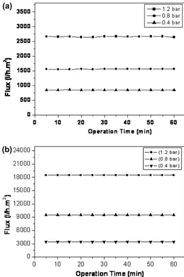
Fig. 5. Permeate flux versus time, at 3 working pressure values, using distilled water for S1 and S2 sintered at 1,150 and 1,250°C for 1 h, respectively.
