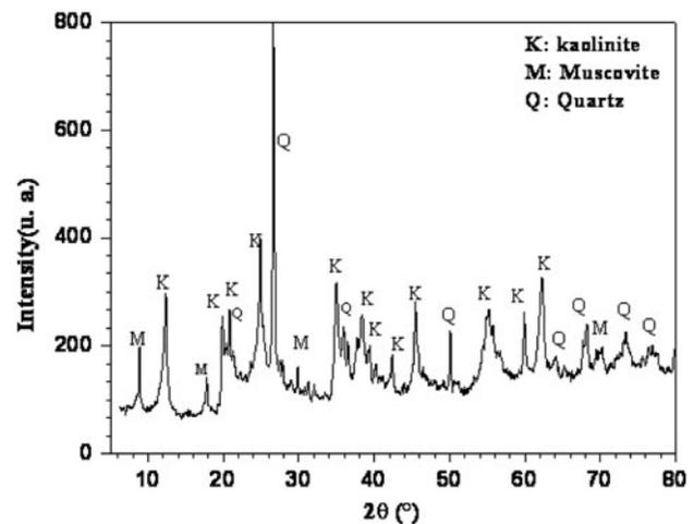
Fig. 1. XRD spectrum of used clay powders.
