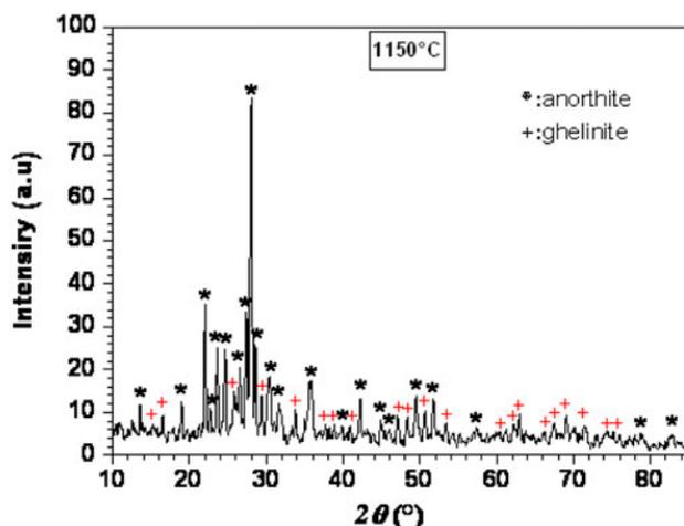
Fig. 3. XRD spectrum of prepared supports sintered at 1,150°C, for 1 h.
