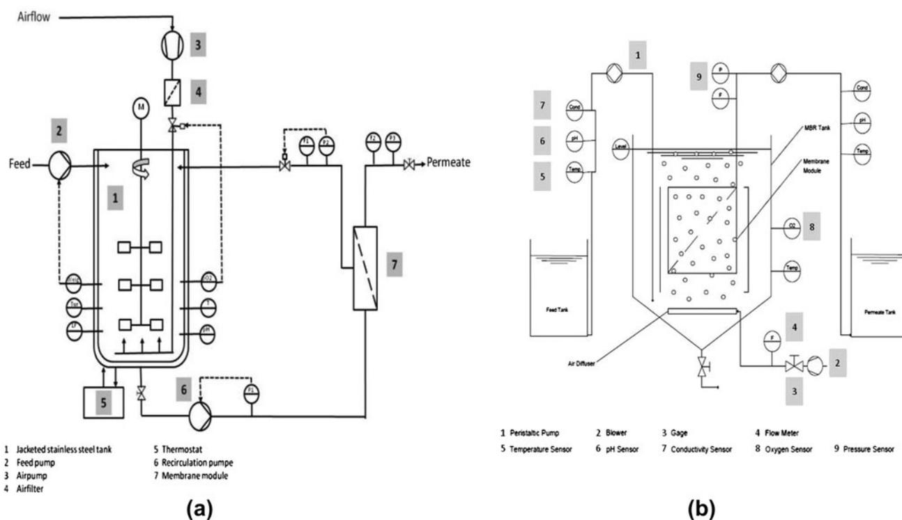
Fig. 1. Schematic representation of laboratory MBR (a) side-stream and (b) submerged.
