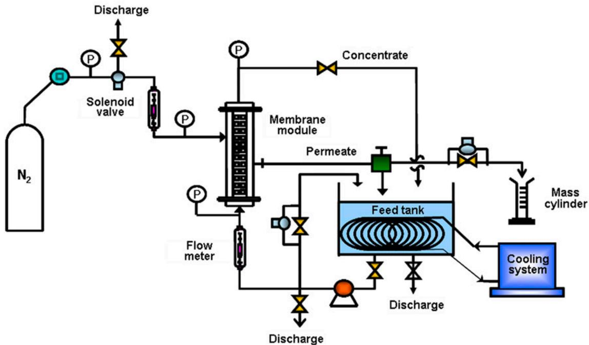
Fig. 1. Apparatus of hybrid water treatment process of tubular ceramic UF and  $\text{TiO}_2$  photocatalyst-coated PP beads with periodic air backflushing [27].
