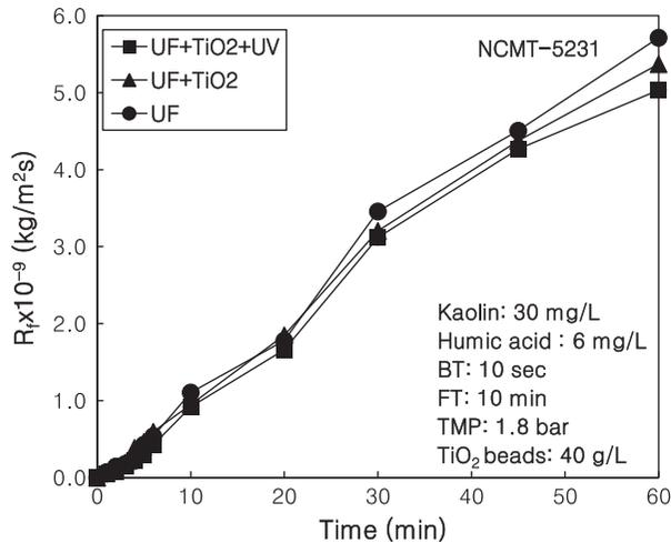
Fig. 4. Roles of membrane filtration, adsorption, and photo-oxidation on resistance of membrane fouling in hybrid process of tubular ceramic UF and  $\text{TiO}_2$  photocatalyst-coated PP beads.
