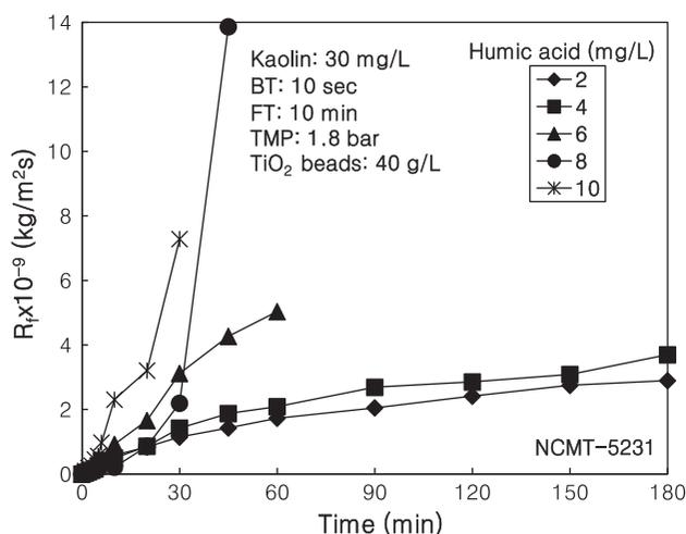
Fig. 2. Effect of HA on resistance of membrane fouling in hybrid process of tubular ceramic UF and TiO<sub>2</sub> photocatalyst-coated PP beads.
