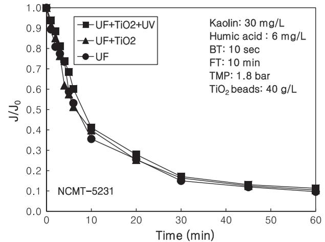
Fig. 5. Roles of membrane filtration, adsorption, and photo-oxidation on dimensionless permeate flux in hybrid process of tubular ceramic UF and  $\text{TiO}_2$  photocatalyst-coated PP beads.
