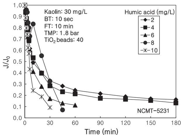
Fig. 3. Effect of HA on dimensionless permeate flux in hybrid process of tubular ceramic UF and TiO<sub>2</sub> photocatalyst-coated PP beads.
