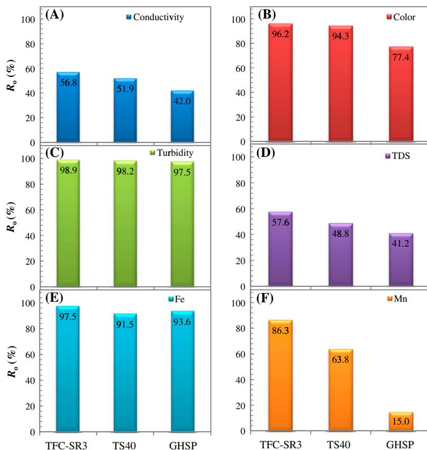
Fig. 7. Rejection of (A) conductivity; (B) color; (C) turbidity; (D) total dissolved solids (TDS); (E) Fe; and (F) Mn from natural groundwater using NF and UF membranes.
