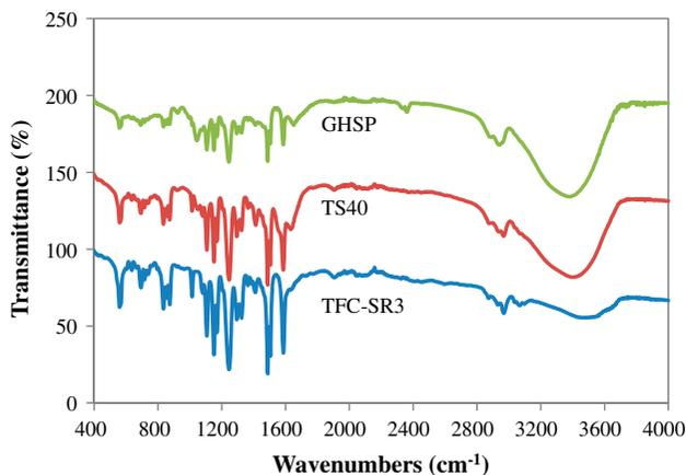
Fig. 4. FTIR spectra of clean NF (TFC-SR3 and TS40) and UF (GHSP) membranes.
