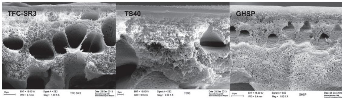
Fig. 3. FESEM images of the cross-sectional morphologies of clean NF and UF membranes.
