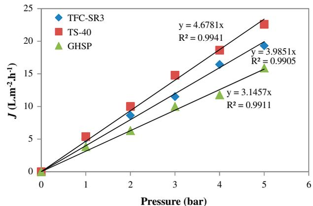
Fig. 5. Pure water flux of NF and UF membranes.
