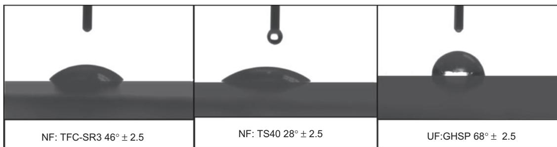
Fig. 1. Water drop contact angle  $\theta^\circ$  as a function of membrane surface hydrophilicity.
