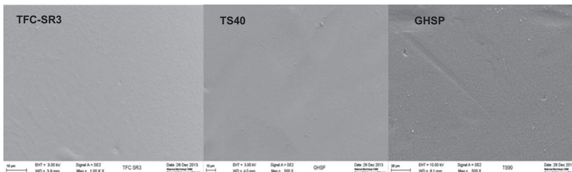
Fig. 2. FESEM images of the membrane surfaces of clean NF and UF membranes.
