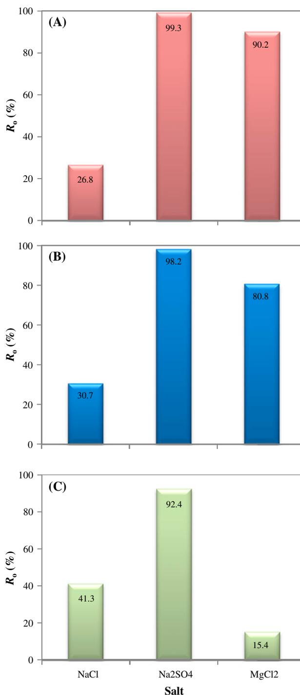
Fig. 6. Rejection of salt solutions (NaCl,  $\text{Na}_2\text{SO}_4$ , and  $\text{MgCl}_2$ ) by (A) TFC-SR3; (B) TS40; and (C) GHSP membranes at operating condition: 1,000 ppm salt, 5.0 bar, 25 °C.
