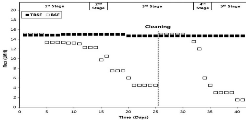
Fig. 6. Flux decline with operation.
