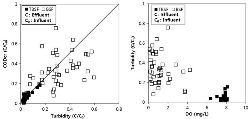
Fig. 5. Turbidity, CODcr vs. DO in standing water.
