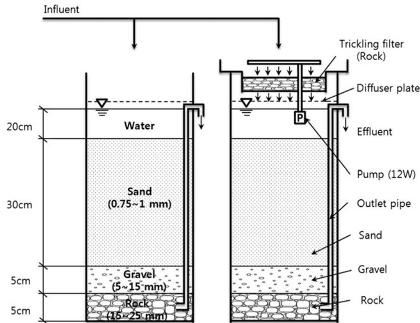
Fig. 1. BSF (left) and TBSF (right).
