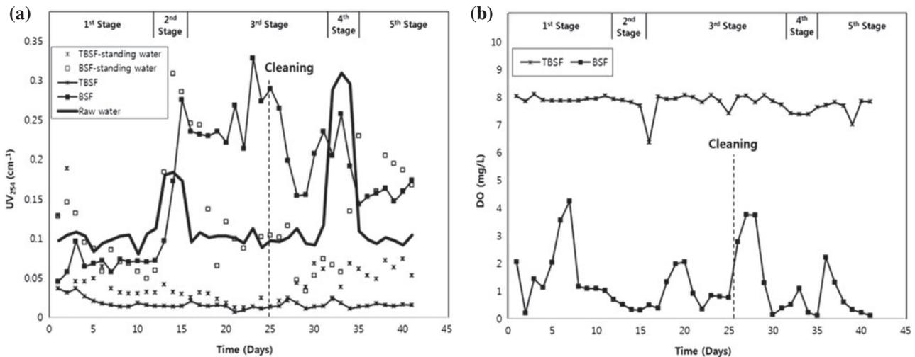
Fig. 7.  $UV_{254}$  and DO changes for operation. (a)  $UV_{254}$  to standing water and effluent and (b) DO changes for operation.
