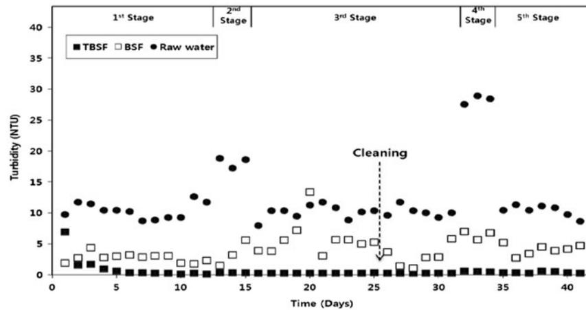
Fig. 4. Result of turbidity in TBSF/BSF operation.
