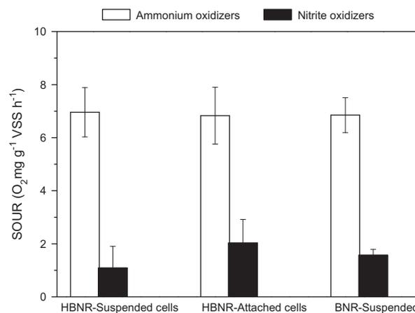
Fig. 5. Results of SOUR test in the aerobic tanks of HBNR and BNR (unit of SOUR is  $\text{mg O}_2 \text{ gVSS}^{-1} \text{ h}^{-1}$ ).
