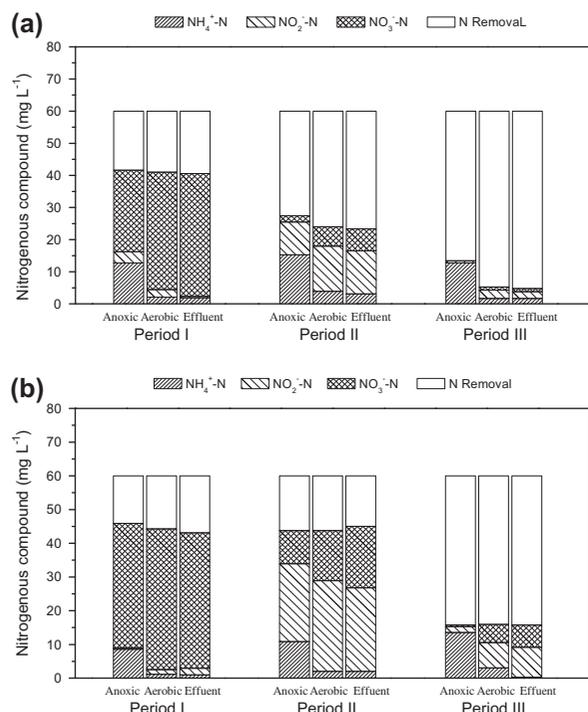
Fig. 4. Typical variation of nitrogen species concentrations along the HBNR (a), and BNR (b) during three periods in stable stage.
