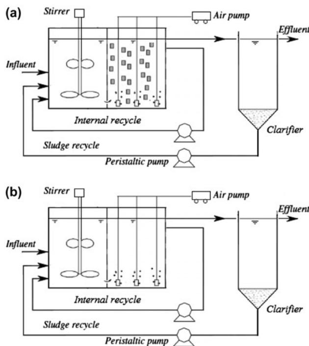
Fig. 1. Schematics of HBNR (a) and BNR (b) reactors.
