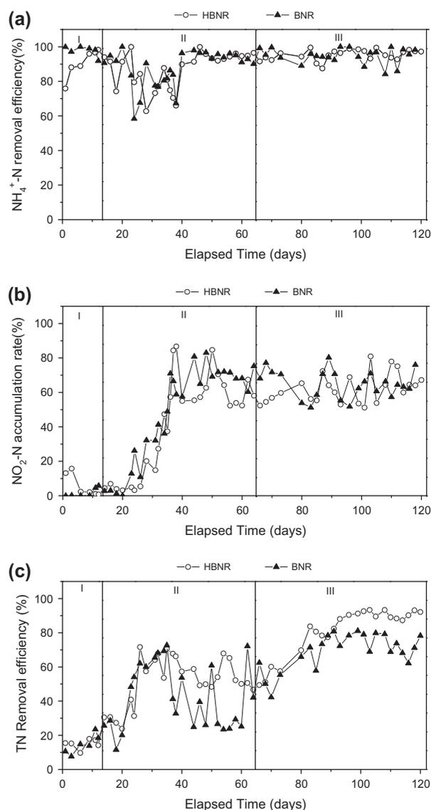
Fig. 3. Profiles of  $\text{NH}_4^+\text{-N}$  removal efficiency (a), NAR (b), and TN removal efficiency (c) in the HBNR and BNR.
