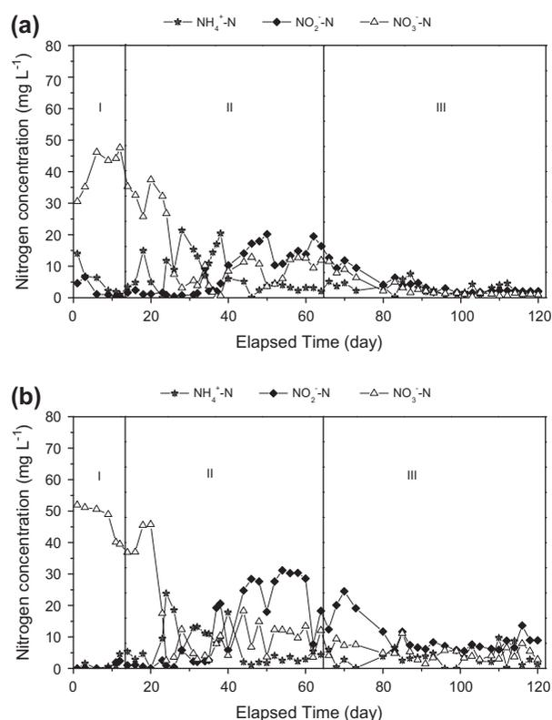
Fig. 2. Concentration profiles of  $\text{NH}_4^+\text{-N}$ ,  $\text{NO}_2^-\text{-N}$ , and  $\text{NO}_3^-\text{-N}$  in the effluent of HBNR (a) and BNR (b).
