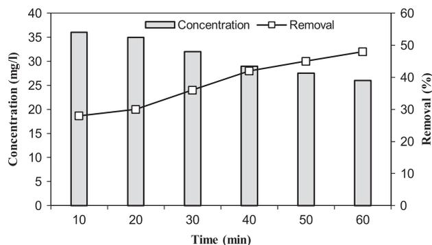
Fig. 5. Effect of ZnO catalyst, UV-C radiation, and ultrasonic wave process on formaldehyde degradation (formaldehyde concentration: 50 mg/l, ZnO dosage: 20 mg/l, and neutral pH of the solution).
