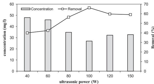
Fig. 10. Effect of ultrasonic wave power on sonophotocatalytic process (formaldehyde concentration: 80 mg/l, ZnO dosage: 60 mg/l, pH of the solution: 8, and contact time: 30 min).
