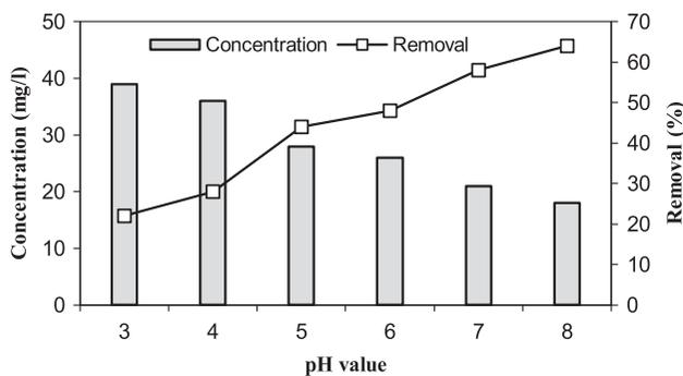
Fig. 7. Effect of pH of the solution on formaldehyde removal efficiency by sonophotocatalytic process (formaldehyde concentration: 50 mg/l, ZnO dosage: 20 mg/l, and contact time: 30 min).
