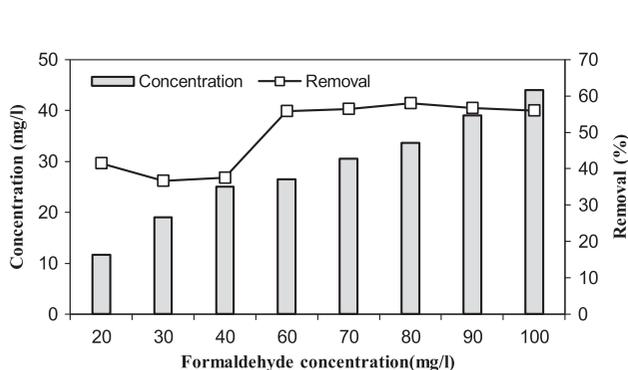
Fig. 9. Effect of initial concentration of formaldehyde on sonophotocatalytic process (ZnO dosage: 60 mg/l, pH of the solution: 8, and contact time: 30 min).
