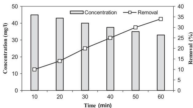
Fig. 4. Effect of ultrasonic wave on formaldehyde degradation (formaldehyde concentration: 50 mg/l and neutral pH of the solution).
