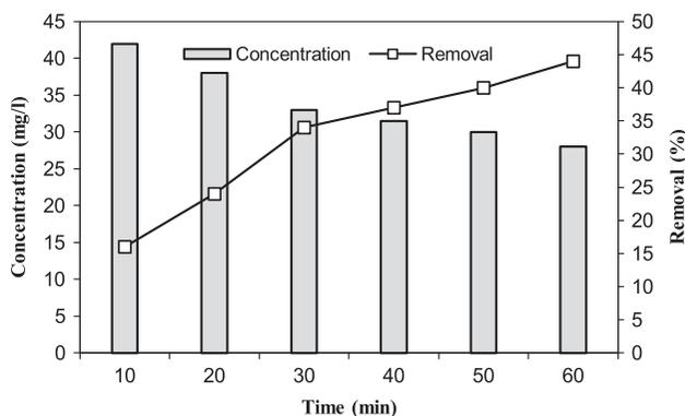
Fig. 3. Effect of ZnO nanoparticle on formaldehyde degradation (formaldehyde concentration: 50 mg/l, ZnO dosage: 20 mg/l, and neutral pH of the solution).
