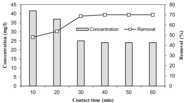
Fig. 11. Effect of contact time on formaldehyde removal efficiency by sonophotocatalytic process ( $\text{CH}_2\text{O}$  concentration: 80 mg/l, ZnO dosage: 60 mg/l, pH of the solution: 8, and ultrasonic intensity: 100 W).
