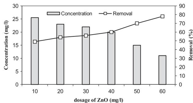
Fig. 8. Effect of ZnO dosage on formaldehyde removal efficiency by sonophotocatalytic process (formaldehyde concentration: 50 mg/l, pH of the solution: 8, and contact time: 30 min).
