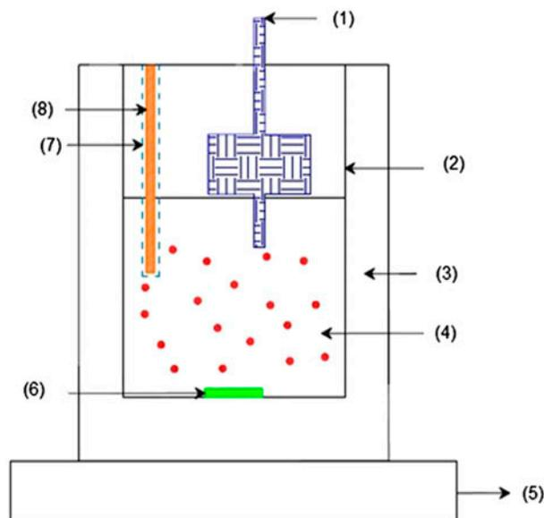
Fig. 1. Schematic diagram of sonophotocatalytic reactor (1—transcendent, 2—sonophotocatalytic reactor, 3—cooling water chamber, 4—sample content nZnO, 5—stirrer, 6—magnet, 7—quartz pipe, and 8—UV lamp).
