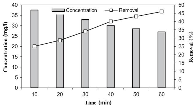
Fig. 2. Effect of UV-C radiation on formaldehyde degradation (formaldehyde concentration: 50 mg/l and neutral pH of the solution).
