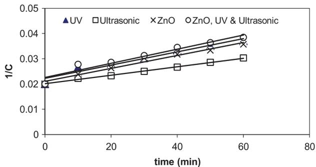
Fig. 6. Kinetic variances of UV-C photolysis, nZnO catalyst, ultrasonic, and enhanced nanophotocatalyst with ultrasonic wave (sonophotocatalytic process).
