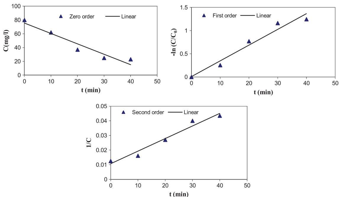
Fig. 12. Kinetic variances of photolysis, nZnO catalyst, ultrasonic wave, and sonophotocatalytic process.
