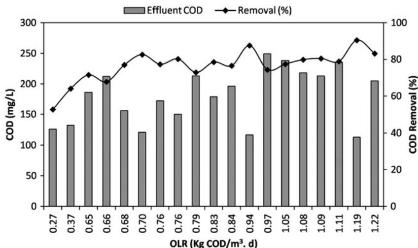
Fig. 3. Effects of OLR on COD removal.
