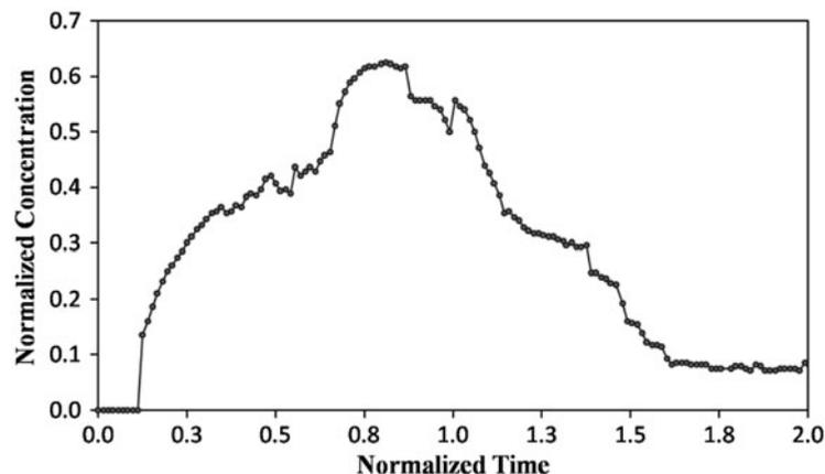
Fig. 5. Normalized RTD curves for the packaged system.
