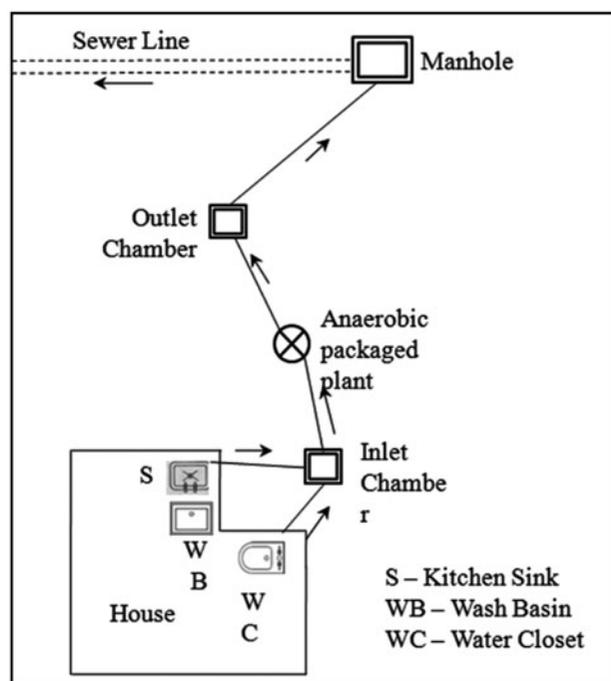
Fig. 1. Typical layout and flow scheme of the single household packaged system.
