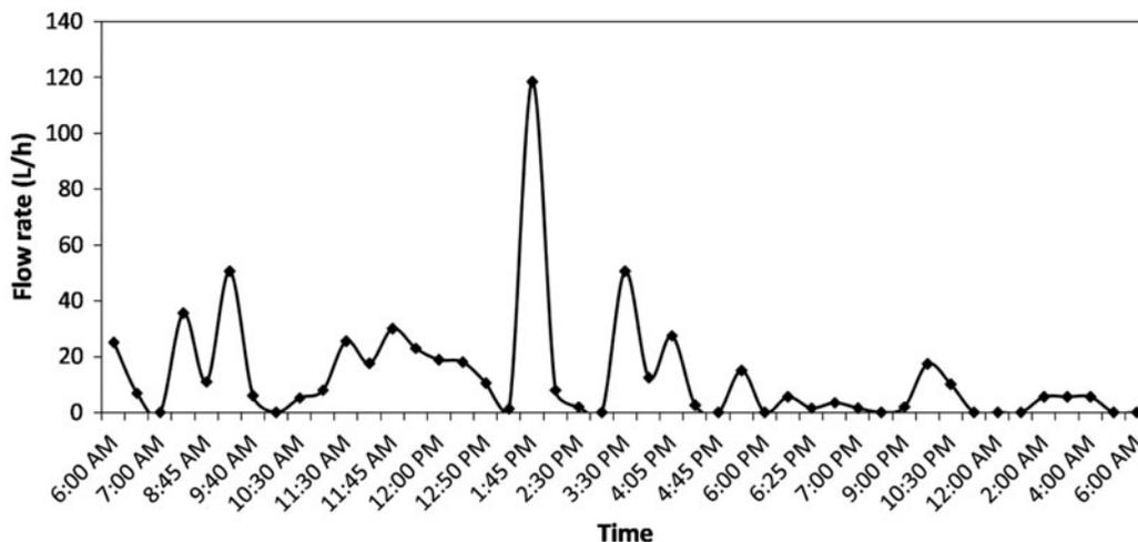
Fig. 2. Hourly fluctuations in the generated domestic wastewater.
