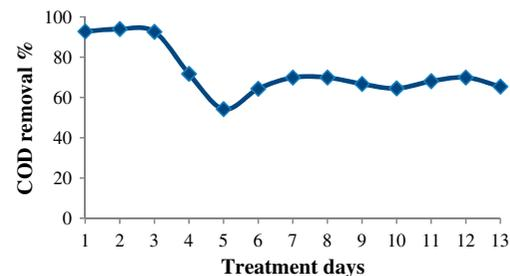
Fig. 2. COD removal efficiency during adaptation period.
