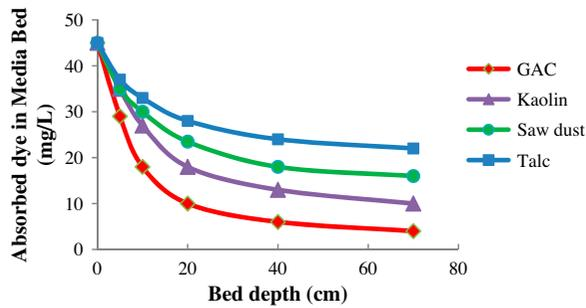
Fig. 4. Adsorbed dye vs. different bed depths.
