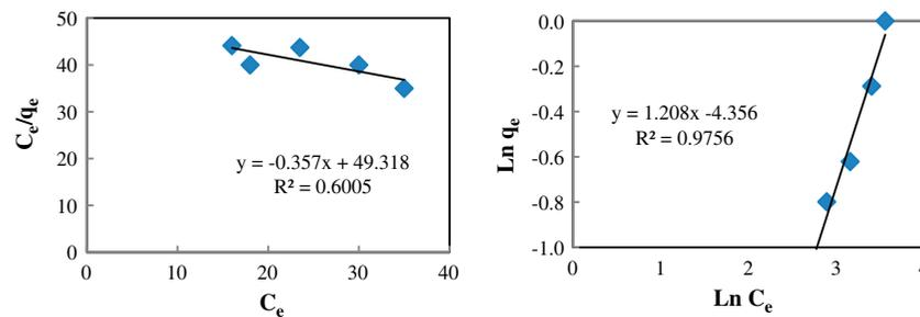
Fig. 8. Langmuir and Freundlich adsorption isotherms for saw dust.
