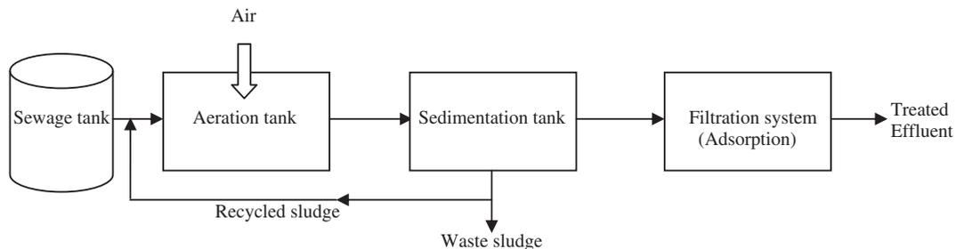
Fig. 1. The schematic layout of the experimental setup.
