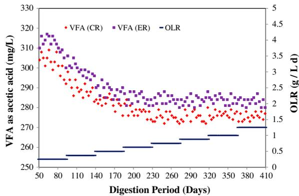
Fig. 4. Variation of VFA in the anaerobic reactors during the study period.
