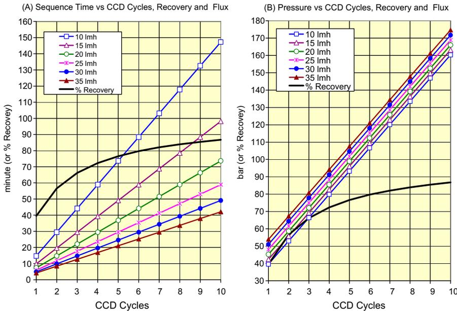
Fig. 4.1. Sequential variations of time (A) and pressure (B) as function CCD cycles, recovery, and flux for the SWRO-CCD ME2 (E = SWC6-MAX) unit according to the database in Table 4 for the flux range 10–35 Lmh.
