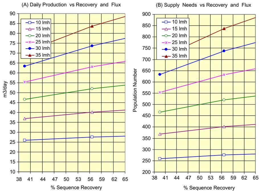
Fig. 4.3. Sequential variations of daily permeates production (A) and community size supply needs (B) as function of recovery and flux for the SWRO-CCD ME3 (E = SWC6-MAX) unit according to the database in Table 4 for the flux range 10–35 Lmh.
