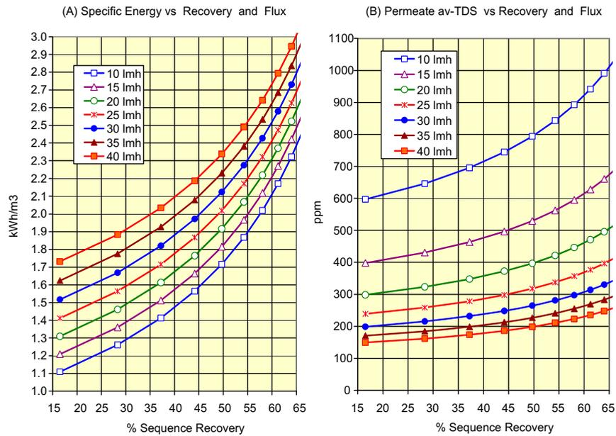
Fig. 2.2. Sequential variations of specific energy (A) and TDS of permeates (B) as function of recovery and flux for the SWRO-CCD ME (E = SWC6-MAX) unit according to the database in Table 2 for the flux range 10–40 Lmh.
