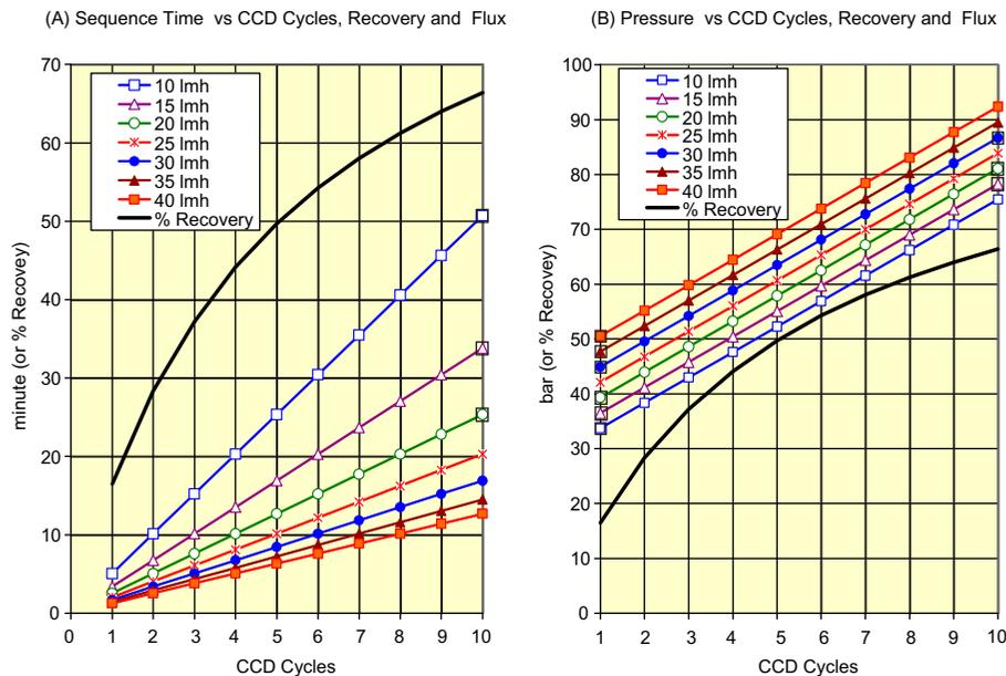
Fig. 2.1. Sequential variations of time (A) and pressure (B) as function CCD cycles, recovery, and flux for the SWRO-CCD ME (E = SWC6-MAX) unit according to the database in Table 2 for the flux range 10–40 Lmh.
