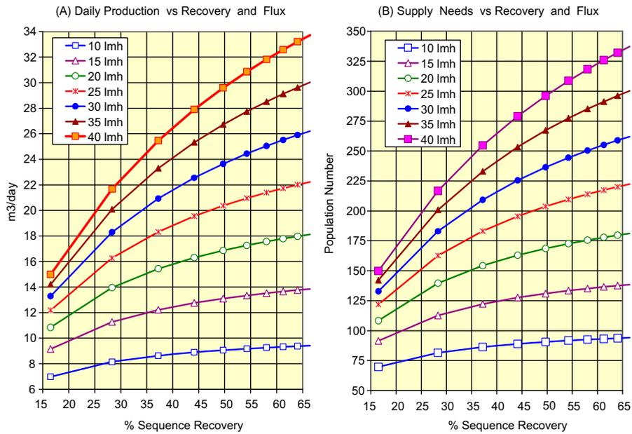
Fig. 2.3. Sequential variations of daily permeates production (A) and community size supply needs (B) as function of recovery and flux for the SWRO-CCD ME (E = SWC6-MAX) unit according to the database in Table 2 for the flux range 10–40 Lmh.
