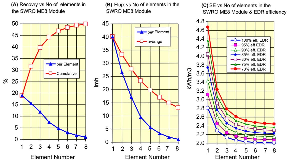
Fig. 1. Recovery (A), flux (B), and specific energy (C) variations as function of number of elements per conventional ME $n$  ( $n = 1-8$ ; E = SWC6-MAX) module according to Table 1.
