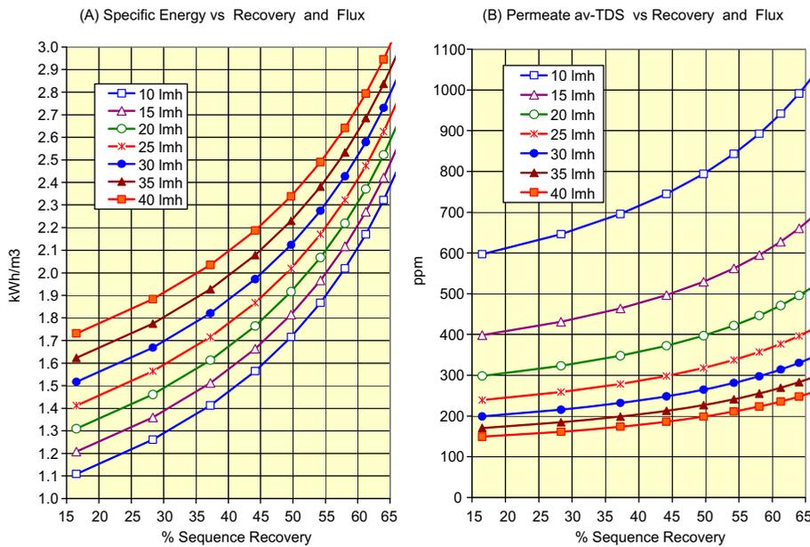
Fig. 3.2. Sequential variations of specific energy (A) and TDS of permeates (B) as function of recovery and flux for the SWRO-CCD ME2 (E = SWC6-MAX) unit according to the database in Table 3 for the flux range 10–40 Lmh.
