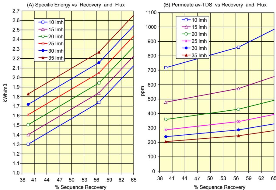
Fig. 4.2. Sequential variations of specific energy (A) and TDS of permeates (B) as function of recovery and flux for the SWRO-CCD ME3 (E = SWC6-MAX) unit according to the database in Table 4 for the flux range 10–35 Lmh.
