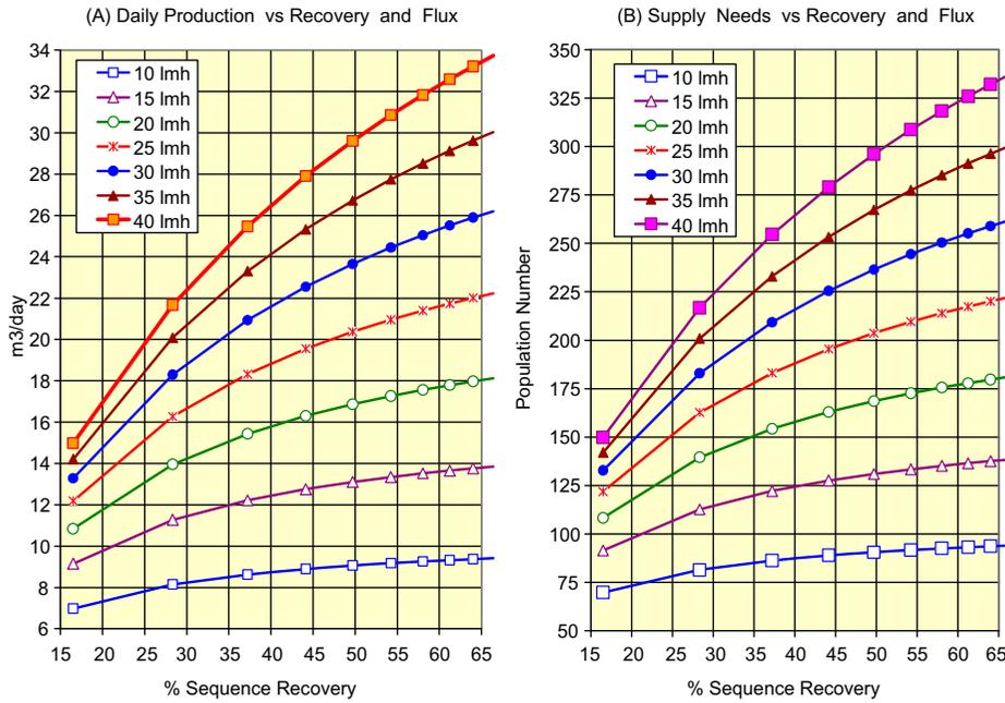
Fig. 3.3. Sequential variations of daily permeates production (A) and community size supply needs (B) as function of recovery and flux for the SWRO-CCD ME2 (E = SWC6-MAX) unit according to the database in Table 3 for the flux range 10–40 Lmh.
