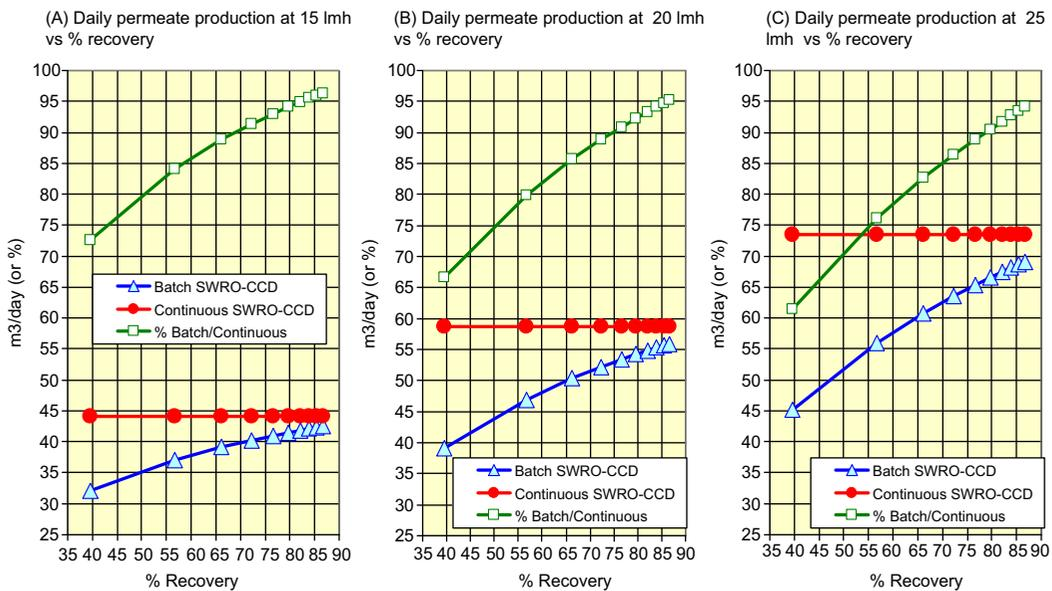
Fig. 5. Daily permeate production of continuous and batch ME3 (E = SWC6-MAX) units at flux of 15, 20, and 25 Lmh on the recovery scale according to the database in Table 4 with the cited flux.
