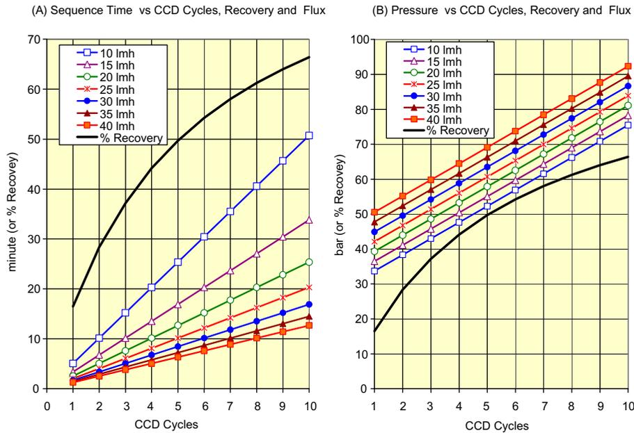
Fig. 3.1. Sequential variations of time (A) and pressure (B) as function of CCD cycles, recovery, and flux for the SWRO-CCD ME2 (E = SWC6-MAX) unit according to the database in Table 3 for the flux range 10–40 Lmh.
