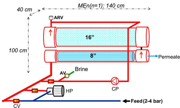
Fig. 2. SWRO-CCD ME batch unit design comprising a single element 8'' module connected in line to an empty 16'' PV of 175 L total closed circuit volume, one circulation pump with vfd (CP), one positive displacement pump for high pressure with vfd (HP), three one-way CV, one AV, and an ARV—red lines stands for pressurized sections and blue for none pressurized lines.
