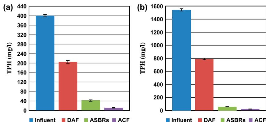
Fig. 3. Elimination of TPH content at different crude oil concentrations of (a)  $412 \pm 3 \text{ mg l}^{-1}$  and (b)  $1,590 \pm 10 \text{ mg l}^{-1}$ .
