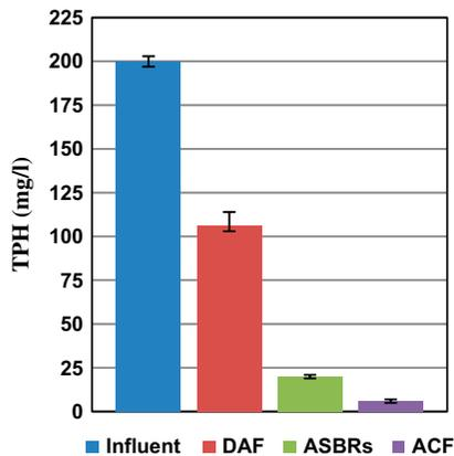
Fig. 2. The removal of TPH using pilot stages at optimum values of HRT and RAS rate of the ASBRs.
