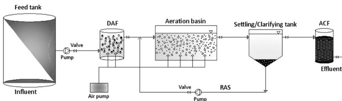
Fig. 1. Schematic diagram of pilot stages: Feed tank; DAF; ASBRs including aeration basin and settling/clarifying compartments; ACF.
