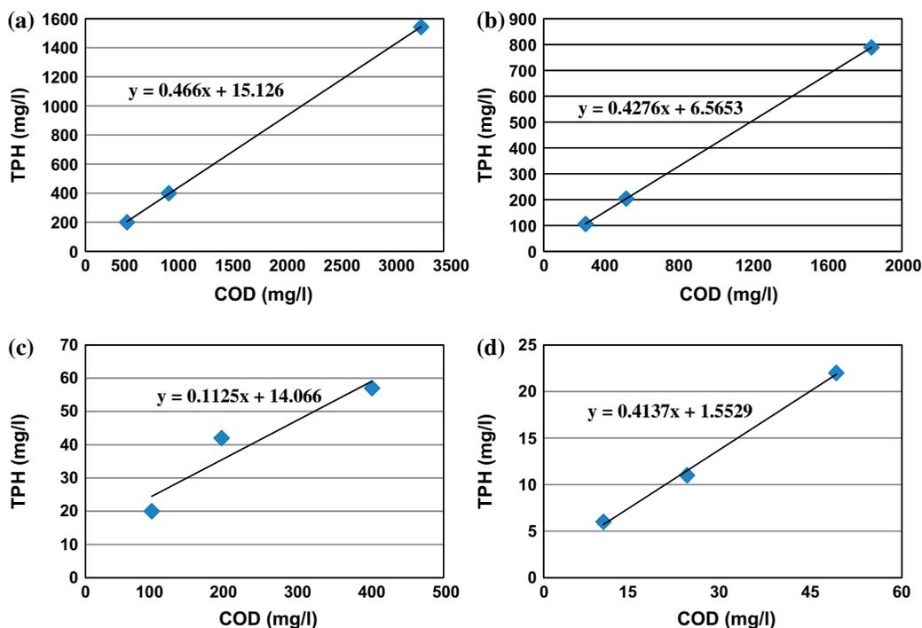
Fig. 5. The correlation between TPH and COD in all process steps.
