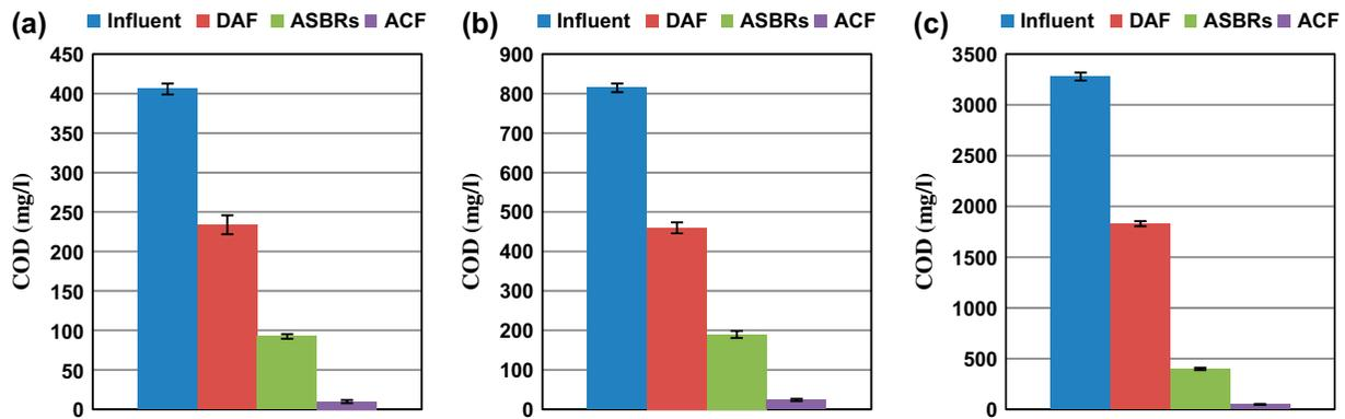
Fig. 4. The COD reduction through remediation steps at initial oil feeding of (a)  $206 \pm 1 \text{ mg l}^{-1}$ , (b)  $412 \pm 3 \text{ mg l}^{-1}$ , and (c)  $1,590 \pm 10 \text{ mg l}^{-1}$ .
