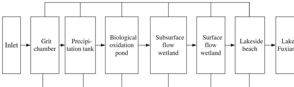
Fig. 2. The process flow diagram of the riparian wetland (Phase I).
