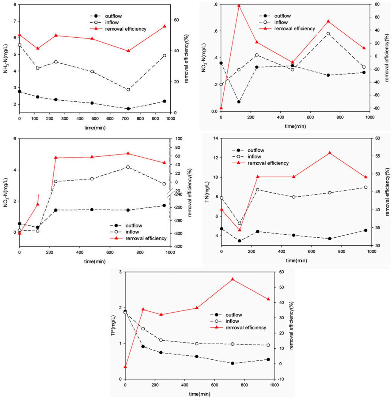
Fig. 4. Different water quality parameters in Yaonigou wetland (Phase II) under stormwater events.
