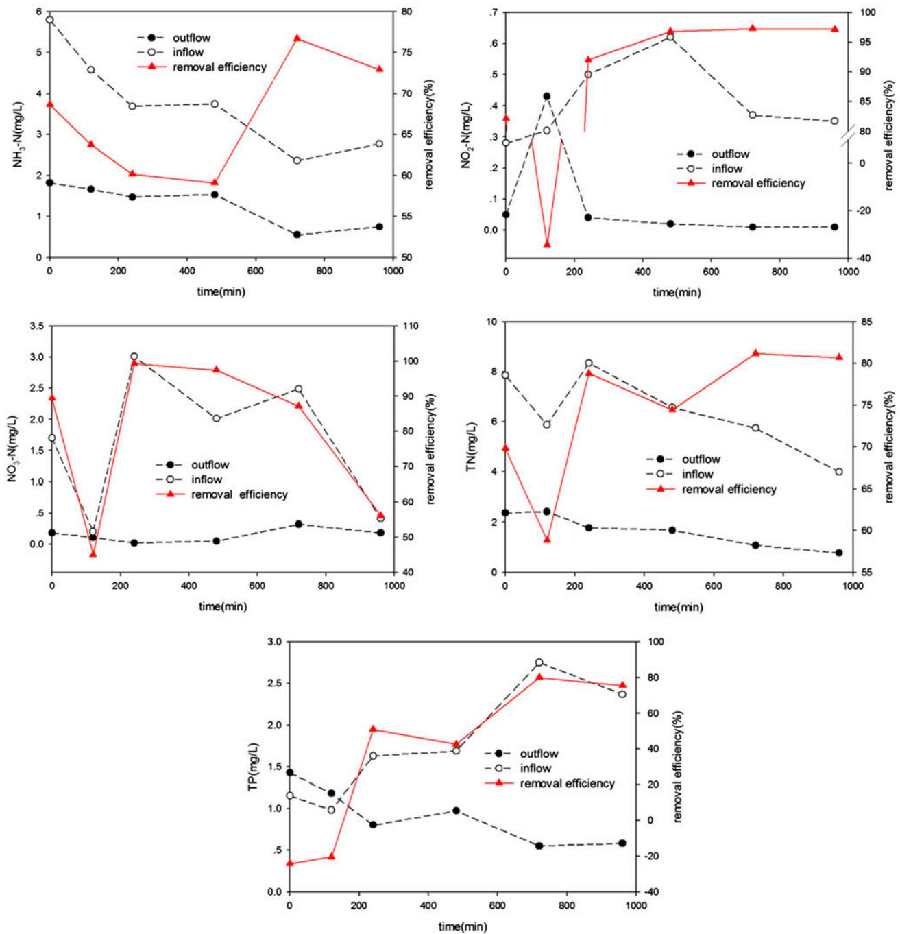
Fig. 3. Different water quality parameters in Yaonigou wetland (Phase I) for the stormwater events.
