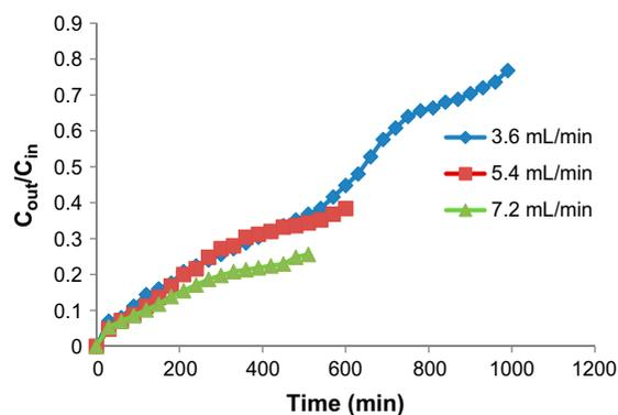
Fig. 2. Breakthrough curve for flow rate in continuous mode study.
