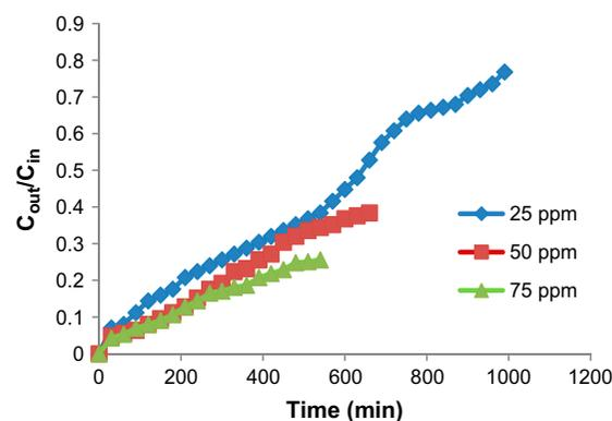
Fig. 3. Breakthrough curve for initial dye concentration in continuous mode study.
