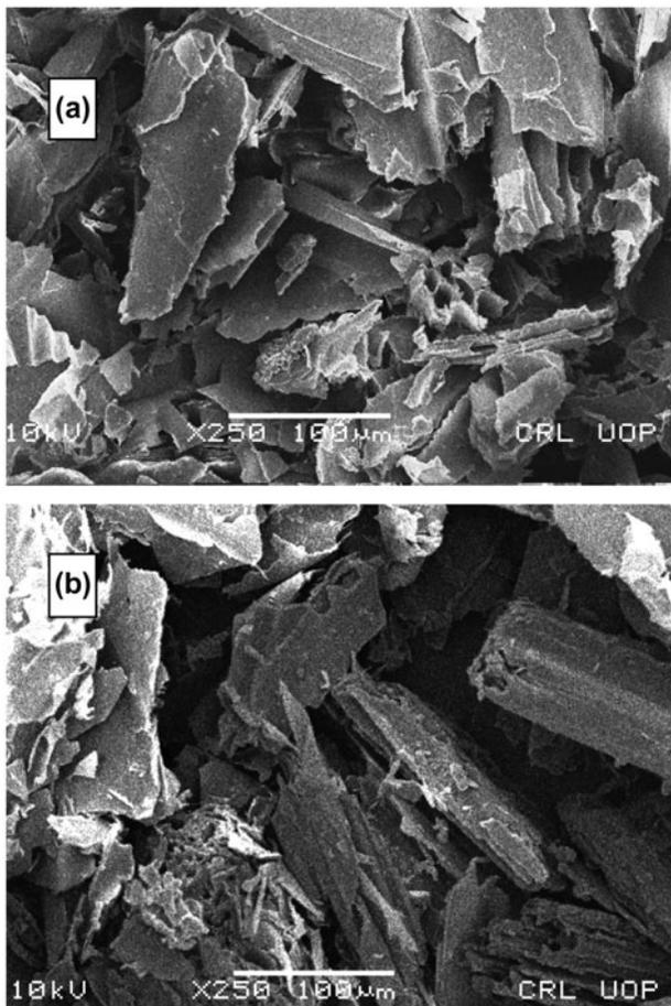
Fig. 4. SEM analysis of (a) native biomass and (b) dye-loaded biomass.
