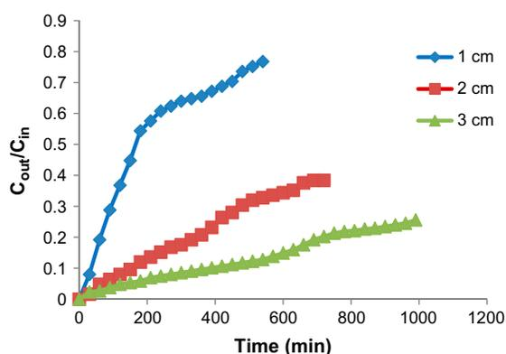
Fig. 1. Breakthrough curve for bed height in continuous mode study.
