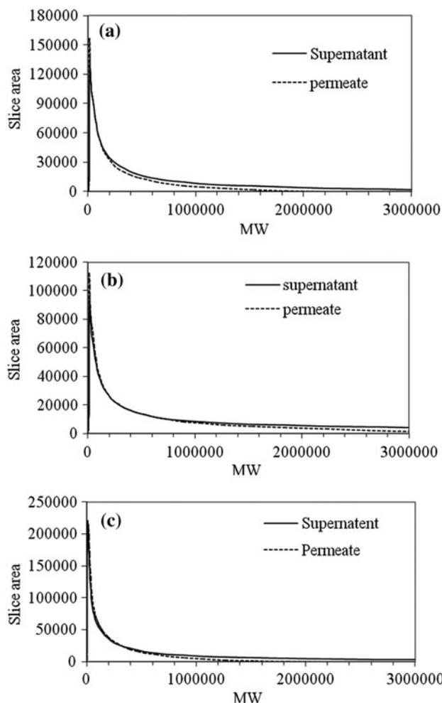
Fig. 8. MW distribution of supernatants and corresponding permeate samples in MBRs. (a) Control MBR; (b) CGMS-added MBR; (c) MGMS-added MBR.
