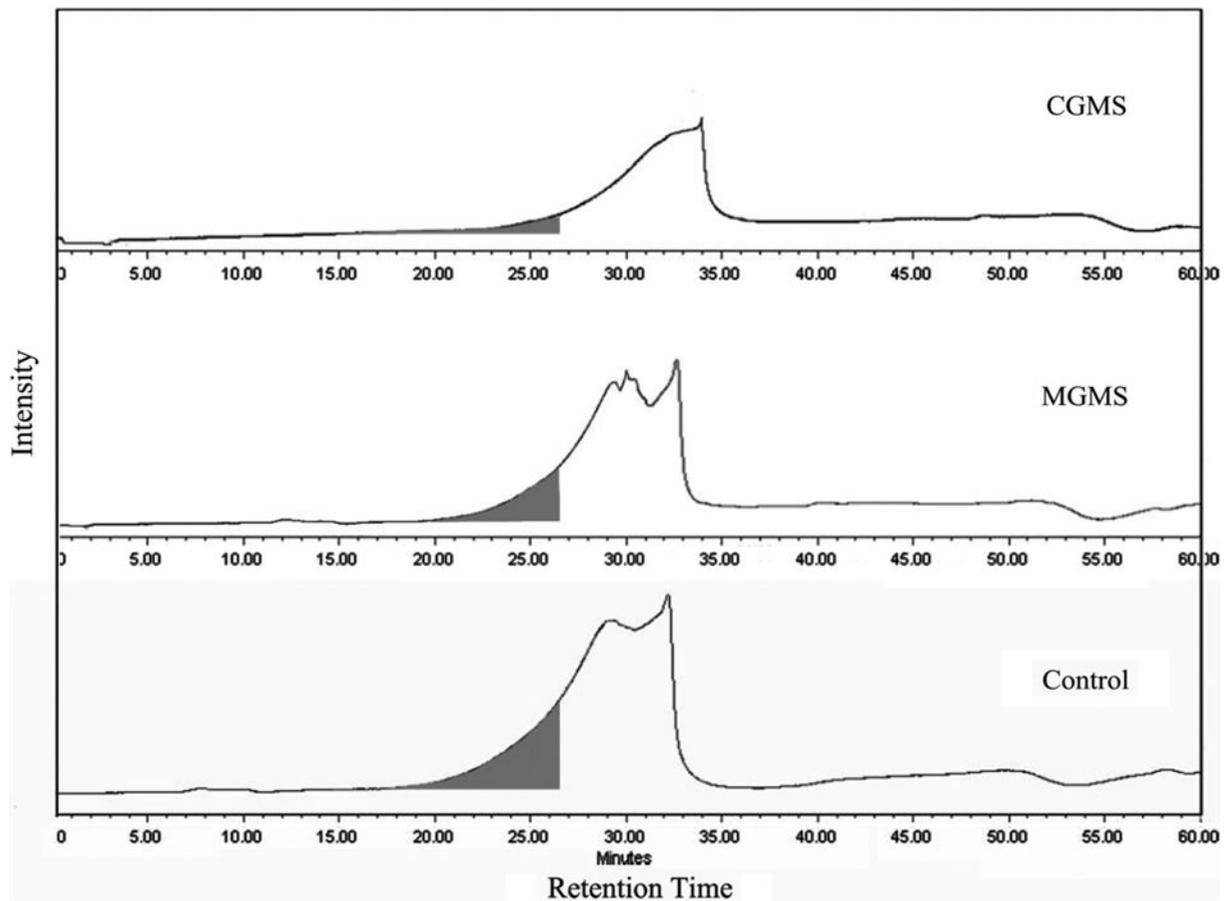
Fig. 6. GPC spectra of the MBR supernatants under a constant flux of 20 L/m<sup>2</sup> h (retention time from 0 to 26.6 min corresponds to MW ≥ 100 kDa).
