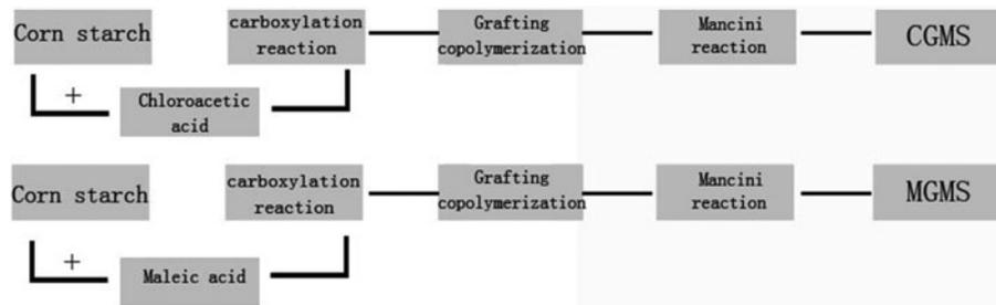
Fig. 2. Preparation process of the two modified starches.
