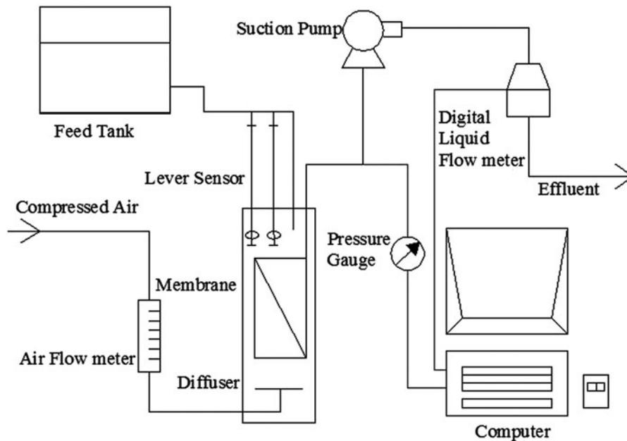
Fig. 1. Schematic diagram of the submerged membrane bioreactor.
