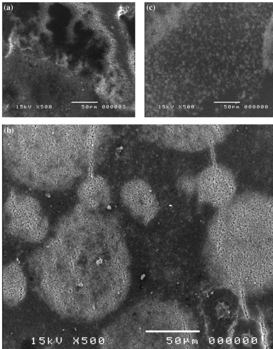
Fig. 4. SEM image of the surface of the fouled membrane from the control MBR. (a) Control MBR; (b) CGMS-added MBR; (c) MGMS-added MBR.
