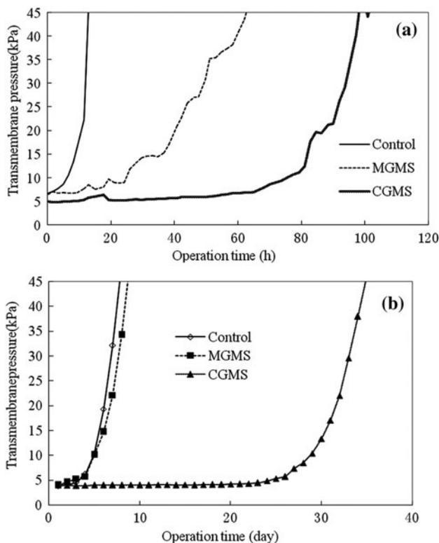
Fig. 3. (a) TMP profiles of different MBR systems at 40 L/m<sup>2</sup> h. (b) TMP profiles of different MBR systems at 20 L/m<sup>2</sup> h (filter aids added before filtration).
