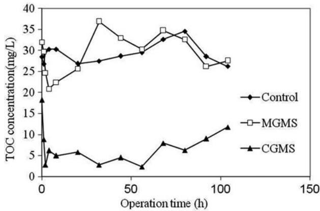
Fig. 5. TOC profiles in one filtration cycle (under a constant flux of 40 L/m<sup>2</sup> h).
