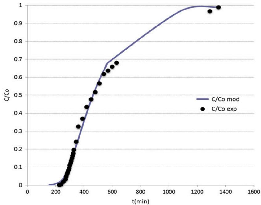
Fig. 12.  $Cr^{3+}$  experimental and model curves for vermiculite.
