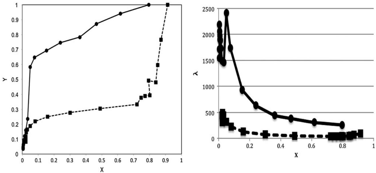
Fig. 5.  $Cr^{2+}$  equilibrium curves (left) and distribution coefficients (right). Clinoptilolite is marked with dashed line and square points and vermiculite in solid line and cyclic points.
