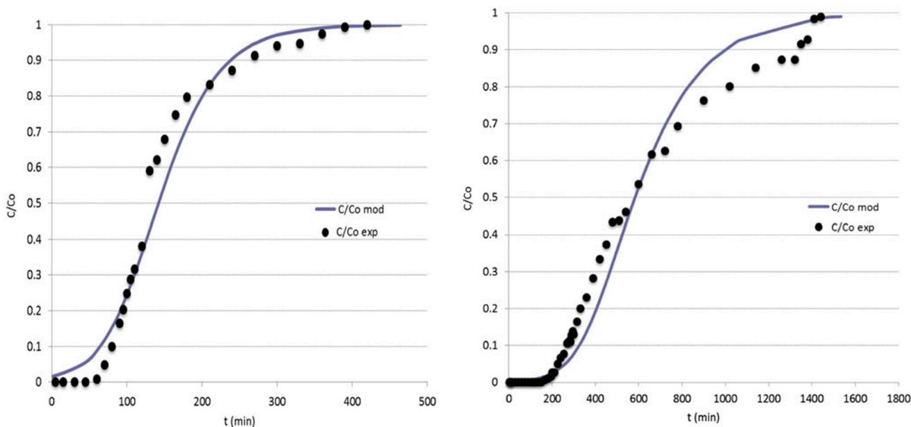
Fig. 10.  $Zn^{2+}$  experimental and model curves for clinoptilolite (left) and vermiculite (right).
