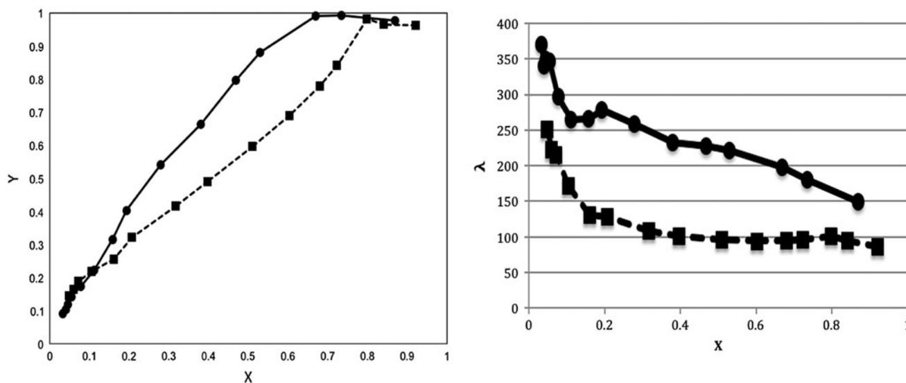
Fig. 3. Zn<sup>2+</sup> equilibrium curves (left) and distribution coefficients (right). Clinoptilolite is marked with dashed line and square points and vermiculite in solid line and cyclic points.
