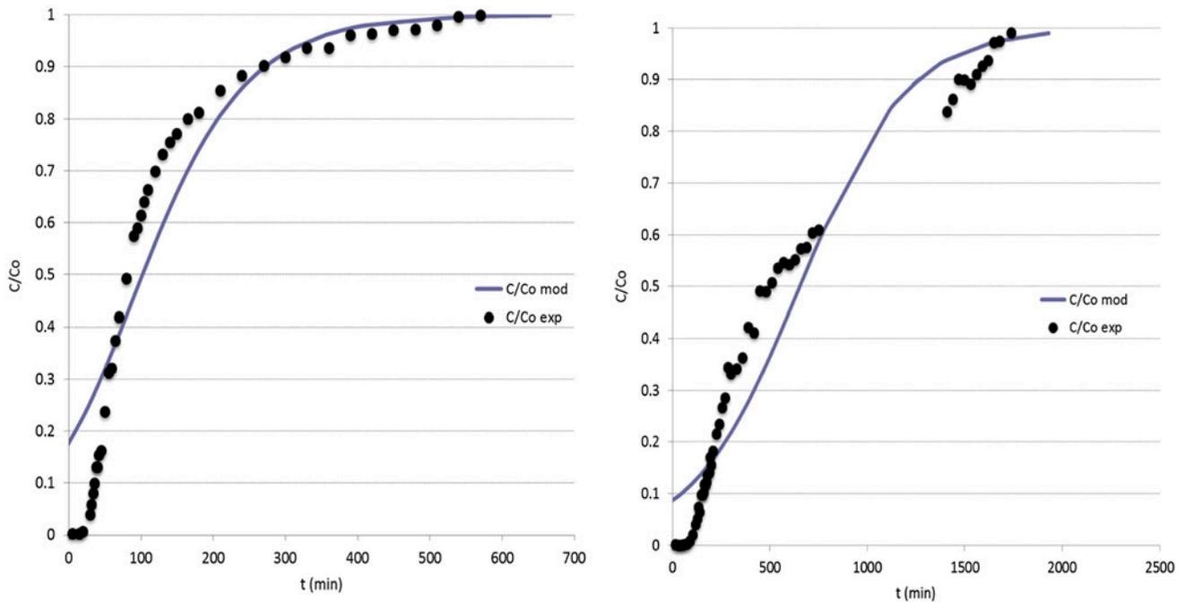
Fig. 11.  $Mn^{2+}$  experimental and model curves for clinoptilolite (left) and vermiculite (right).
