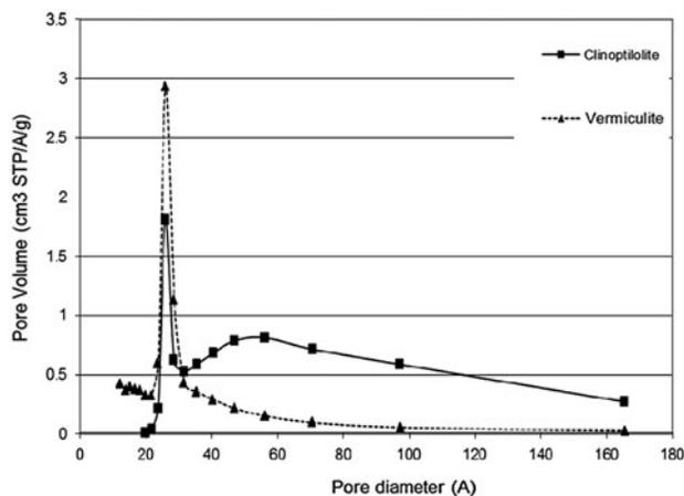
Fig. 1. Pore size distribution of clinoptilolite and vermiculite (BET analysis).
