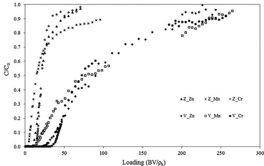
Fig. 9. Breakthrough curves for clinoptilolite (Z) and vermiculite (V).
