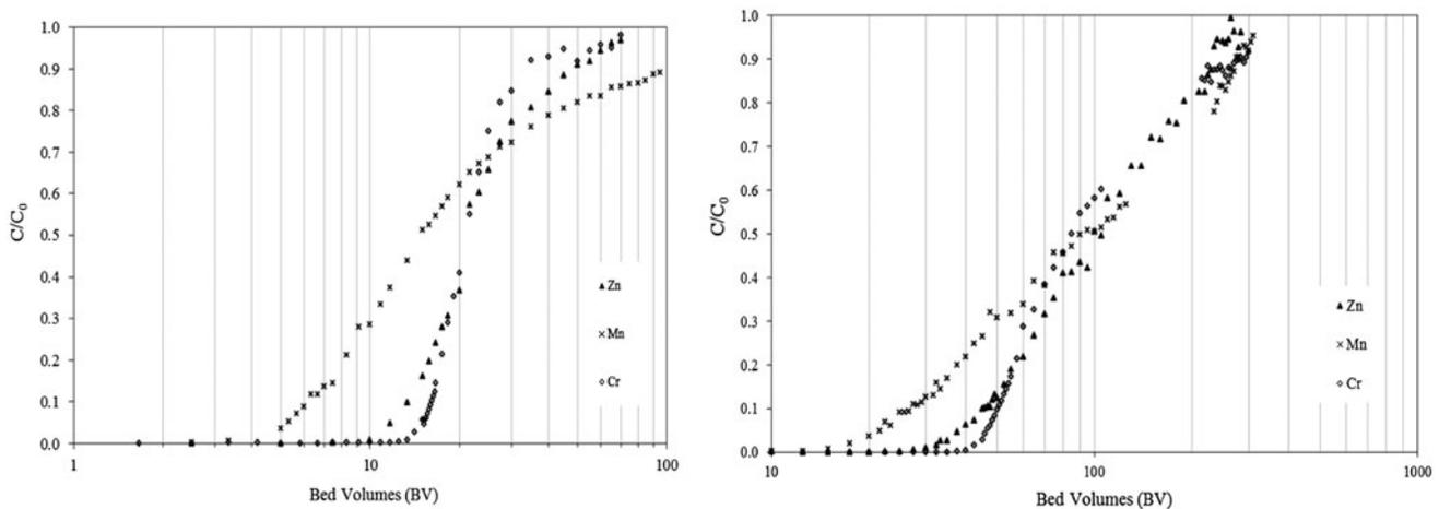
Fig. 8. Breakthrough curves for clinoptilolite (left) and vermiculite (right).
