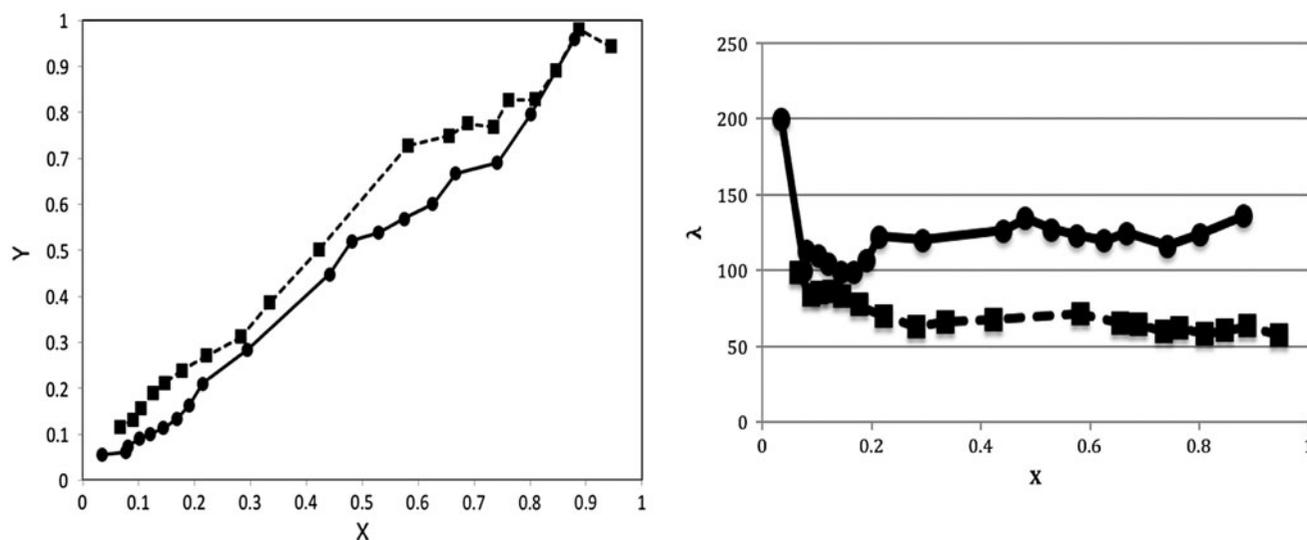
Fig. 4. Mn<sup>2+</sup> equilibrium curves (left) and distribution coefficients (right). Clinoptilolite is marked with dashed line and square points and vermiculite in solid line and cyclic points.
