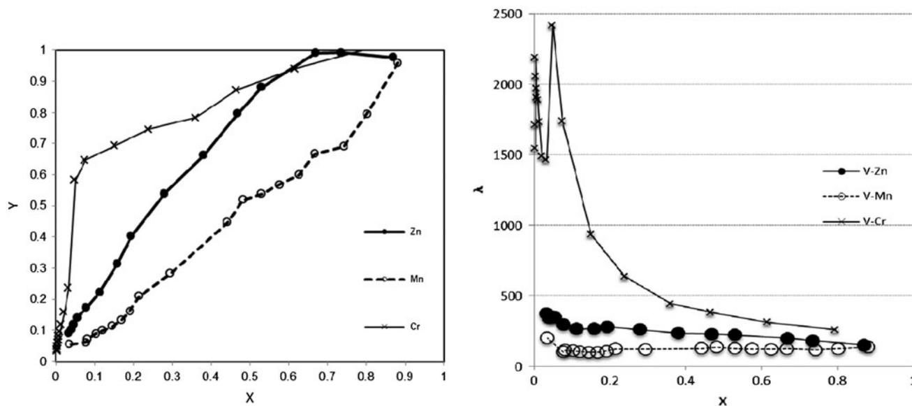
Fig. 7. Vermiculite equilibrium curves (left) and distribution coefficients (right).
