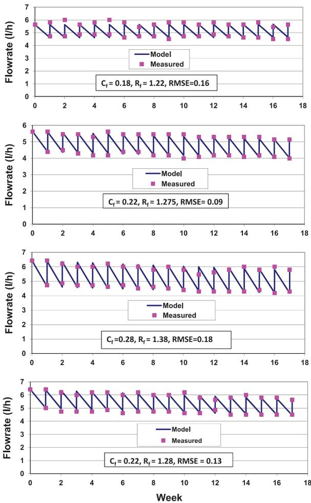
Fig. 2. Comparisons of model results with measured data for “Site 1.”
