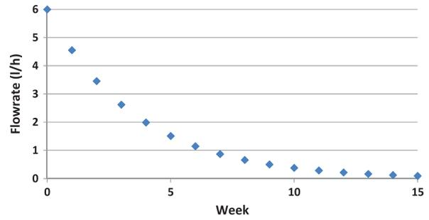
Fig. 6. Continuous decline of flow capacity for a filter without cleaning with  $C_f = 0.24$ .
