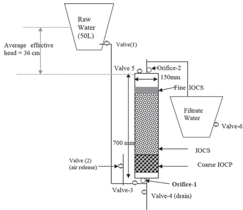
Fig. 1. Photo and schematic diagram of IHE family filter.
