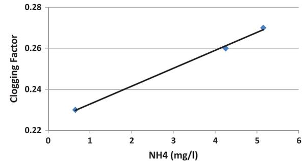
Fig. 8. Relationship of clogging factor with influent ammonium concentration.
