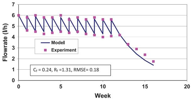
Fig. 5. Comparison of model results with measurements for a filter not cleaned after week 11.
