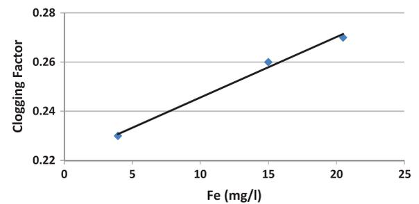
Fig. 7. Relationship of clogging factor with influent iron concentration.
