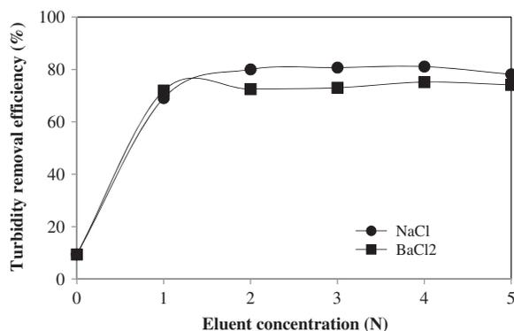
Fig. 3c. Effect of eluent concentration on turbidity removal efficiency.
