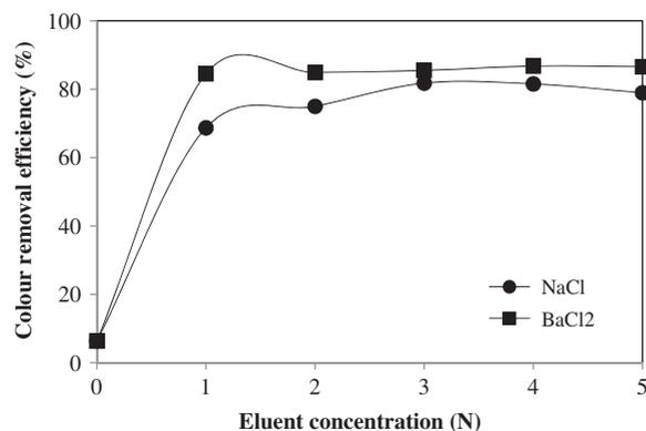
Fig. 3a. Effect of eluent concentration on color removal efficiency.
