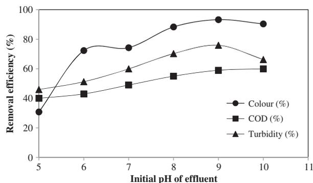
Fig. 6. Effect of initial pH of effluent on removal efficiency. Note: pH = 5–11; coagulant: extragens = 3 g of crab shell powder: 100 mL of 3 N NaCl; coagulant volume = 100 mL; sample number 1.
