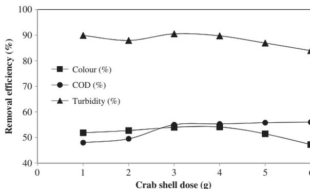
Fig. 4. Effect of coagulant dose on removal efficiency.
