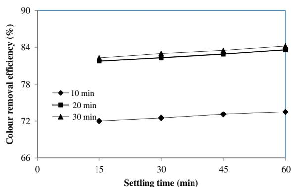
Fig. 2a. Effect of time on color removal efficiency. Note: pH = actual effluent pH (7.2–7.8); coagulant: extragens = 5 g of crab shell powder: 100 mL of 3 N NaCl; coagulant volume = 100 mL; sample number 1.
