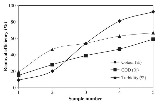
Fig. 7. Effect of initial concentration of effluent on removal efficiency. Note: pH = actual effluent pH (7.2–7.8); coagulant: extragens = 3 g of crab shell powder: 100 mL of 3 N NaCl; coagulant volume = 100 mL; sample number 1–5.
