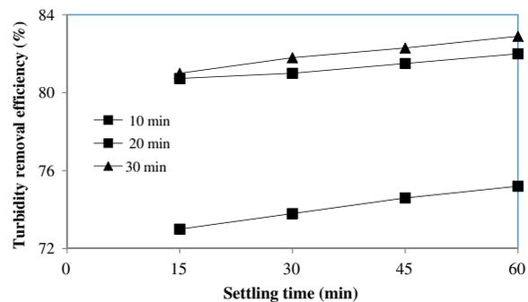
Fig. 2b. Effect of time on turbidity removal efficiency. Note: pH = actual effluent pH (7.2–7.8); coagulant: extragens = 5 g of crab shell powder: 100 mL of 3 N NaCl; coagulant volume = 100 mL; sample number 1.
