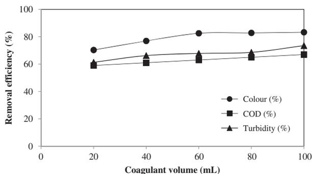
Fig. 5. Effect of coagulant volume on removal efficiency. Note: pH = actual effluent pH (7.2–7.8); coagulant: extragens = 3 g of crab shell powder: 100 mL of 3 N NaCl; coagulant volume = 20–100 mL; sample number 1.
