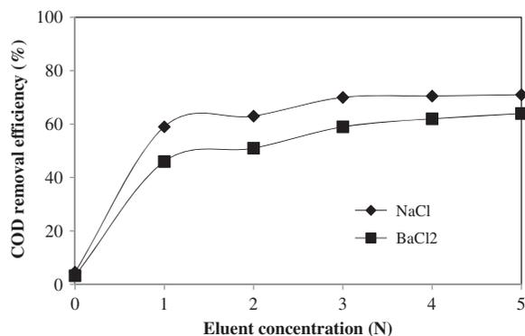
Fig. 3b. Effect of eluent concentration on COD removal efficiency.
