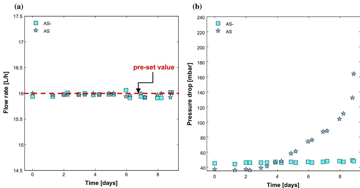
Fig. 4. Feedwater flow rate (a) and pressure drop in time (b) over the MFS systems with automatic flow control fed with water without (AS-) and with dosed (AS) biodegradable substrate.
