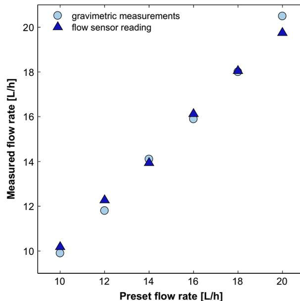
Fig. 3. Correlation between preset and measured flow rate of the developed automated system for the range 10–20 L h<sup>-1</sup>.
