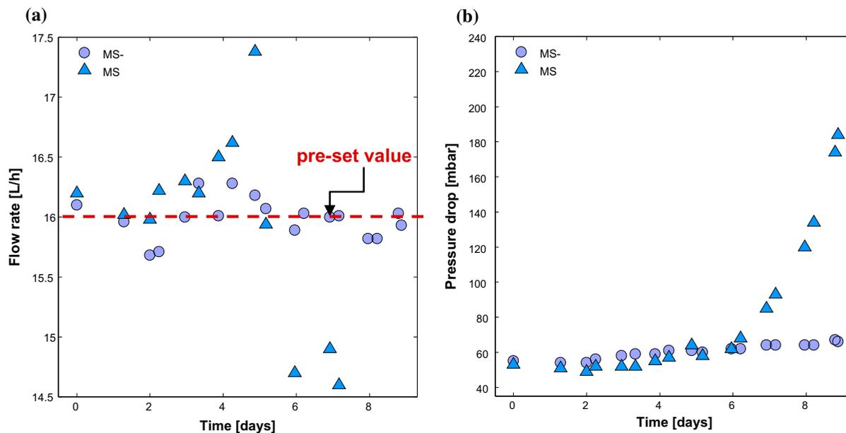
Fig. 2. Feedwater flow rate (a) and pressure drop in time (b) over the MFS systems with manual flow control and fed with water without (MS-) and with supplemented (MS) biodegradable substrate.
