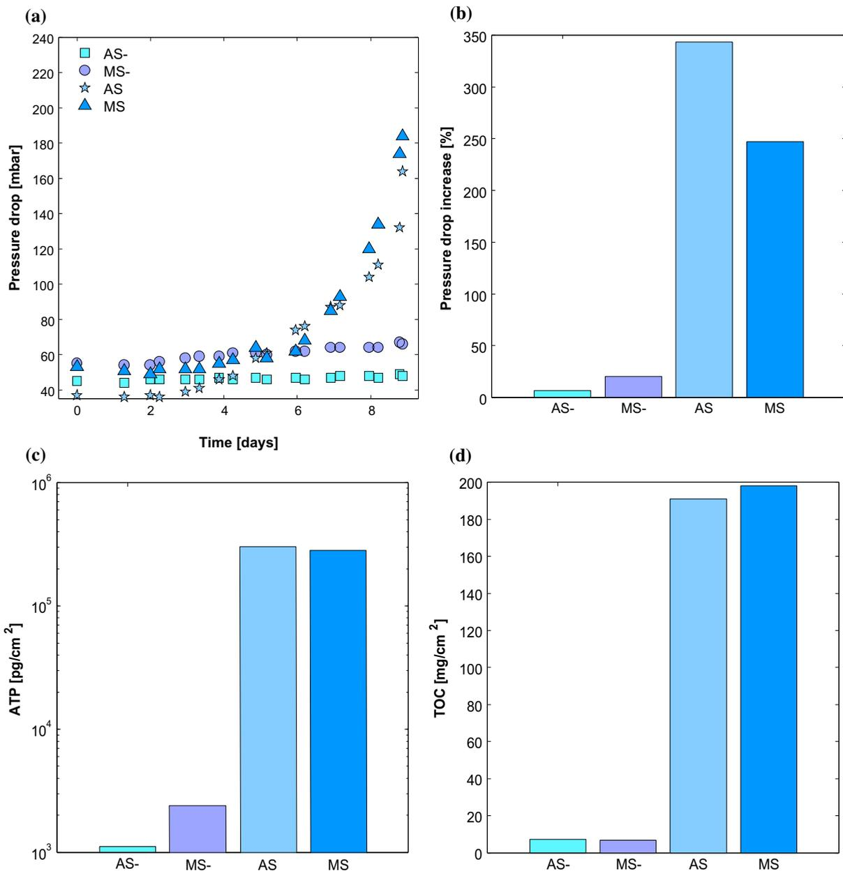
Fig. 5. Pressure drop in time (a) and pressure drop increase (b), and accumulated biomass in ATP and TOC (c,d) for manually and automatic controlled setups. Manual flow control without substrate (MS-) and with dosed substrate (MS). Automatic flow control without substrate (AS-) and with dosed substrate (AS). In all cases, the initial pressure drop was lower for the automatic setups.
