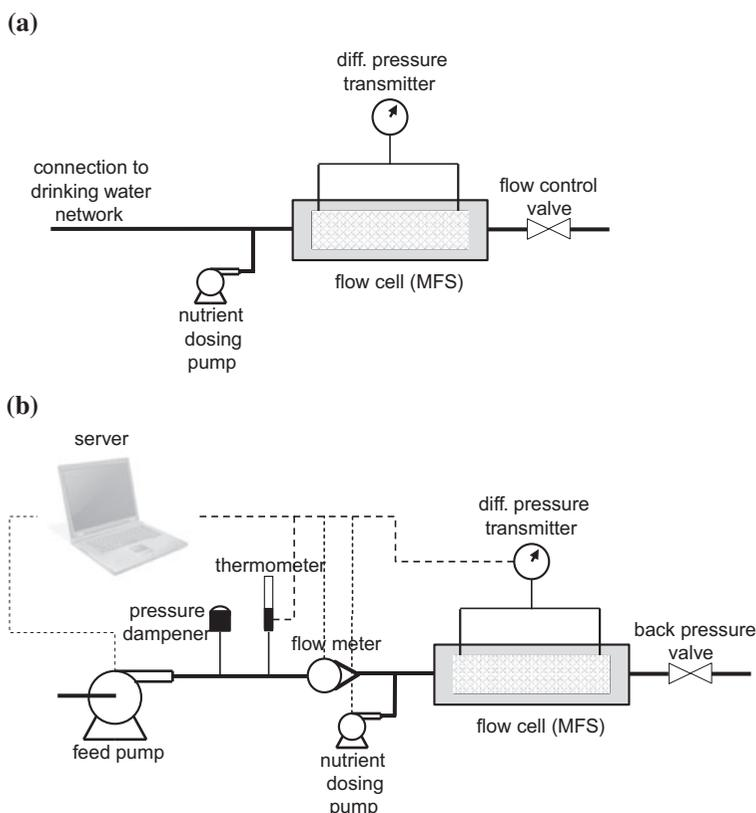
Fig. 1. Schematic representation of the system for MFS operation: (a) with manual flow control and the (b) developed setup with automatic flow control and data logging system.
