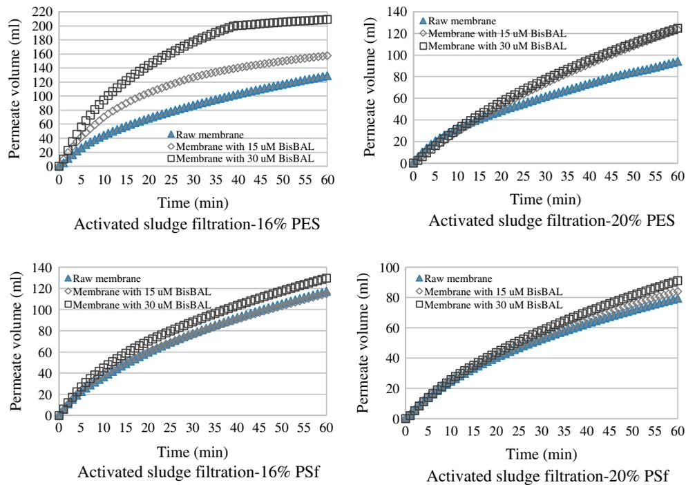
Fig. 3. Activated sludge filtration permeate profiles.
