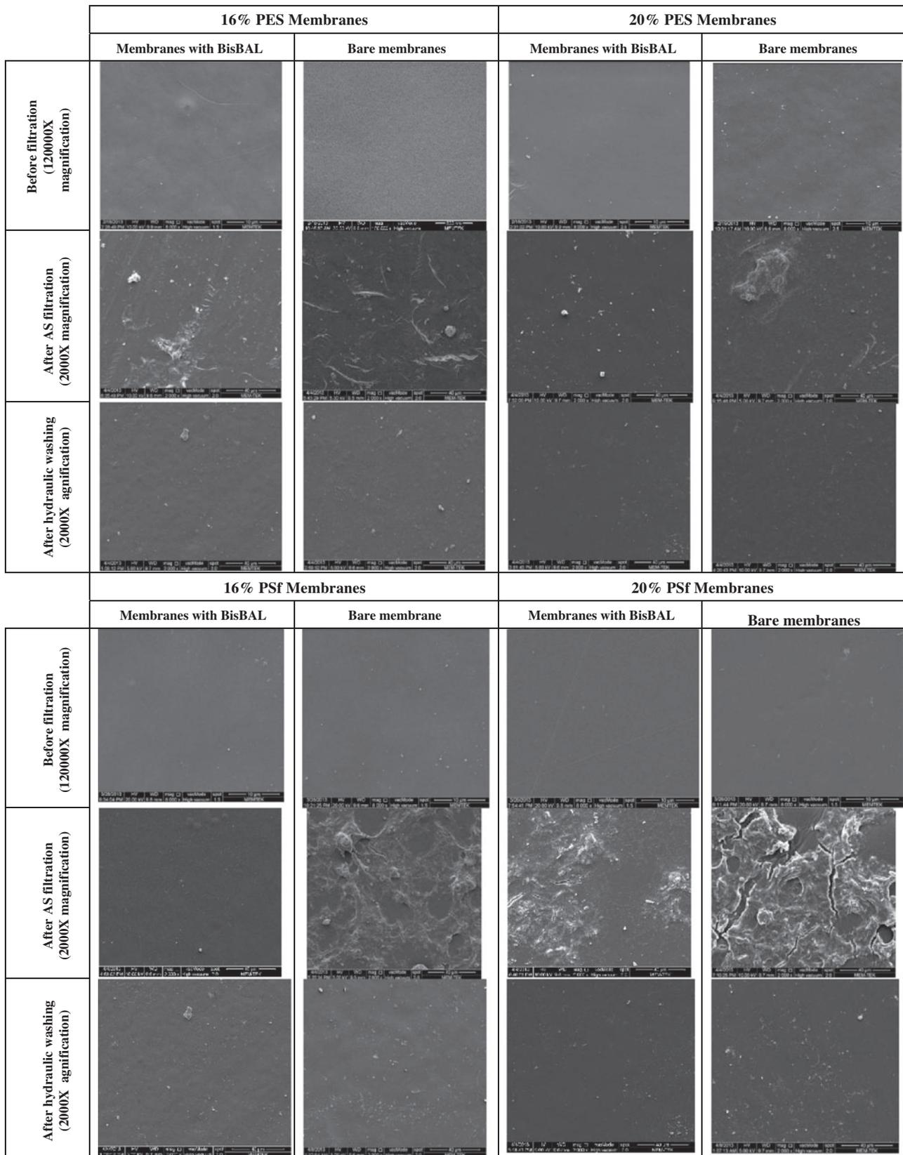
Fig. 4. SEM images of without BisBAL and produced antibiofouling membranes before filtration, after activated sludge filtration, and after hydraulic washing, following activated sludge filtration.
