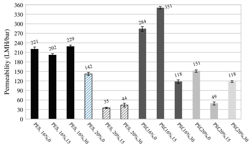
Fig. 1. Pure water permeability values of membranes (Ex.; PES, 16%, 0: nonmodified PES (16%) membrane Ex.; PSf, 20%, 30: modified PSf (20%) membrane with 30  $\mu$ M BisBAL).
