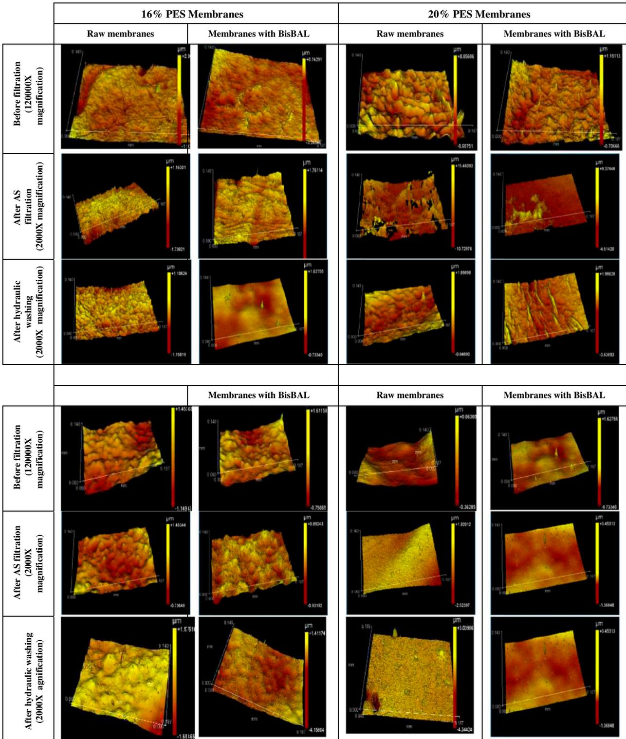
Fig. 5. Optic profilometer result images of without BisBAL and produced antibiofouling membranes before filtration, after activated sludge filtration, and after hydraulic washing, following activated sludge filtration.
