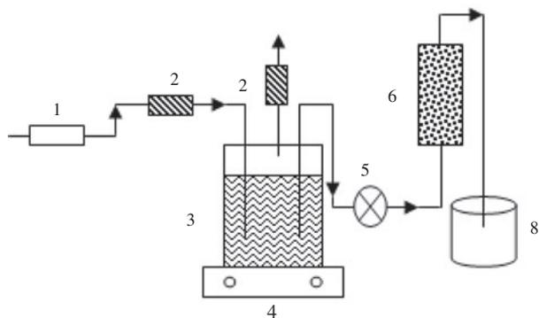
Fig. 1. Continuous system: (1) air pump; (2) air filters; (3) feed reservoir; (4) magnetic stirrer; (5) peristaltic pump; (6) column reactor; (7) sampling/effluent and (8) treated water collection.
