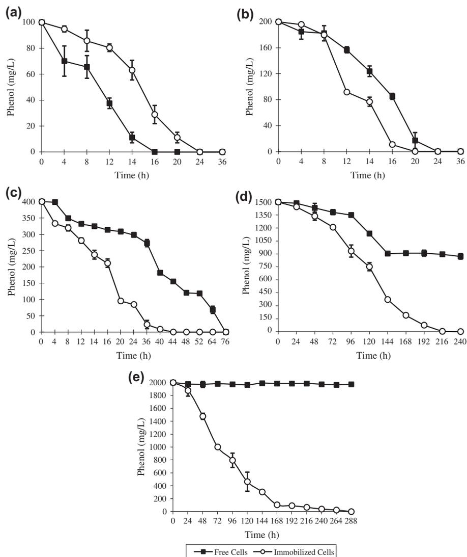
Fig. 6. The effects of phenol concentration (mg/L): (a) 100, (b) 200, (c) 400, (d) 1500 and (e) 2,000 on phenol removal by free and immobilized cells.
