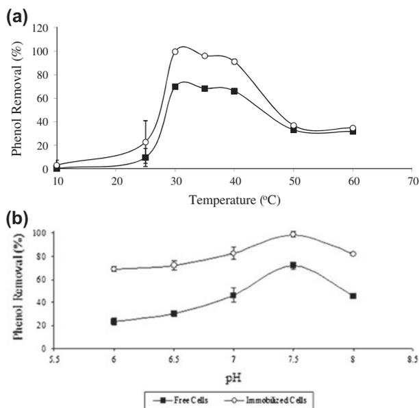
Fig. 5. The effect of (a) temperature at pH 7.5 and (b) pH at 30°C, on phenol removal.
