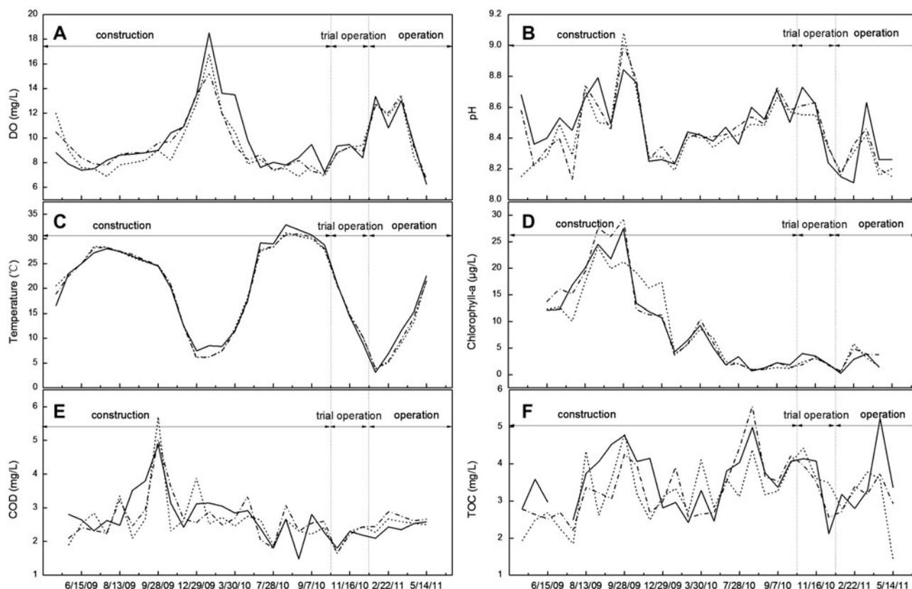
Fig. 2. Variation of DO (A), pH (B), temperature (C), Chla (D),  $COD_{Mn}$  (E), and TOC (F) in representative stations of the reservoir; solid line represents S2, dash dot represents S6, and short dash represents S9.
