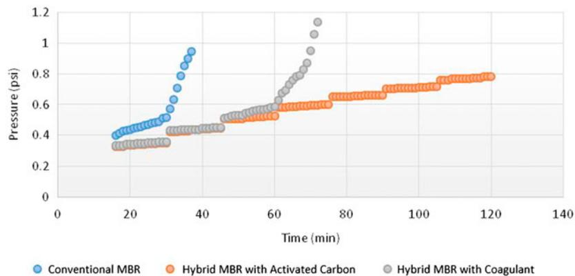
Fig. 4. Fouling control performance for conventional MBR, MBR-PAC, and MBR-coagulant.
