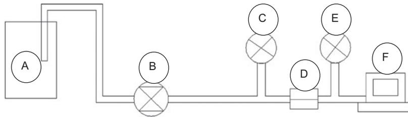
Fig. 2. Crossflow filtration system (A: Sludge tank; B: Water pump; C: Inlet pressure gauge; D: Membrane holder; E: Outlet pressure gauge; F: Computer).
