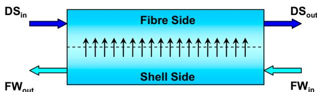
Fig. 2. DURASEP- FO-AC membrane configuration.
