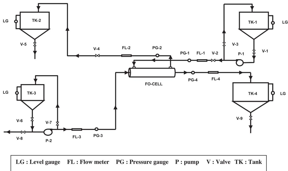
Fig. 1. Schematic diagram of forward osmosis pilot plant unit used in this study.
