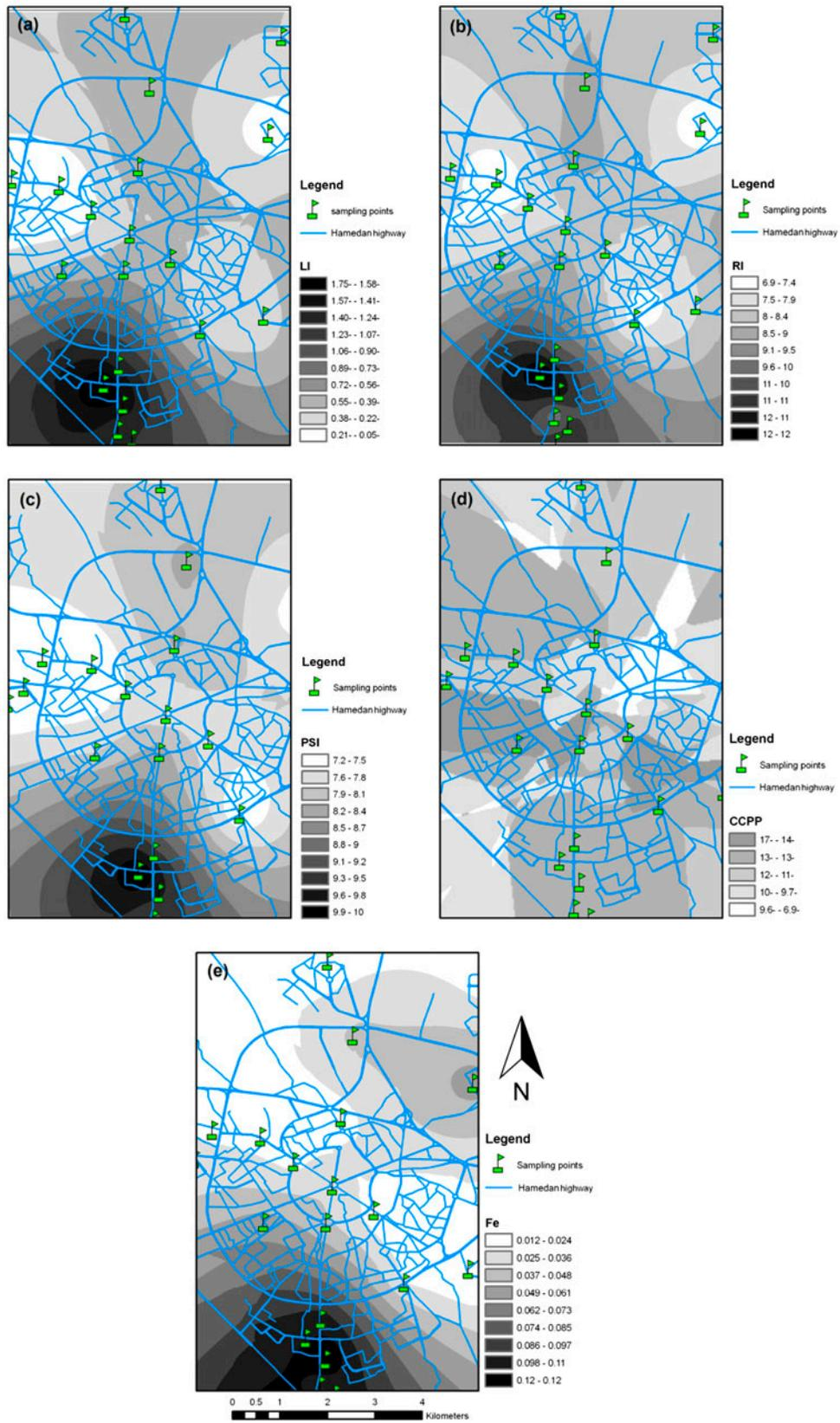
Fig. 4. The prediction maps of corrosion indices (a)–(d) and iron concentration (e) based on the Kriging interpolation model.
