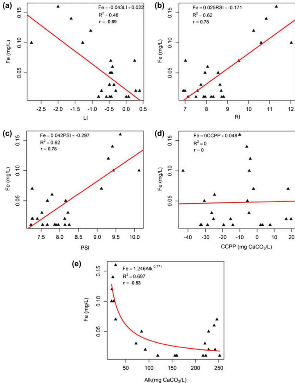
Fig. 3. Scatter plots of corrosion indices (a)–(d) and alkalinity (e) on iron concentration.
