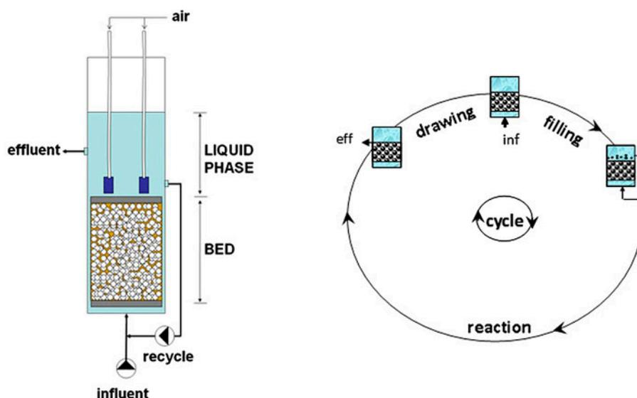
Fig. 1. Sketch (on the left) and operation (on the right) of lab-scale SBBGR.
