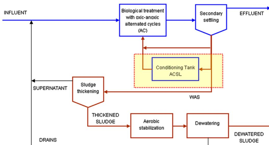
Fig. 2. Sketch of the WWTP upgraded with AC and ACSL.
