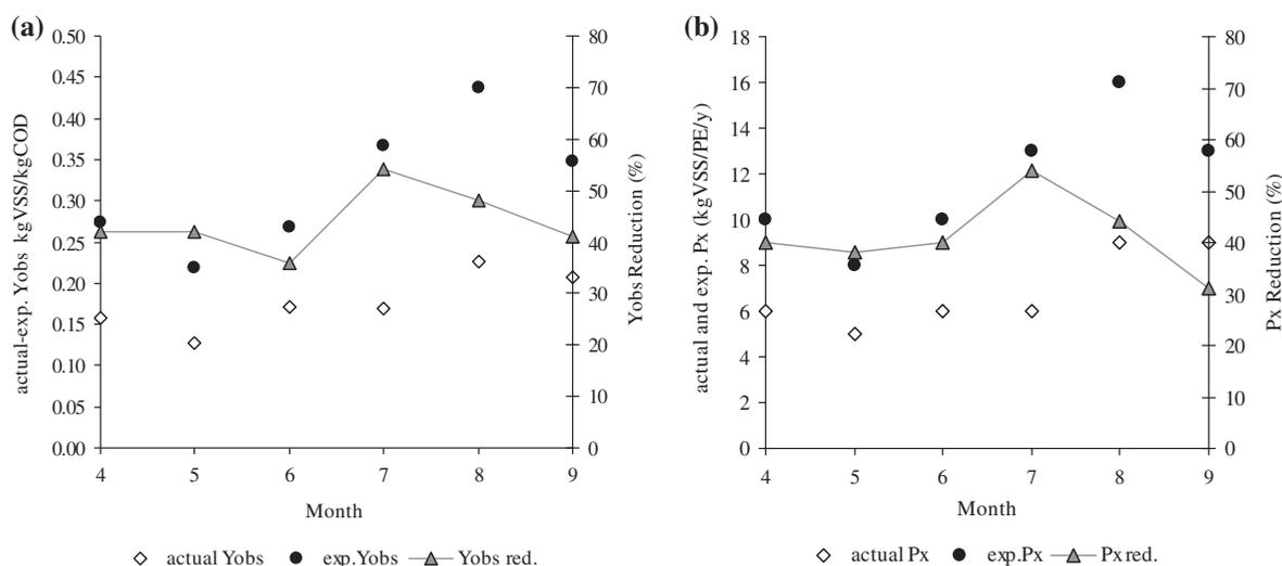
Fig. 5. Actual and expected  $Y_{obs}$  and  $P_x$  values for each experimental month for the ACSL process (a) actual and expected  $Y_{obs}$  and relative reduction percentage; (b) actual and expected  $P_x$  and relative reduction percentage.
