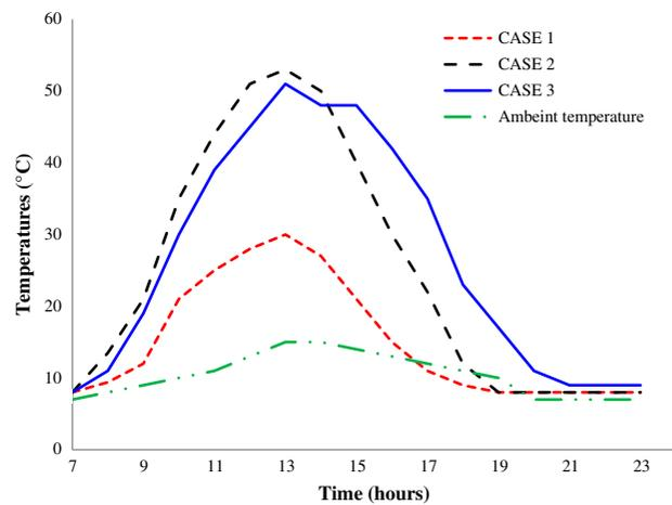
Fig. 4. Water temperatures in the conical distiller for the studied cases.
