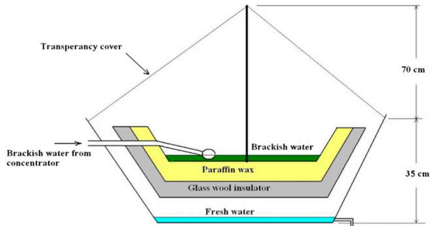
Fig. 1. A schematic diagram for the conical distiller.
