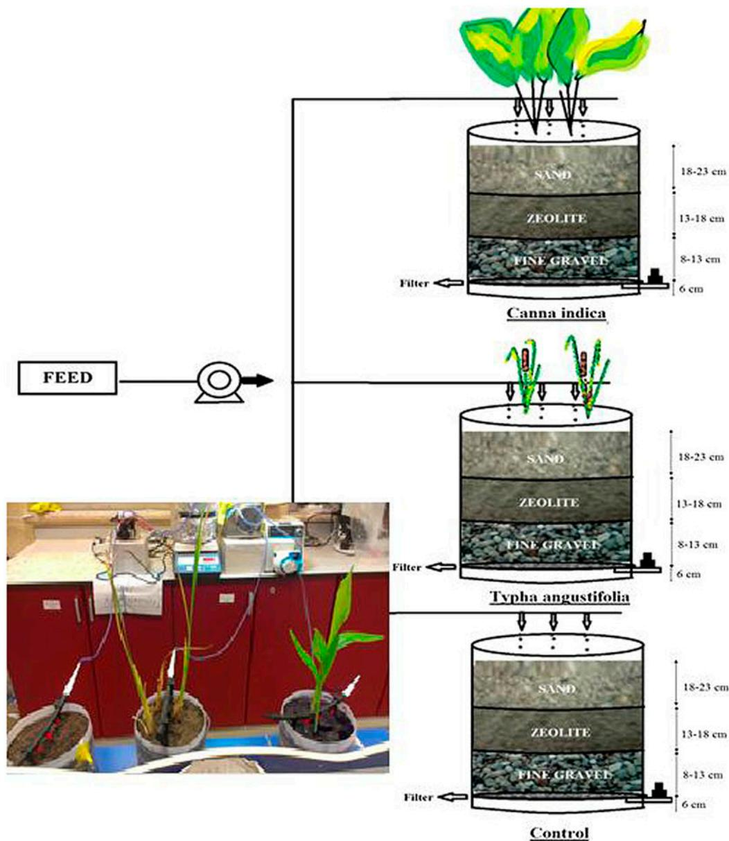
Fig. 2. Reactors were used in experimental studies.
