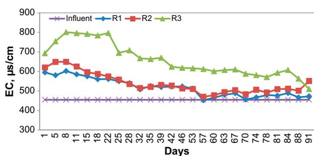
Fig. 7. EC change of the constructed wetland systems (R1: Control, R2: *C. indica*, R3: *T. angustifolia*).
