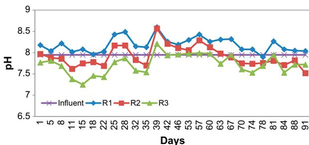
Fig. 5. pH change of the constructed wetland systems (R1: Control, R2: *C. indica*, R3: *T. angustifolia*).
