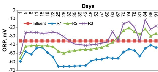
Fig. 6. ORP change of the constructed wetland systems (R1: Control, R2: *C. indica*, R3: *T. angustifolia*).
