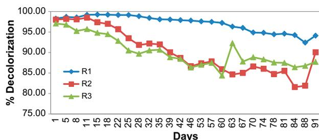
Fig. 8. Decolorization (%) of the constructed wetland systems (R1: Control, R2: *C. indica*, R3: *T. angustifolia*).
