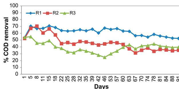
Fig. 3. The COD removal efficiency (%) of the constructed wetland systems (R1: Control, R2: *C. indica*, R3: *T. angustifolia*).
