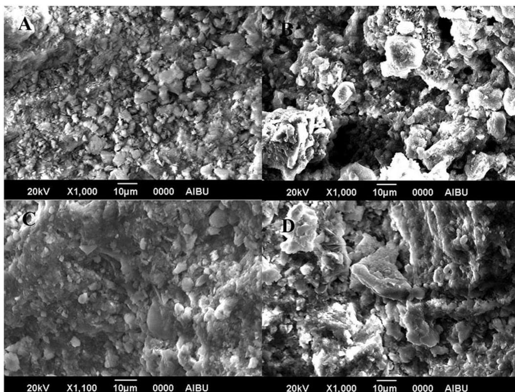
Fig. 9. (A) Scanning electron micrographs of support particle X 1,000, (B) zeolite media of Control Reactor (R1) X 1,000, (C) *C. indica* Reactor (R2) X 1,000 and (D) *T. angustifolia* Reactor (R3) X 1,000.
