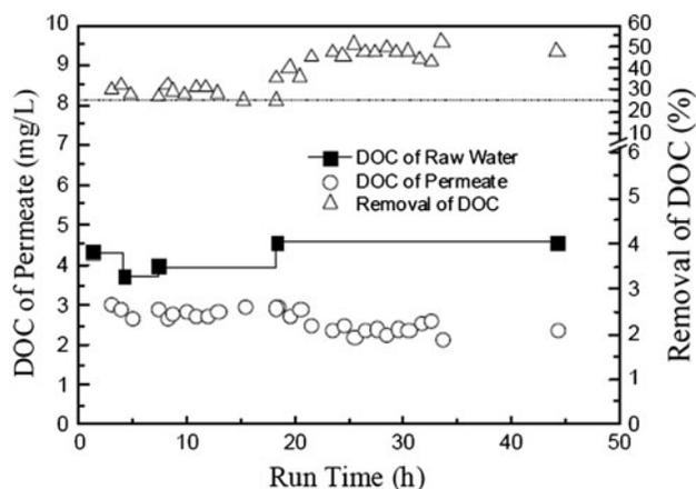
Fig. 7. Removal of DOC by the MCR with a continuous air sparging process. The TMP was 0.025 MPa. The air flow was 1.0 m<sup>3</sup>/h at 20°C. The spiral pump sucking permeate out from membranes ran for 7 min and then stopped for 3 min. The PACl dosage was 90 mg/L, with a corresponding zeta potential of around 0 mV.
