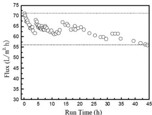
Fig. 4. Membrane flux at a constant TMP of 0.025 MPa with a continual air sparging process. The air flow was  $1.0 \text{ m}^3/\text{h}$  at  $20^\circ\text{C}$ . The spiral pump sucking permeate out from membranes ran for 7 min and then stopped for 3 min. The PACl dosage was  $90 \text{ mg/L}$ , with a corresponding zeta potential of around  $0 \text{ mV}$ .
