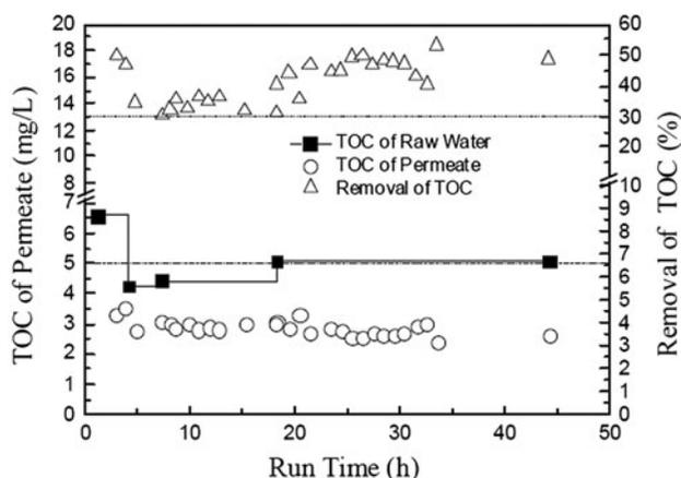
Fig. 6. Removal of TOC by the MCR with a continuous air sparging process. The TMP was  $0.025 \text{ MPa}$ . The air flow was  $1.0 \text{ m}^3/\text{h}$  at  $20^\circ\text{C}$ . The spiral pump sucking permeate out from membranes ran for 7 min and then stopped for 3 min. The PACl dosage was  $90 \text{ mg/L}$ , with a corresponding zeta potential of around  $0 \text{ mV}$ .
