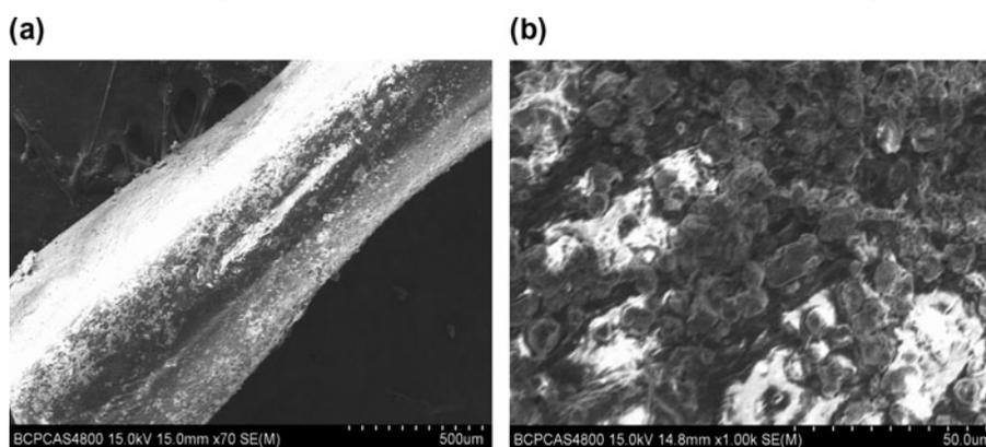
Fig. 9. SEM images of membrane surface after online cleaning by air sparging. TMP = 0.02 MPa. (a) 70 times magnification of membrane surface and (b) 1000 times magnification of cake layer.
