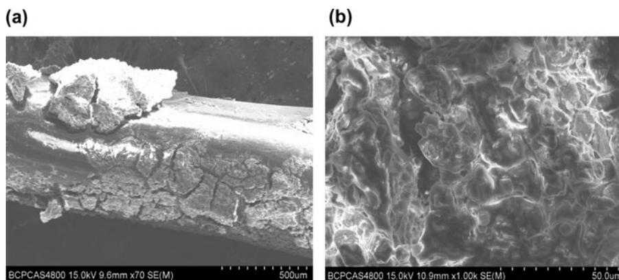
Fig. 8. Fouled membrane surface images obtained by a SEM after 45 h of running for the MCR. The TMP was 0.025 MPa. The air sparging process was continuous at the air flow of 1.0 m<sup>3</sup>/h (20°C). The spiral pump sucking permeate out from membranes ran for 7 min and then stopped for 3 min. The PACl dosage was 90 mg/L, with a corresponding zeta potential of around 0 mV. (a) 70 times magnification of membrane surface and (b) 1000 times magnification of cake layer.
