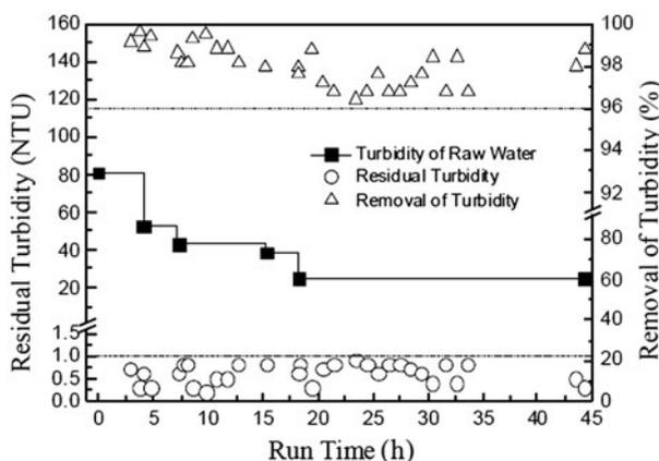
Fig. 5. Removal of turbidity by the MCR with a continuous air sparging process. The TMP was  $0.025 \text{ MPa}$ . The air flow was  $1.0 \text{ m}^3/\text{h}$  at  $20^\circ\text{C}$ . The spiral pump sucking permeate out from membranes ran for 7 min and then stopped for 3 min. The PACl dosage was  $90 \text{ mg/L}$ , with a corresponding zeta potential of around  $0 \text{ mV}$ .
