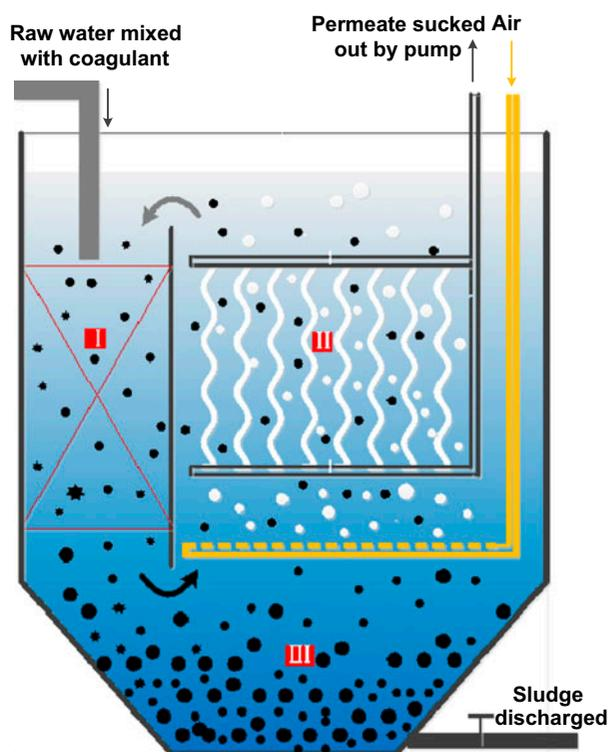
Fig. 1. Principle diagram of the submerged MCR.
