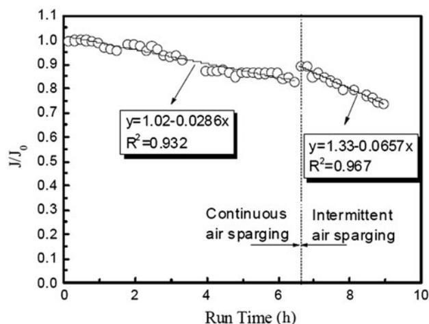
Fig. 3. Effect of air sparging condition on membrane flux. The TMP was 0.025 MPa. The air flow was 1.0 m<sup>3</sup>/h at 20°C. The intermittent air sparging was to aerate for 7 min and then stop for 3 min. The spiral pump sucking permeate out from membranes ran for 7 min and then stopped for 3 min. The PACl dosage was 90 mg/L, with a corresponding zeta potential of around 0 mV.
