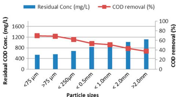
Fig. 3. COD removal at different particle sizes (dosage: 15 g, contact time: 60 min, agitation speed: 150 rpm, and pH 2).
