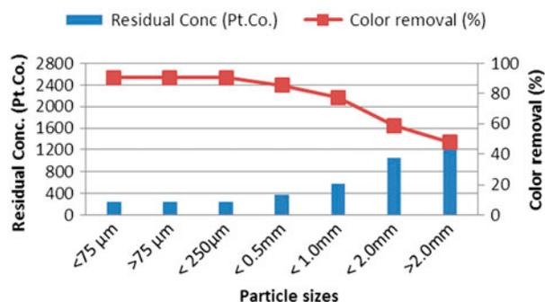
Fig. 1. Color removal at different particle sizes (dosage: 15 g, contact time: 60 min, agitation speed: 150 rpm, and pH 2).
