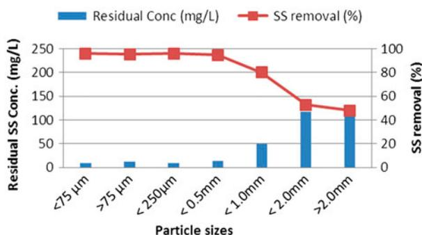
Fig. 2. Suspended solid removal at different particle sizes (dosage: 15 g, contact time: 60 min, agitation speed: 150 rpm, and pH 2).
