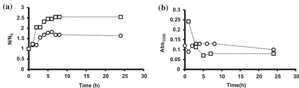
Fig. 2. Growth of *P. putida* (DSM4478) (a) and COD removal (b) in a medium with 100 ppm of *p*-hydroxybenzoic acid without (circles) or with addition (squares) of 25 ppm of phenol in all cases:  $N_0$ :  $2.5 \times 10^{-2}$  g/L;  $T = 28^\circ\text{C}$ ; and 200 rpm.
