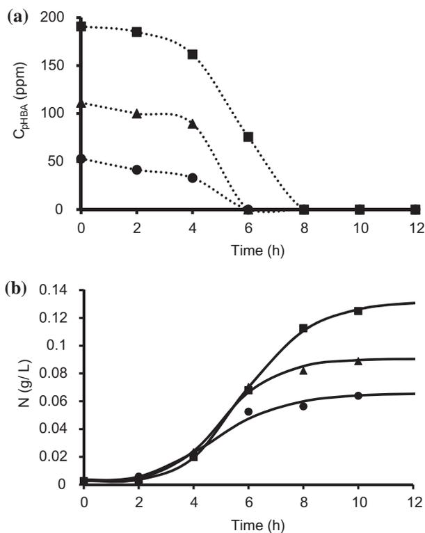
Fig. 4. Evolution of the *p*-hydroxybenzoic acid concentration (a) and growth of *P. putida* (DSM4478) (b) in shake flasks under different *p*-hydroxybenzoic acid concentrations: 50 ppm (●), 100 ppm (▲) and 200 ppm (■). In all cases:  $N_0$ :  $2.5 \times 10^{-2}$  g/L;  $T$ : 28°C; and 200 rpm.
