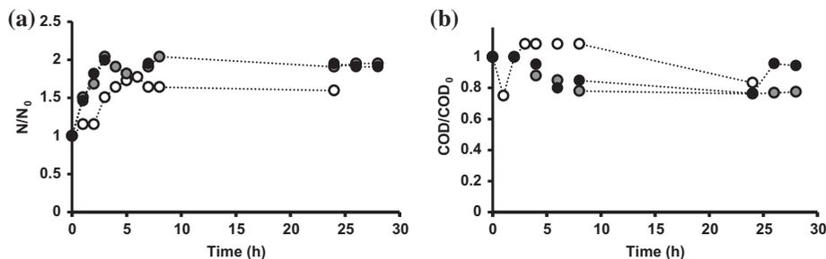
Fig. 1. Growth of *P. putida* (DSM4478) (a) and COD removal (b) in shake flasks without acclimation and under different *p*-hydroxybenzoic acid concentrations: 100 ppm (hollow symbols), 200 ppm (gray symbols), and 300 ppm (black symbols). In all cases:  $N_0$ :  $2.5 \times 10^{-2}$  g/L;  $T = 28^\circ\text{C}$ ; and 200 rpm.
