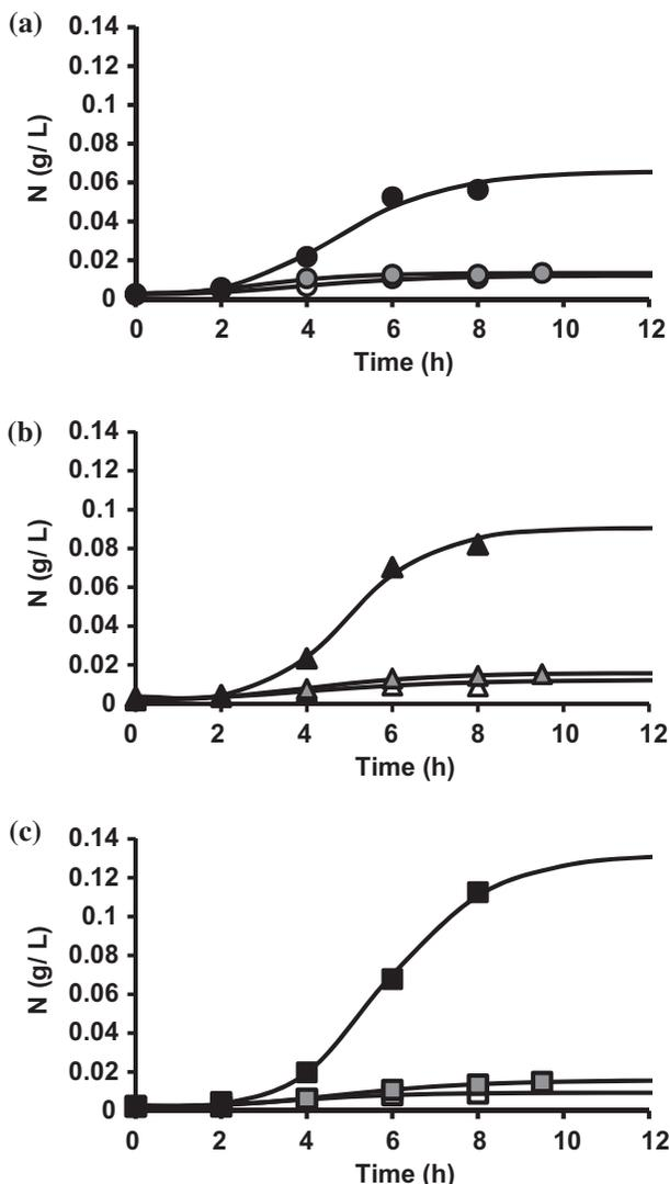
Fig. 5. Growth of *P. putida* (DSM4478) in shake flasks under different agitation speeds: 50 rpm (hollow symbols), 100 rpm (gray symbols) and 200 rpm (black symbols) for the next initial concentrations of *p*-hydroxybenzoic acid: (a) 50 ppm (circles), (b) 100 ppm (triangles), and (c) 200 ppm (squares). In all cases:  $N_0$ :  $2.5 \times 10^{-3}$  g/L;  $T = 28^\circ\text{C}$ .
