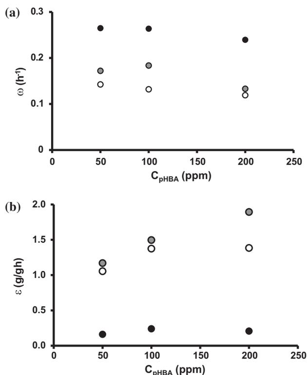
Fig. 7. Effect of the initial concentration of *p*-hydroxybenzoic acid on the  $\omega$  and  $\varepsilon$  values under different agitation speeds: 50 rpm (hollow symbols), 100 rpm (gray symbols), and 200 rpm (black symbols). In all cases:  $N_0$ :  $2.5 \times 10^{-3}$  g/L;  $T = 28^\circ\text{C}$ .
