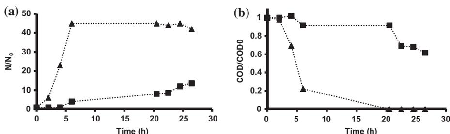
Fig. 3. Growth of *P. putida* (DSM4478) (a) and COD removal (b) in a medium with 100 ppm of *p*-hydroxybenzoic acid after a sequential acclimation (three passes) by means of constant (squares) or progressive concentrations (triangles). In all cases:  $N_0$ :  $2.5 \times 10^{-2}$  g/L;  $T = 28^\circ\text{C}$  and 200 rpm.
