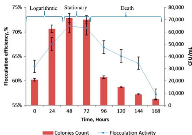
Fig. 2. Time course of *B. Subtilis* growth pattern and flocculation efficiency.
