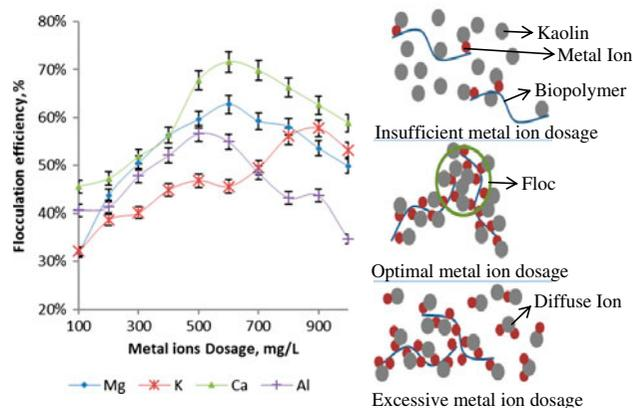
Fig. 4. The effect of multivalent metal ions dosage on flocculation efficiency.
