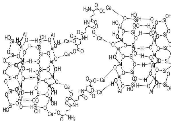
Fig. 6. The structure of the final product of calcium-hybridized biopolymer with kaolin clay suspension.
