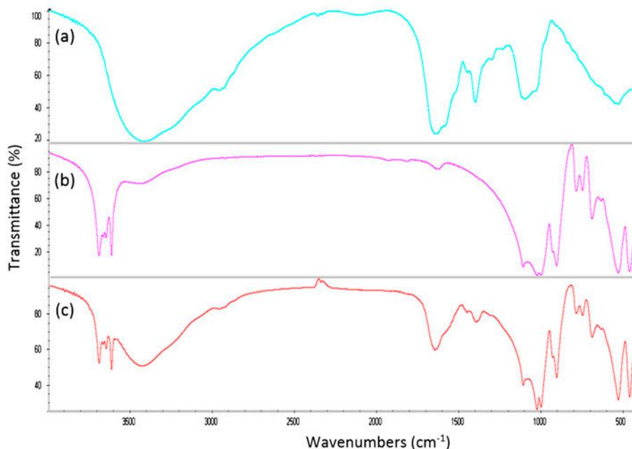
Fig. 5. The infrared spectrum of (a) purified biopolymer hybrid with  $\text{Ca}^{2+}$ , (b) kaolin clay suspension, and (c) sludge of kaolin clay suspension treated by hybridized biopolymer.
