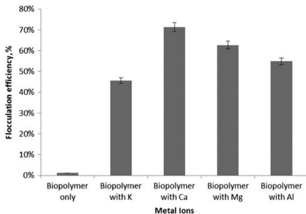
Fig. 3. The effect of biopolymer with and without metal ions hybridization on the flocculating activity (Metal ion concentration was constant at 600 mg/L and the optimal incubation period was 48 h).
