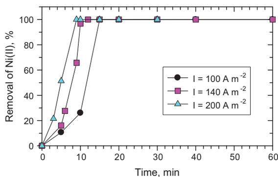
Fig. 4. Removal of Ni(II) at different applied current density (*I*).
