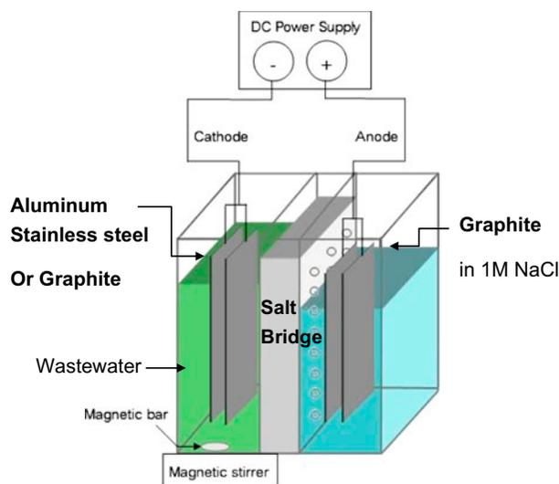
Fig. 1. Diagram of constant-current electrochemical cell.
