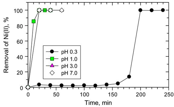
Fig. 3. Removal of Ni(II) at various initial pH using a graphite cathode.
