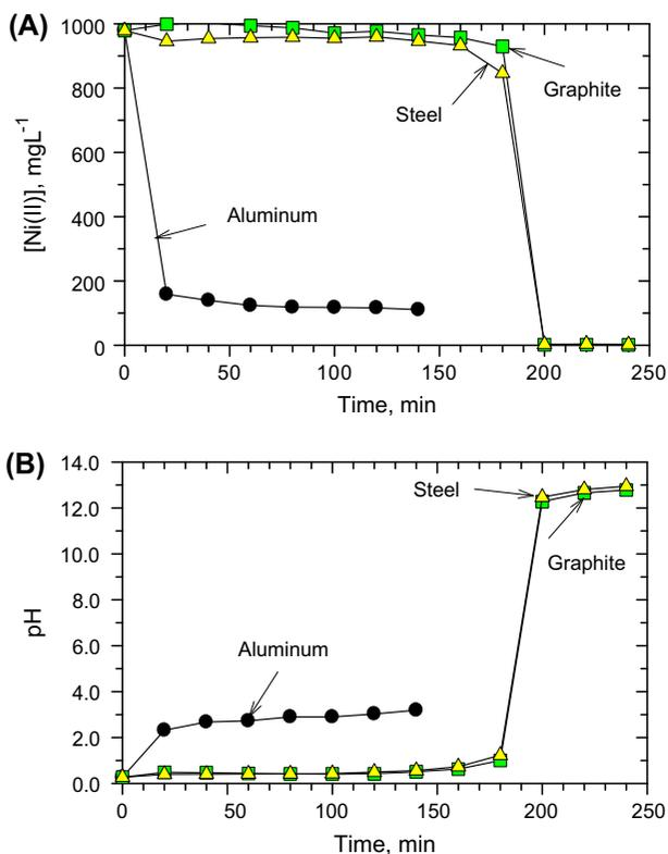
Fig. 2. Electrolysis as a function of time using different cathodes with initial pH 0.3. (A) Decay of concentration of Ni(II) and (B) change in pH.
